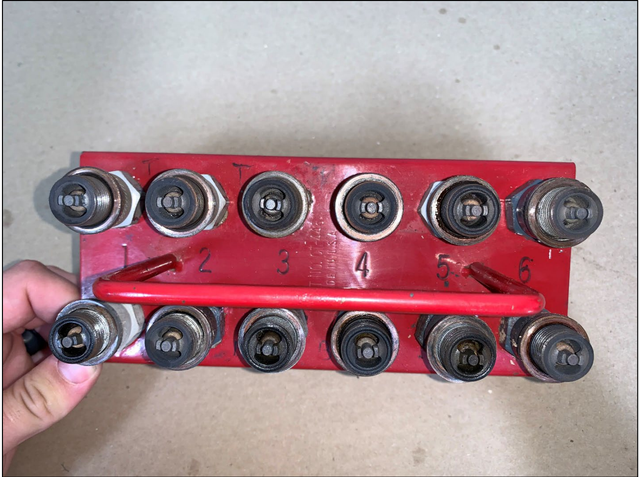
Figure 5: View of the top and bottom spark plugs.
