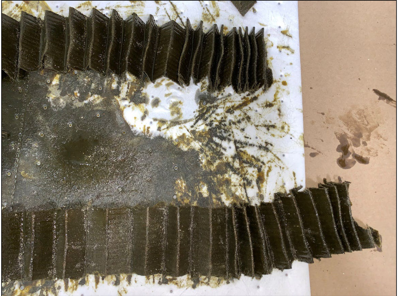
Figure 7: View of the oil filter removed and disassembled.
