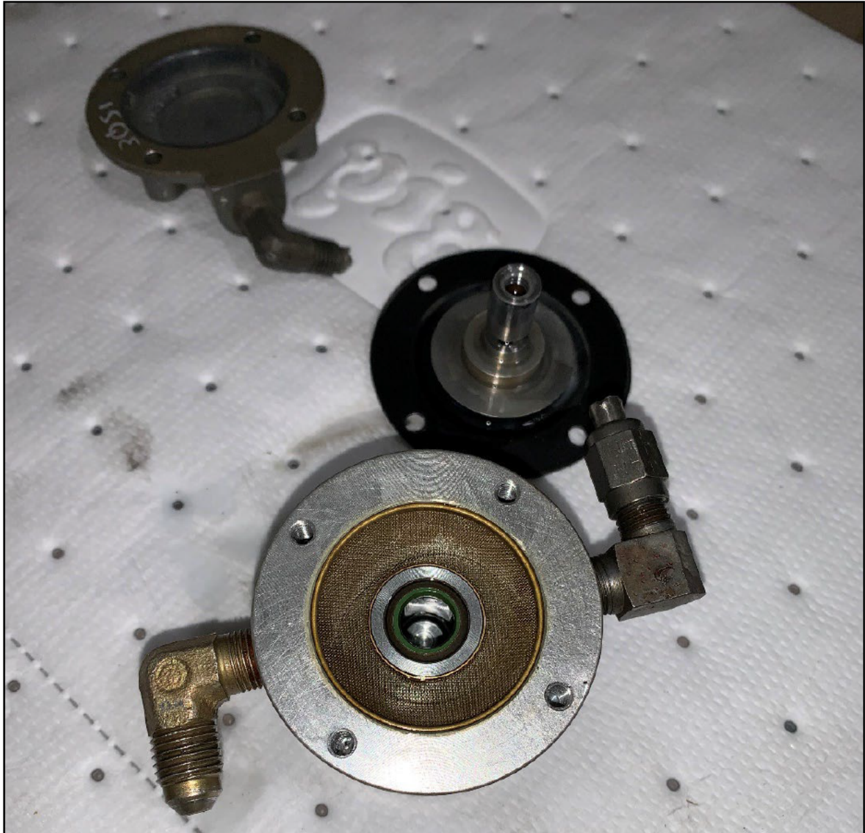
Figure 6: View of the fuel manifold partially disassembled and without contamination.
