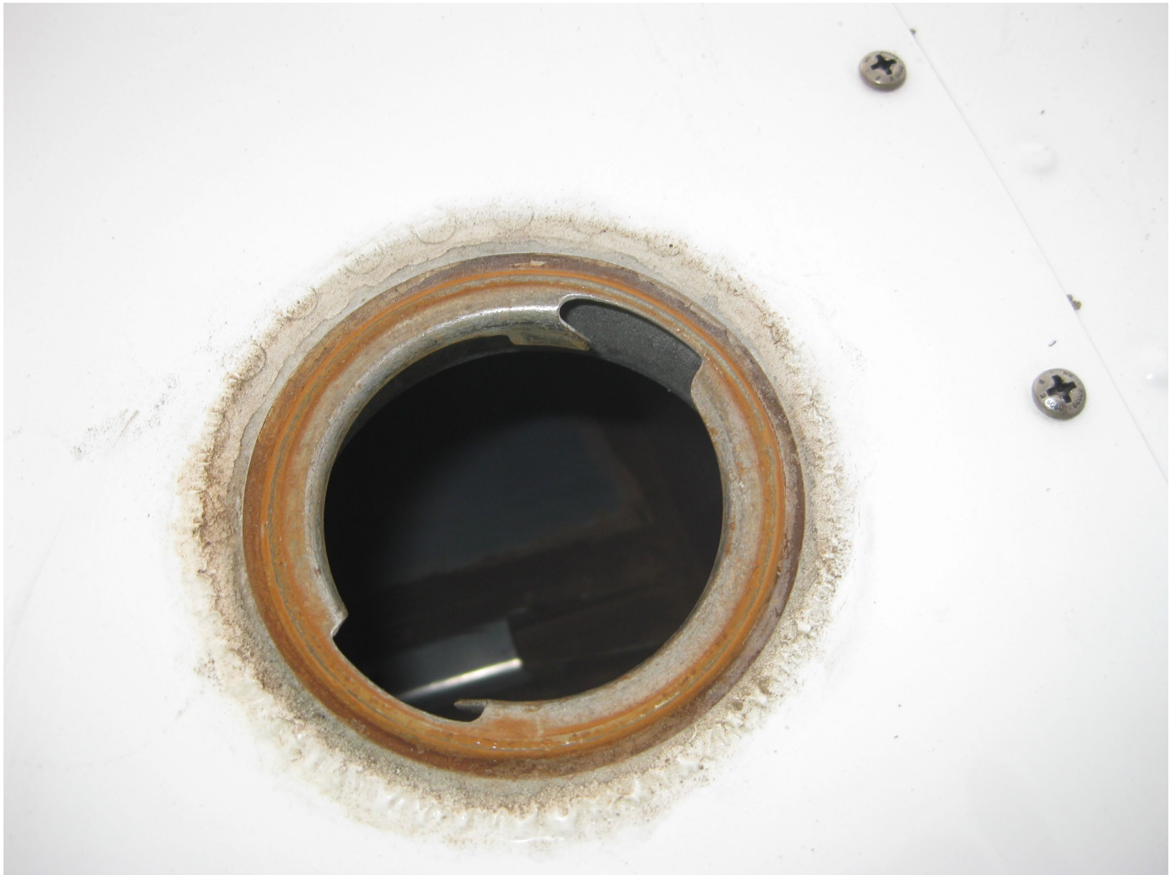
Photo 3 – Left Fuel Tank Filler Port (FAA Photo)
