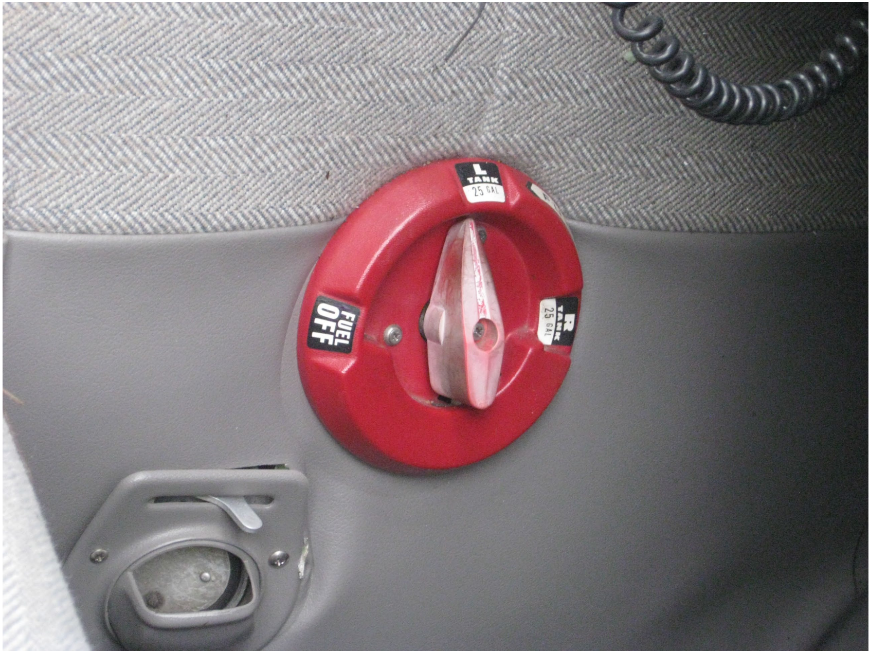
Photo 4 – Cockpit Fuel Tank Selector (FAA Photo)
