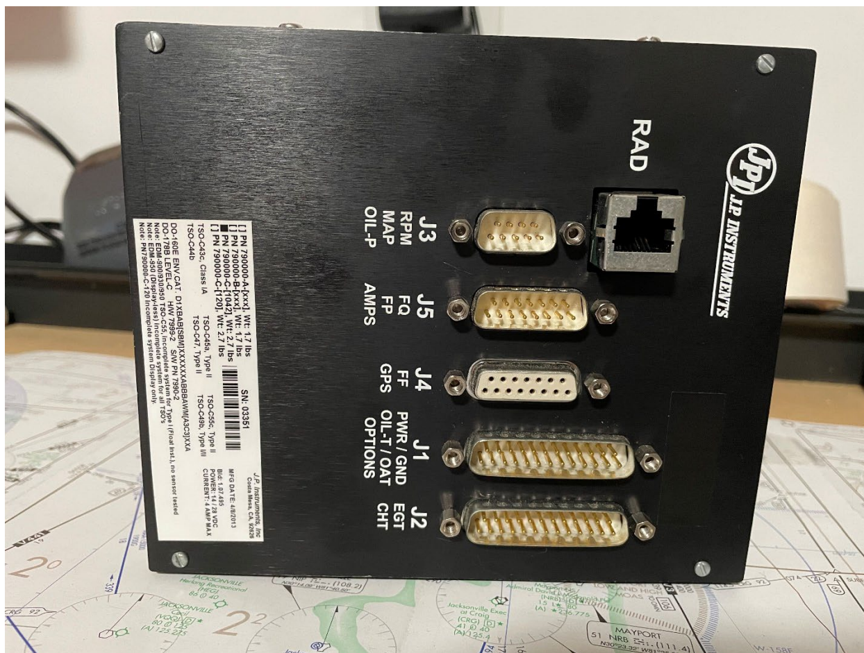
Figure 2. View of Back of JPI
