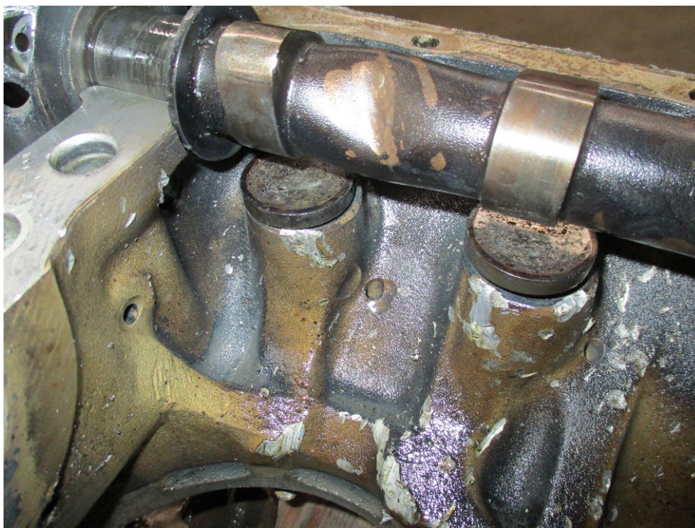
Photograph 1 -Wear to Camshaft Lobes and Lifters (FAA)
