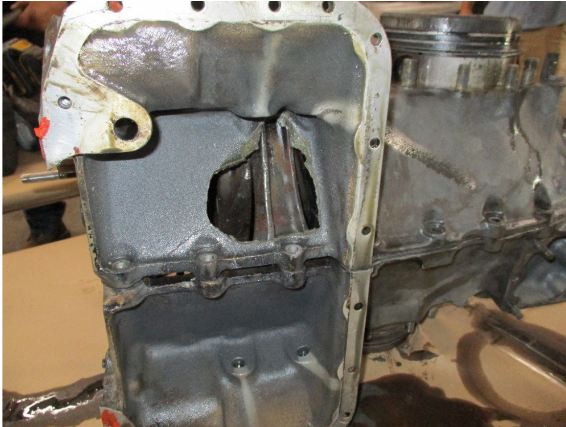
Photograph 6 - Large Hole in the Engine Case (Courtesy of FAA)
