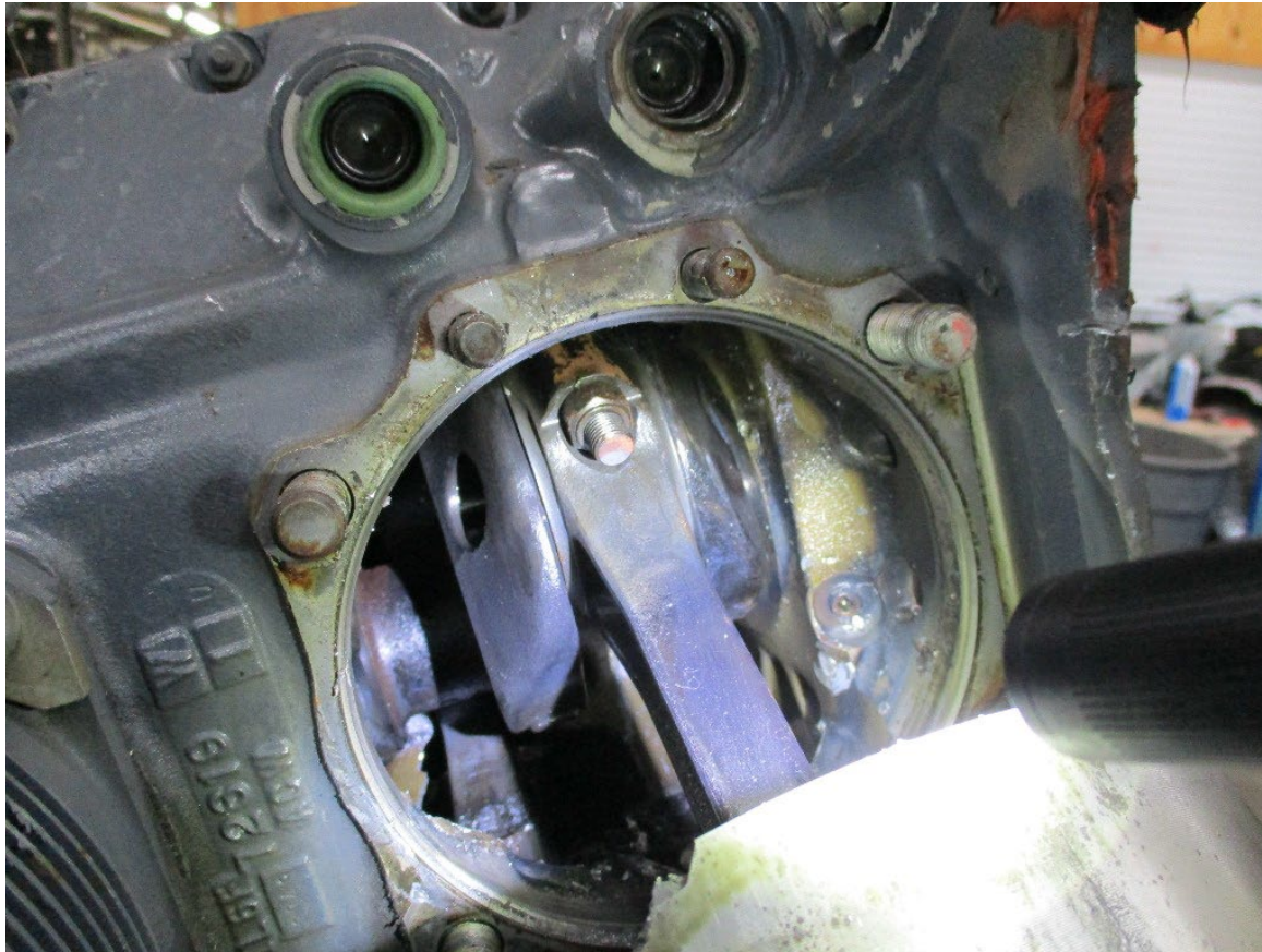
Photograph 5 - Damage to the No. 4 cylinder/piston (Courtesy of FAA)
