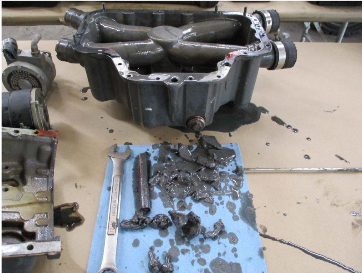
Photograph 7 - Oil Sump Screen and Metallic Debris Found in the Oil Sump (Courtesy of FAA)
