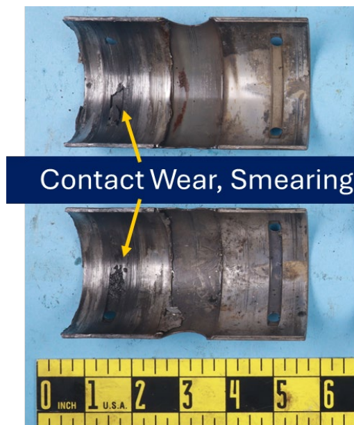
Figure 4. Wear on the forward main journal bearing.
