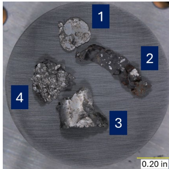
Figure 9. Particles from the oil filter subjected to EDS analysis. EDS Spectra for each particle can be seen in the following figures.
