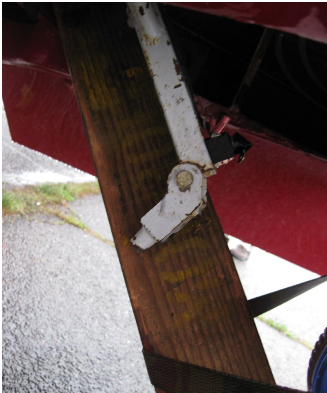
Photo 4 – View of Broken Left Landing Gear Lock. Wood For Support Post-Accident (Courtesy of FAA)
