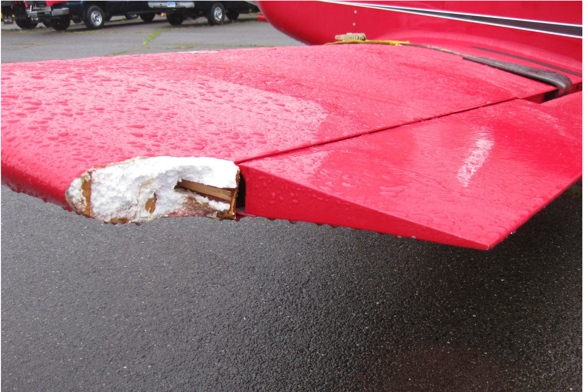
Photo 2 – Closeup View of Damaged Left Wingtip (Courtesy of FAA)
