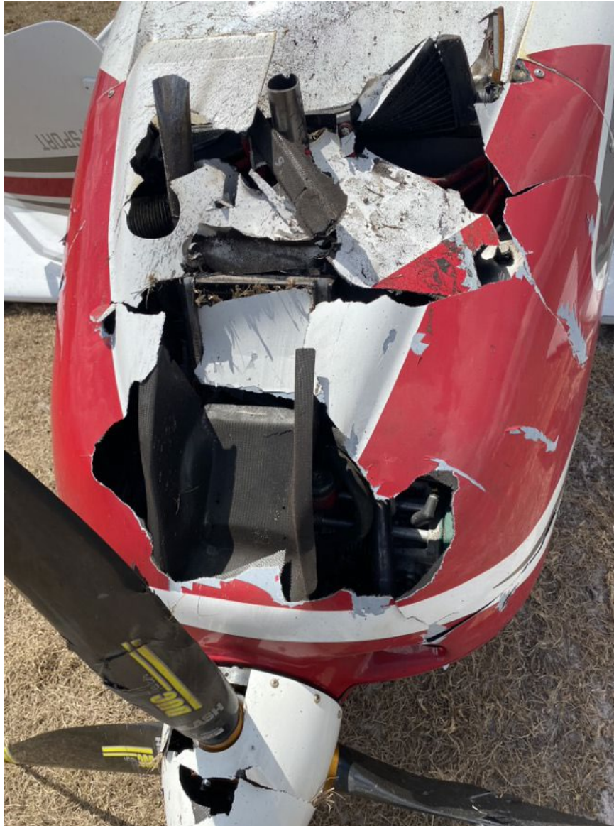
Photograph 7 - Nose Landing Gear Mounting Location (Courtesy of FAA)
