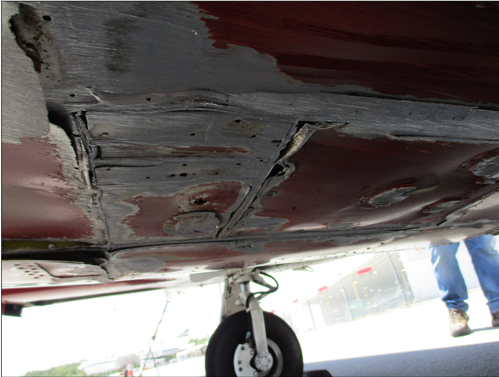
Photos 3: Additional overview of the substantial damage sustained to the fuselage (Photo Courtesy of FAA)
