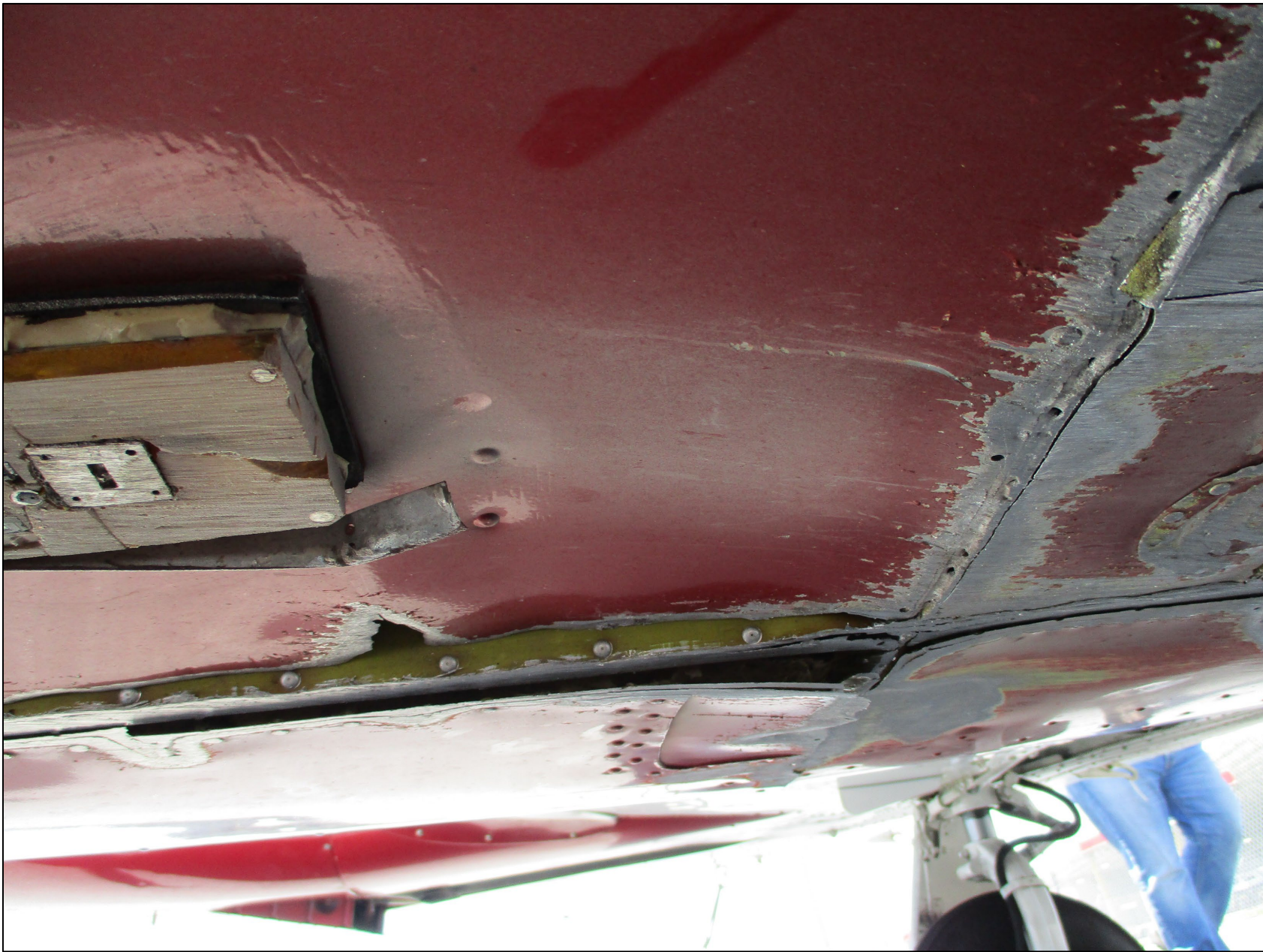
Photos 2: Overview of the substantial damage sustained to the fuselage (Photo Courtesy of FAA)
