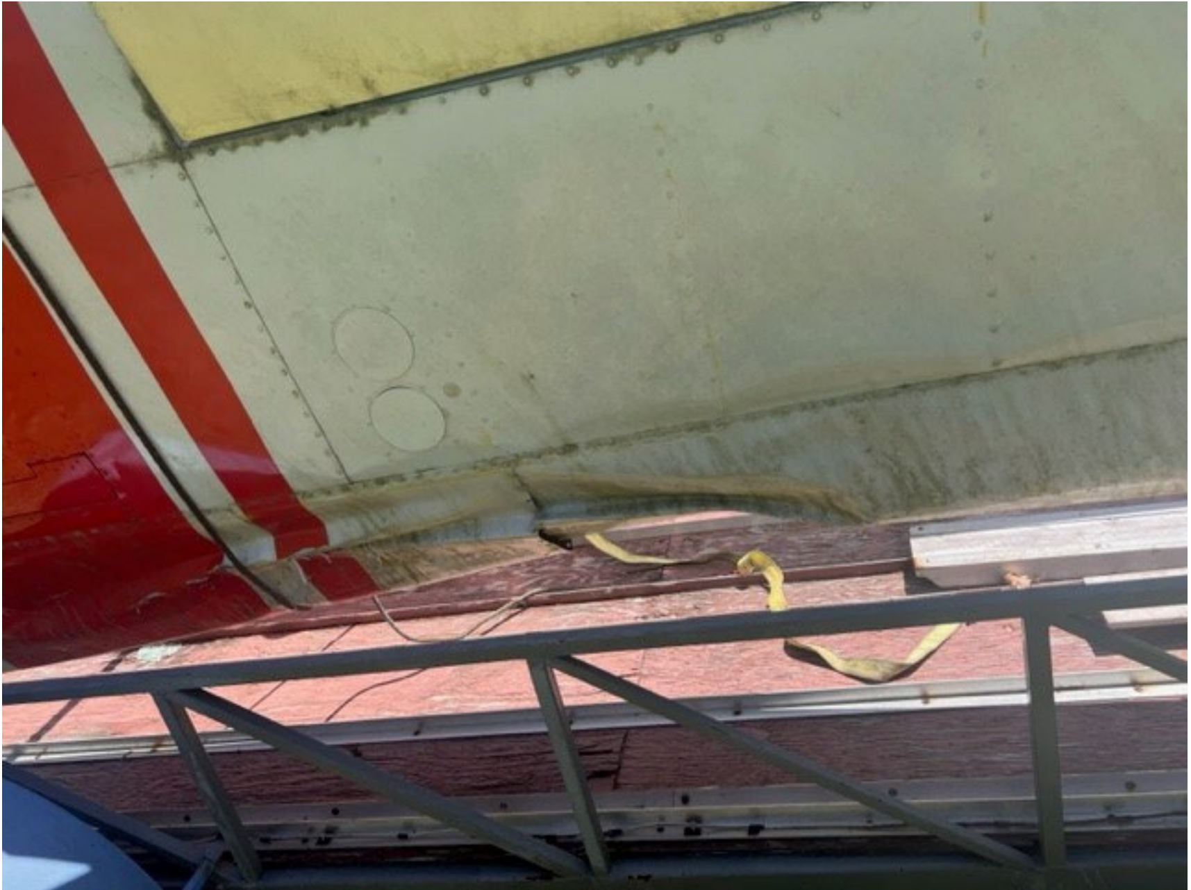
Photo 2 – wing, leading edge damage (FAA)
