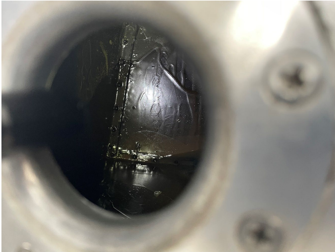
Photograph 3 - Examination of the main fuel tank showing no fuel (Courtesy of FAA)
