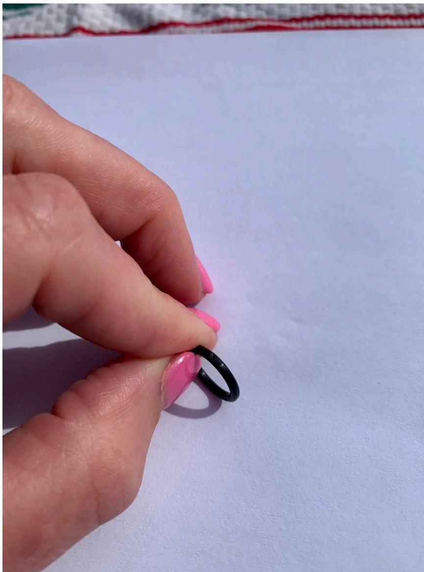
Photograph 1 - Larger tear on check valve O-ring
