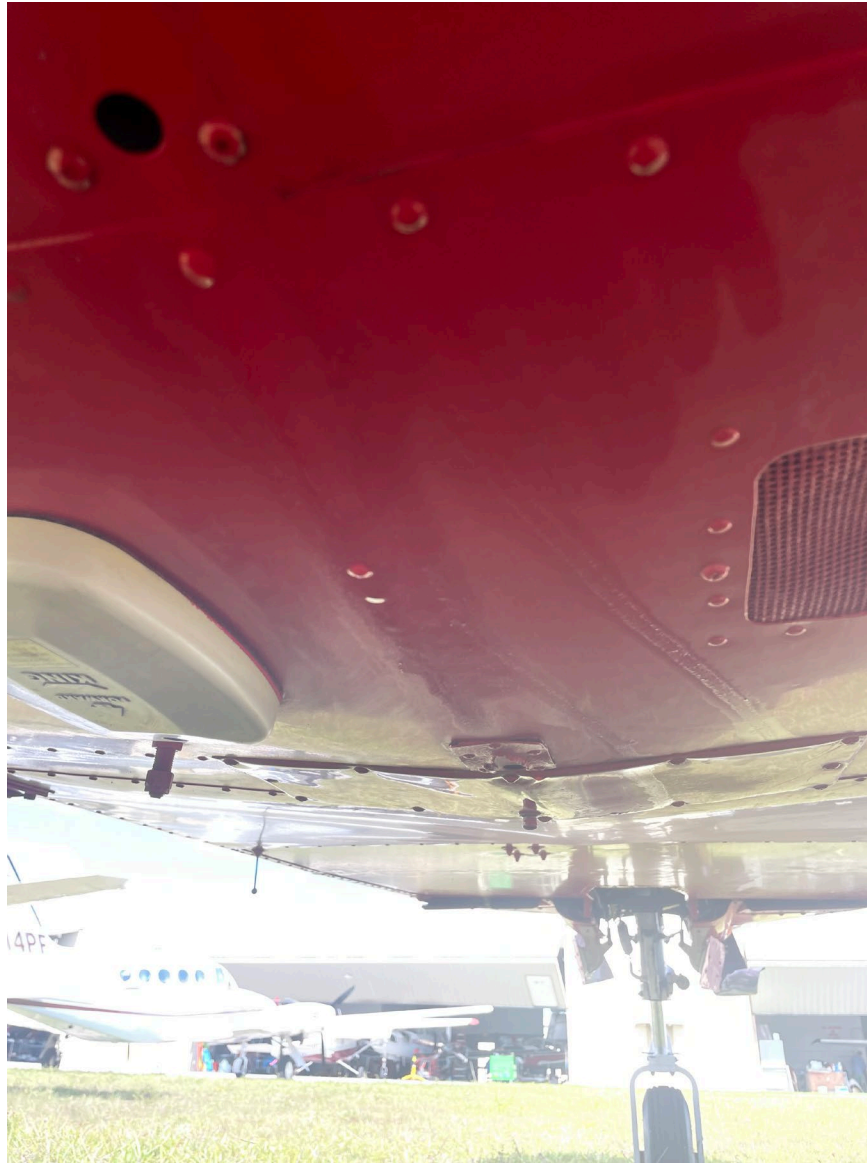
Photograph 4 - Under Belly of Airplane and Hydraulic Fluid (Courtesy of FAA)
