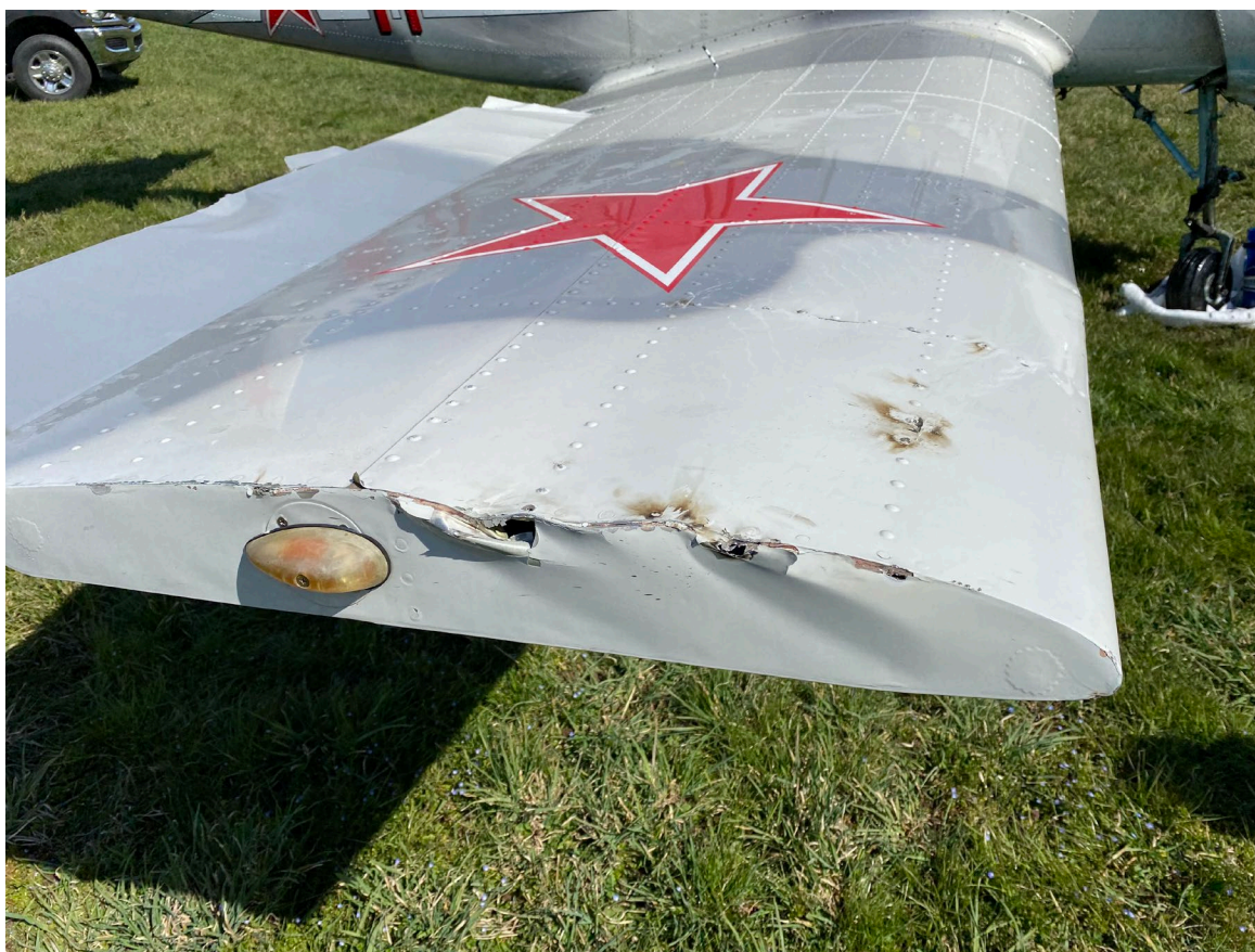
Photograph 1 - View of damage to the right wingtip (Courtesy of FAA)
