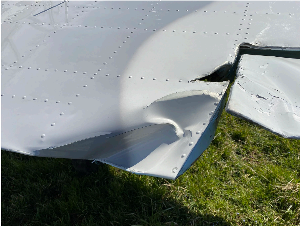
Photograph 3 - View of right wing rib and aileron damage. (Courtesy of FAA)
