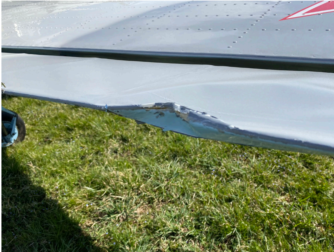
Photograph 2 - View of aileron trailing edge damage. (Courtesy of FAA)
