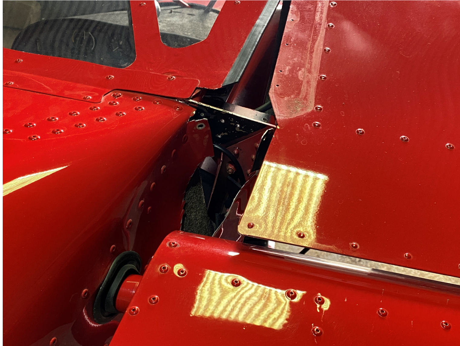
Photo 3: View of the damage to the right wing and fuselage (Photo Courtesy of FAA)
