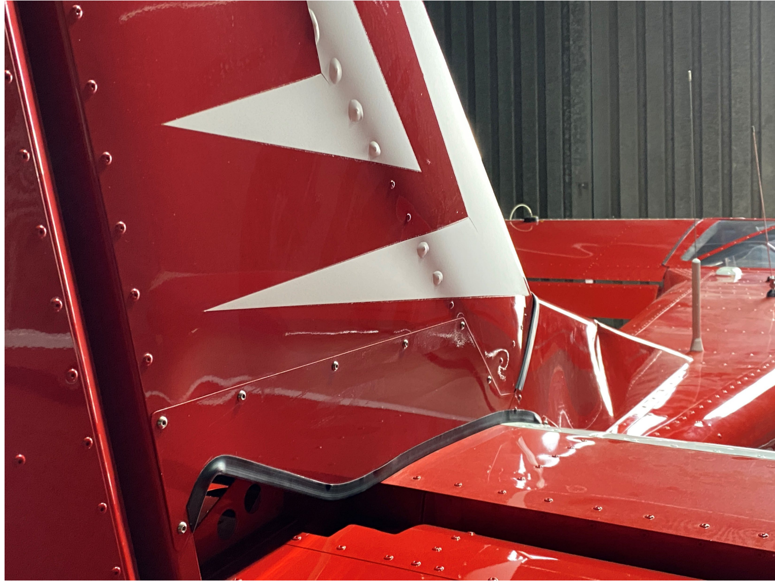
Photo 3: View of damage to the vertical stabilizer (Photo Courtesy of FAA)
