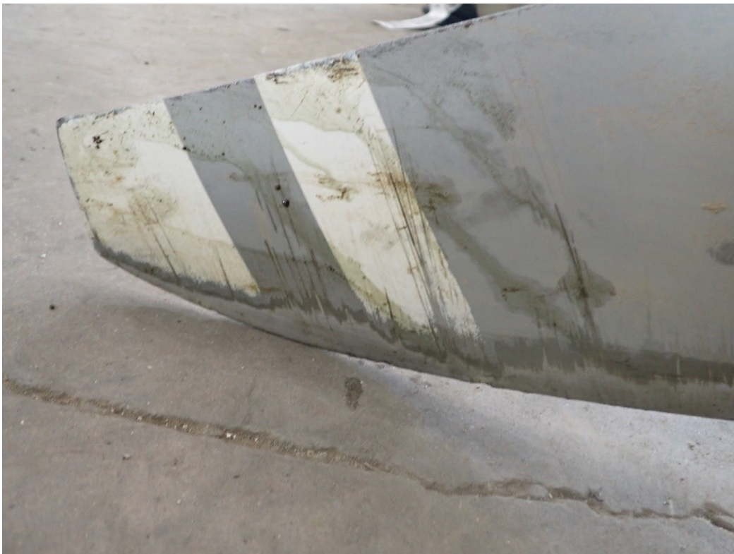
Photo 63: Blade B leading edge polishing, gouging and chordwise scratching.
