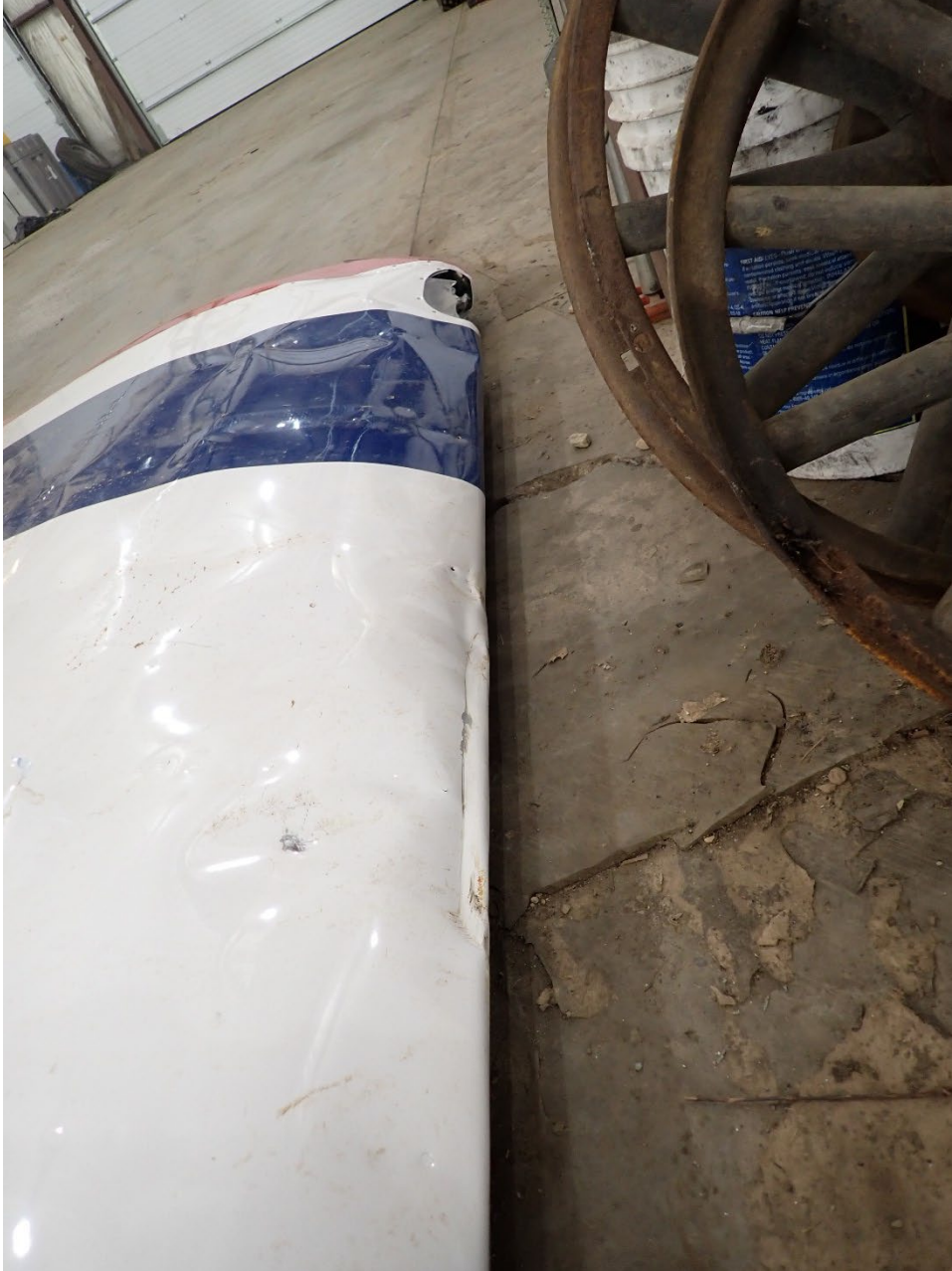
Photo 15: View of the left-wing leading-edge damage.
