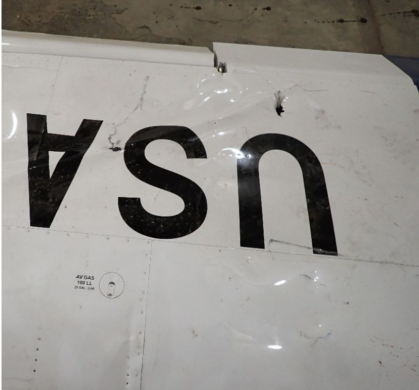
Photo 16: View of the buckling on the top of the left wing.
