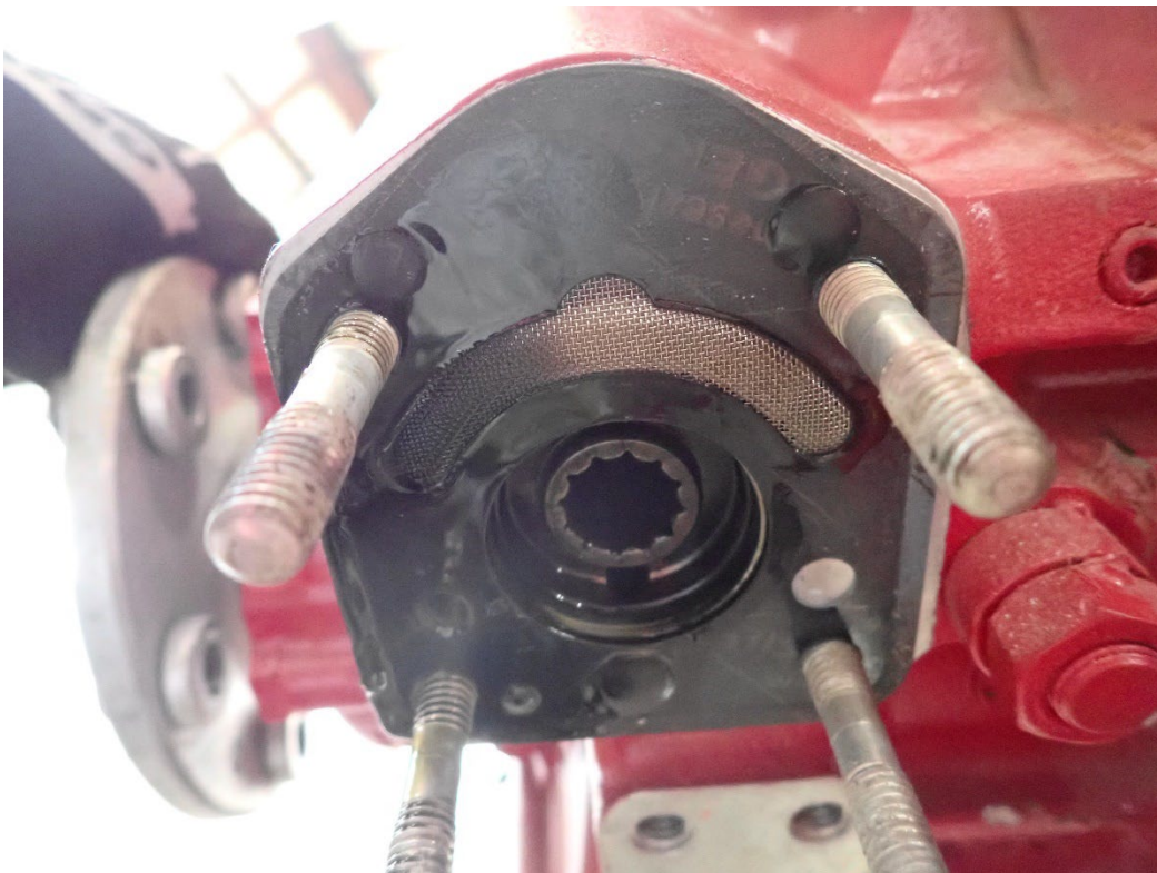
Photo 56: Propeller governor gasket screen free of debris.
