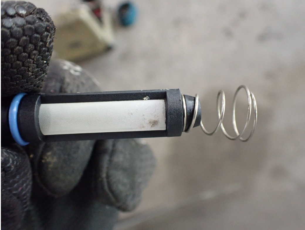
Photo 49: Fuel inlet screen with minor contamination.
