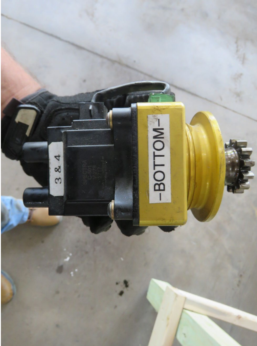
Photo 44: View of the magneto that powered the bottom sparkplugs. (Lycoming Photo)
