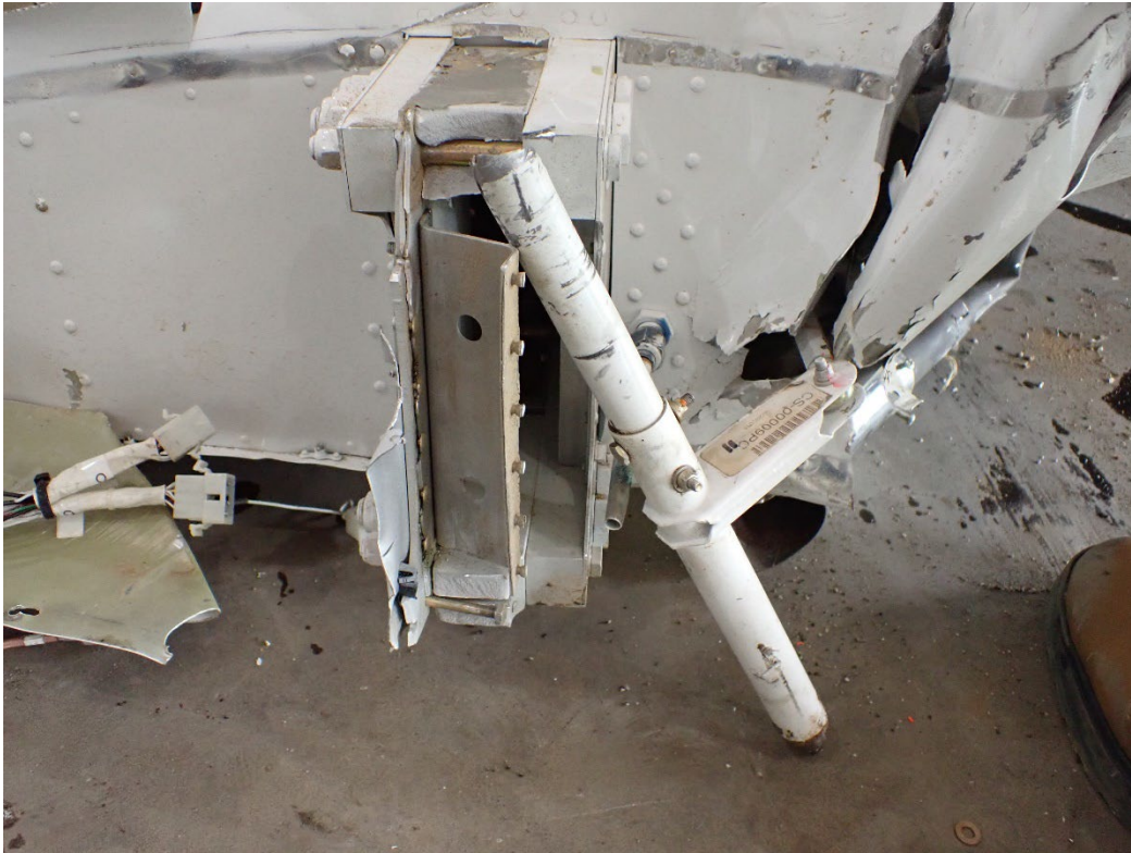
Photo 21: View of the right wing spar that remained attached to the fuselage.
