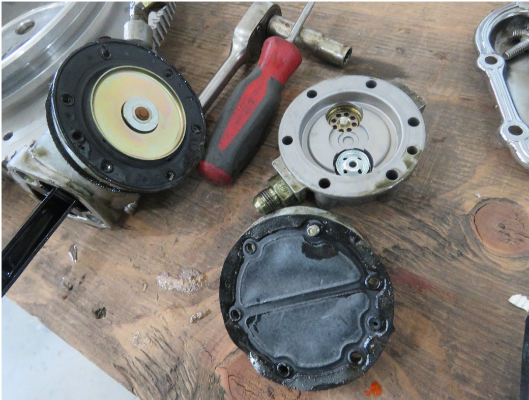
Photo 46: Engine driven fuel pump disassembled for examination. (Lycoming Photo)
