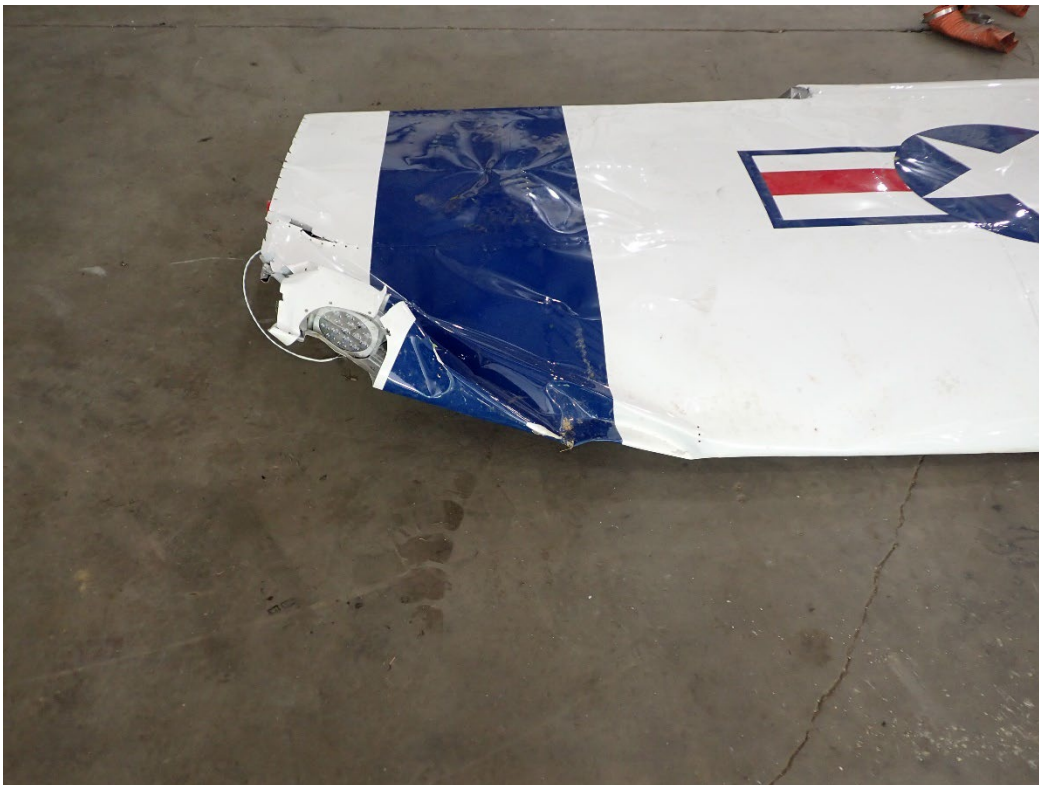
Photo 26: Damage to the right wing outboard leading edge.
