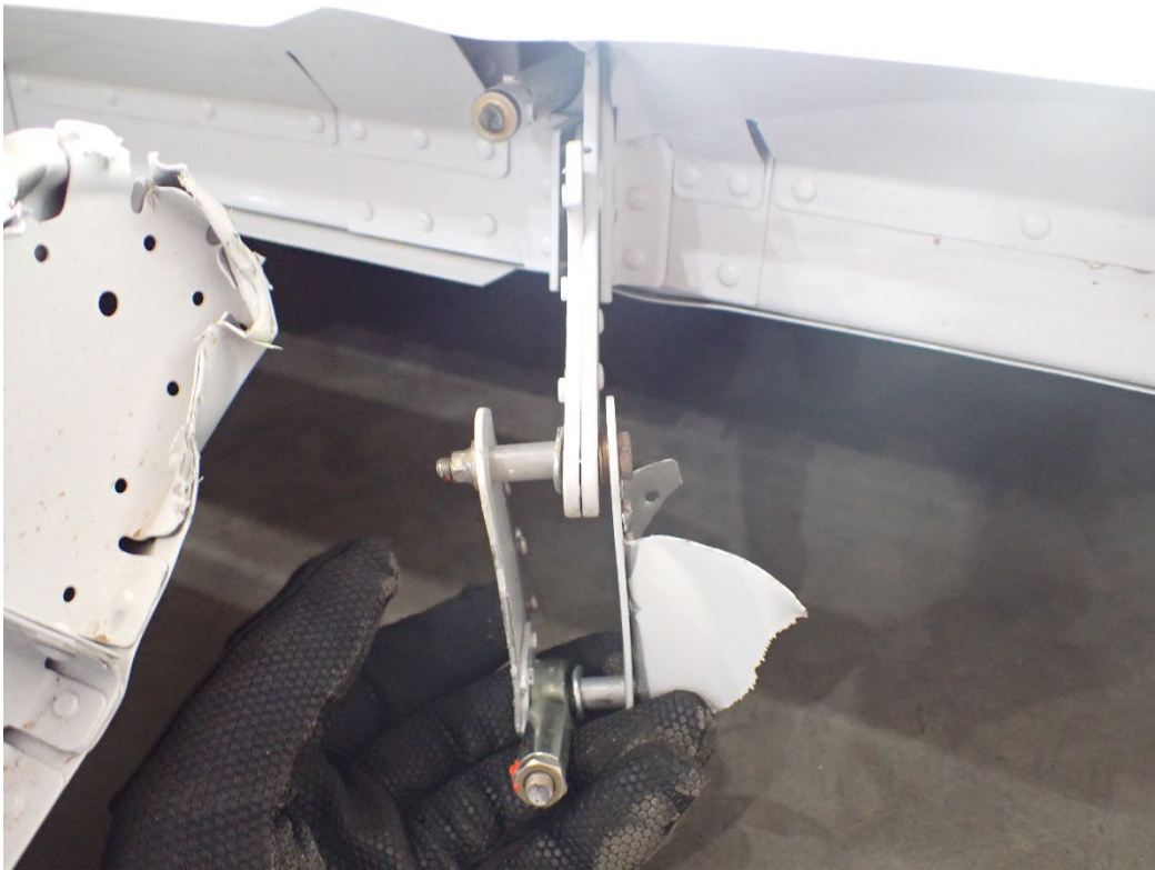
Photo 28: View of impact fractured right aileron pushrod head.
