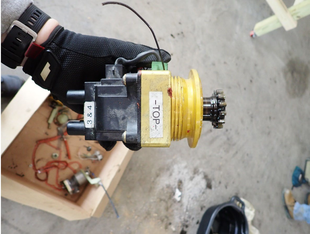
Photo 43: View of the magneto which powered the top sparkplugs.
