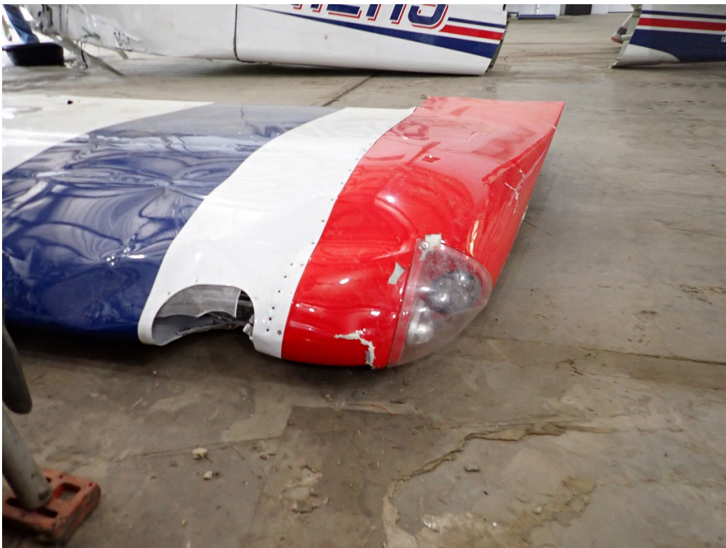
Photo 17: View of the left wing tip damage.
