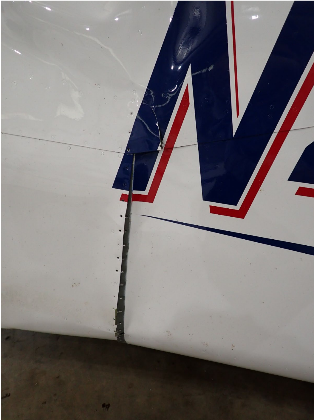
Photo 4: Buckling of the left side of the fuselage.
