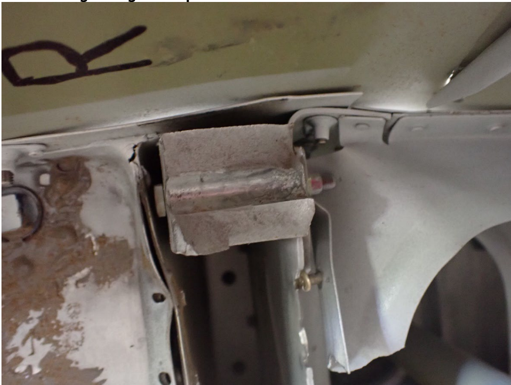
Photo 24: Right wing upper spar fracture.
