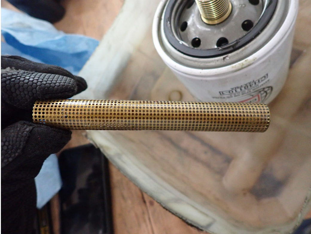
Photo 53: Oil suction screen free of debris.
