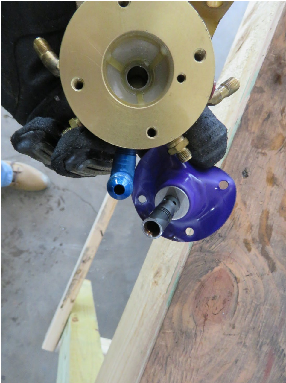
Photo 50: Fuel flow divider removed and disassembled for examination. (Lycoming Photo)
