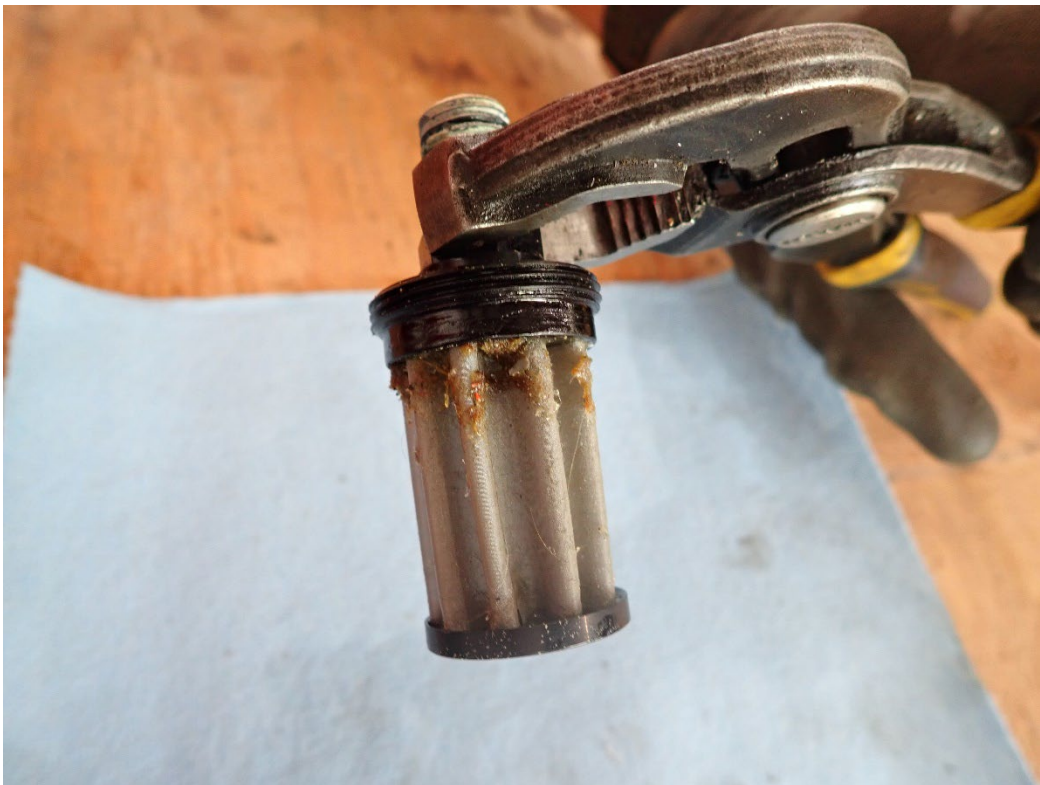
Photo 36: View of debris found in the inline fuel filter.
