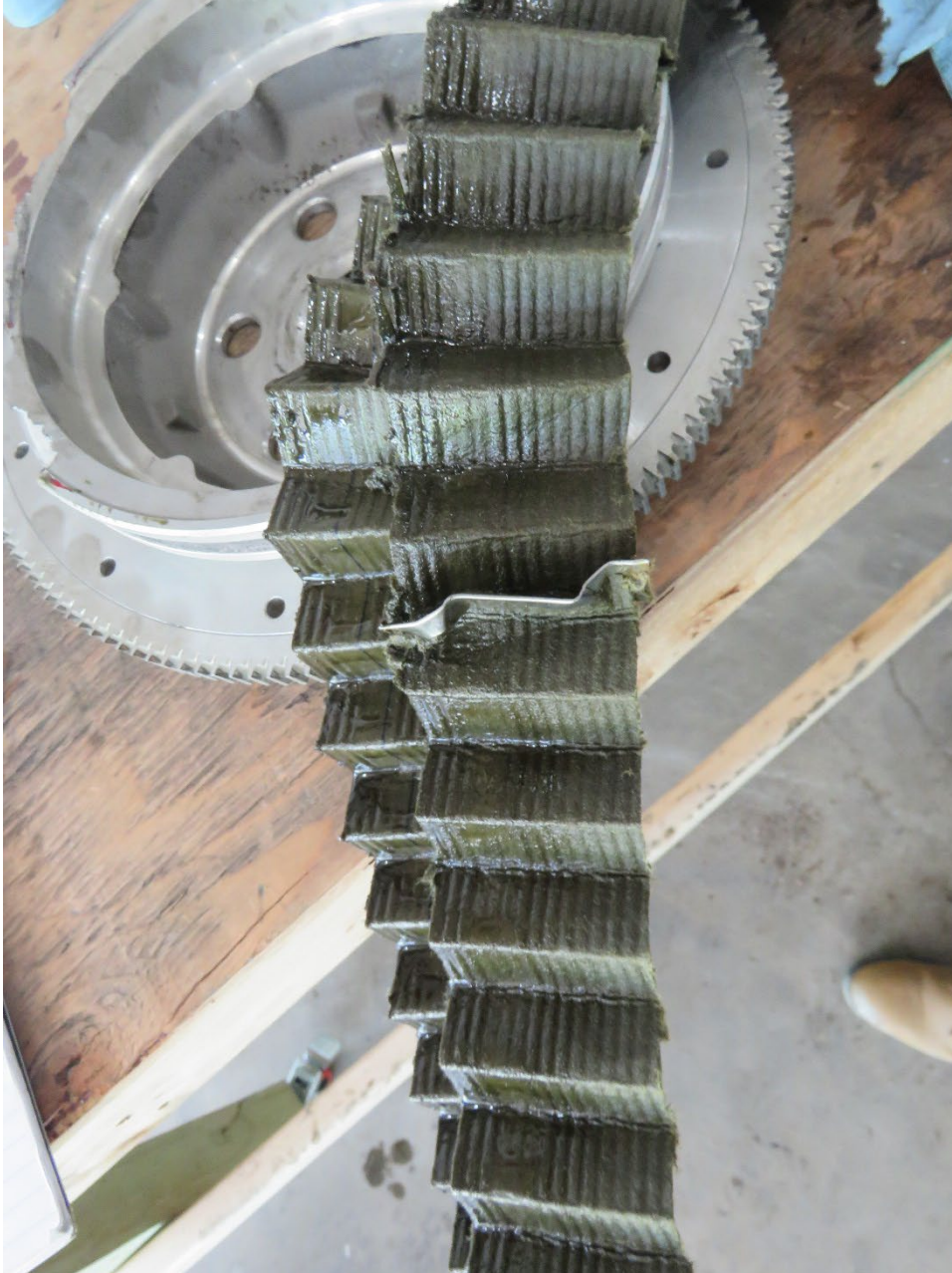
Photo 54: Oil filter pleats free of debris. (Lycoming Photo)
