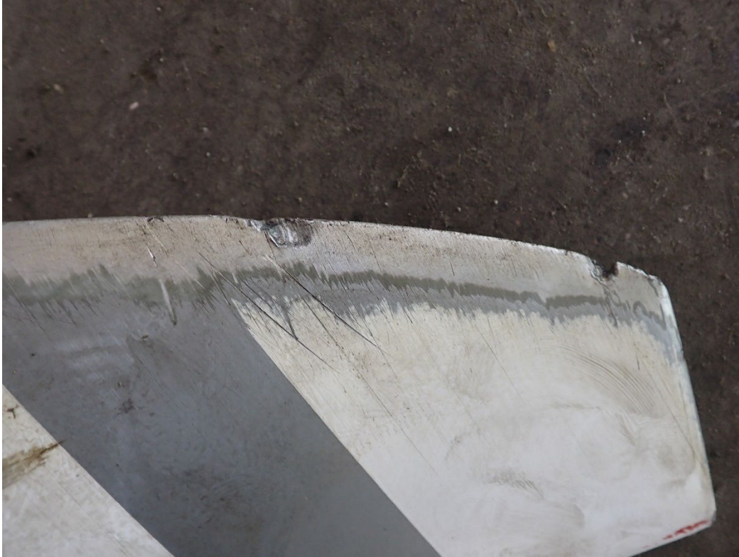
Photo 60: Blade A leading edge gouging, polishing and chordwise scratching.
