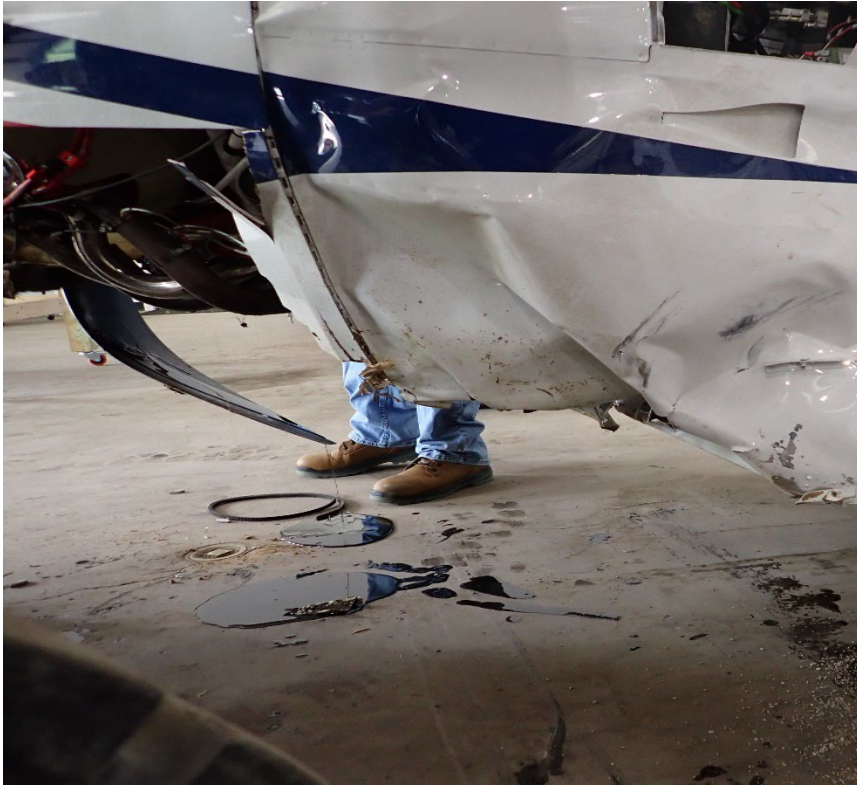
Photo 3: View of the forward fuselage crushed up and aft.
