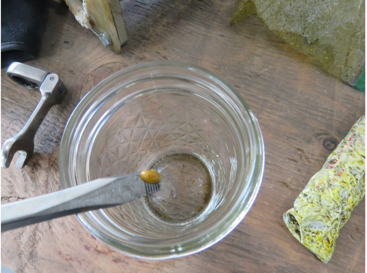
Photo 52: Fuel from the fuel injector unit with water test paste. (Lycoming Photo)
