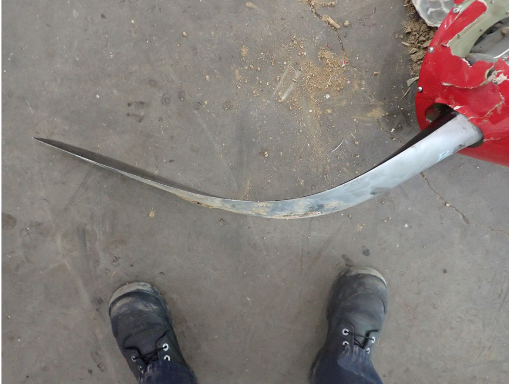
Photo 62: View of the bend in blade B.
