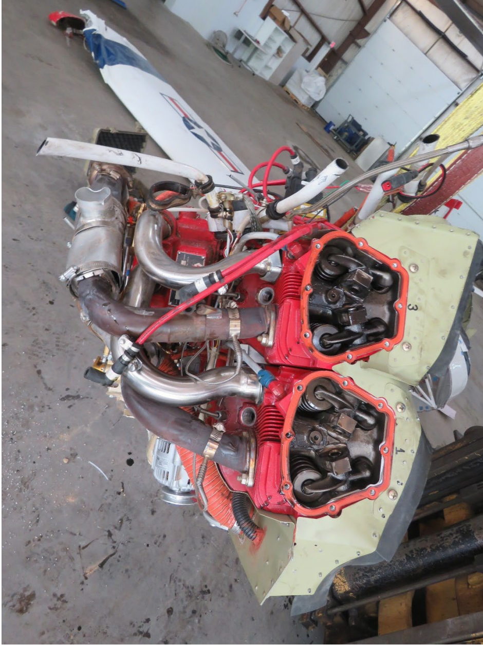
Photo 39: Engine suspended for examination with rocker covers removed. (Lycoming Photo)
