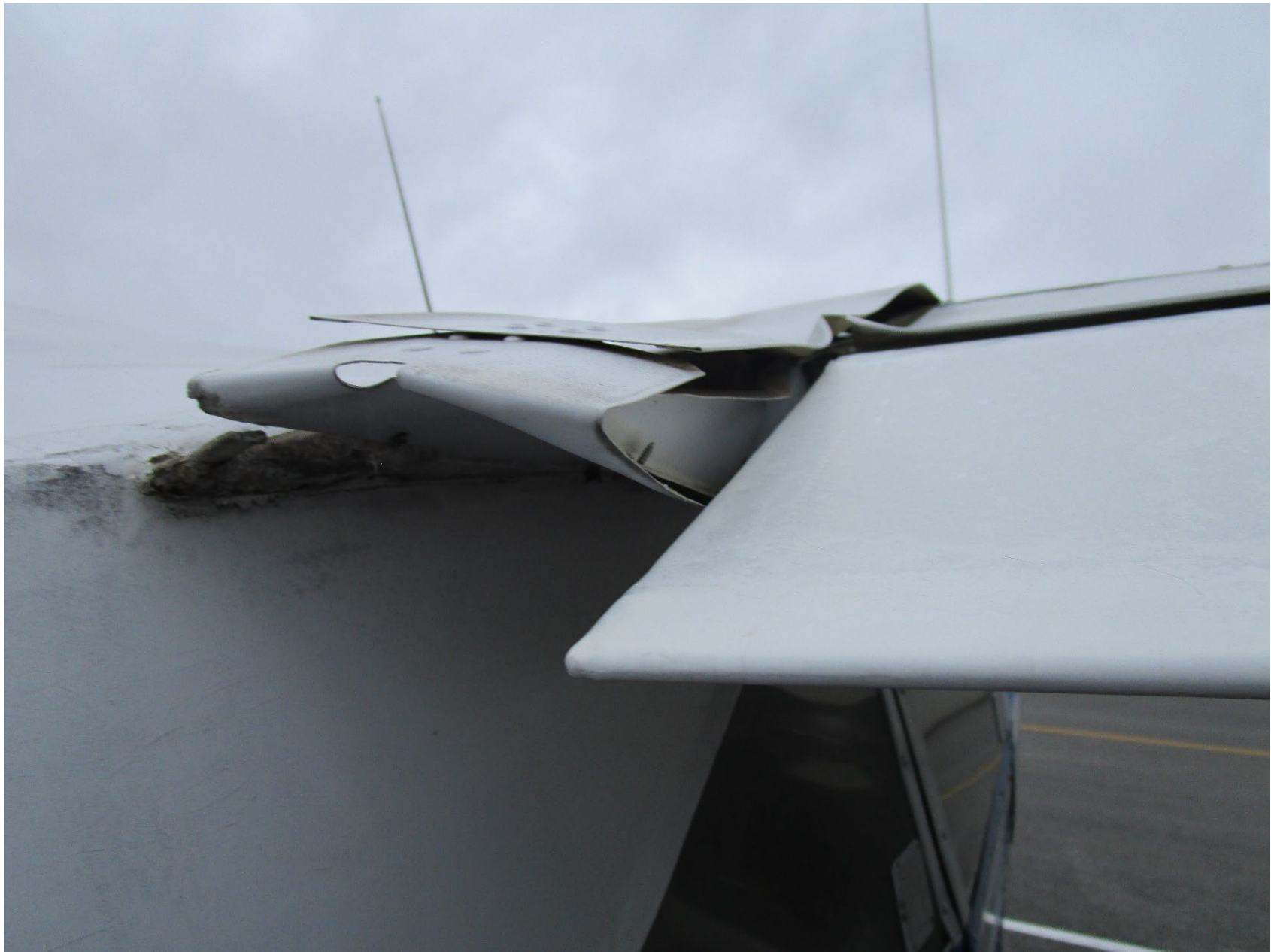
Photo 6 – View of damage at the right wing root and fuselage (Photo courtesy of FAA)
