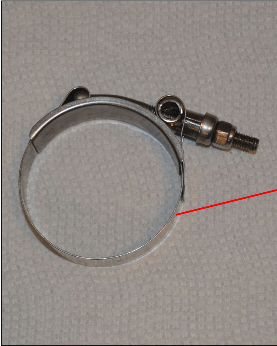
Photos 4, 5: Turbo air intake hose clamp and the turbocharger missing its clamp (Photo Courtesy of Pilot)
