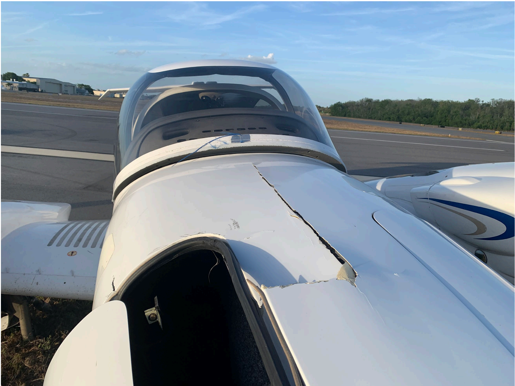
Photo 2 - Embry-Riddle Digital Photograph. Frontal View of the Airplane. Note the Split on the Top Center Portion of the Carbon Fiber Reinforced Polymer Molded Construction Fuselage From Just Forward of the Windshield to About ½ Way Along Nose Section Baggage Compartment Door.
