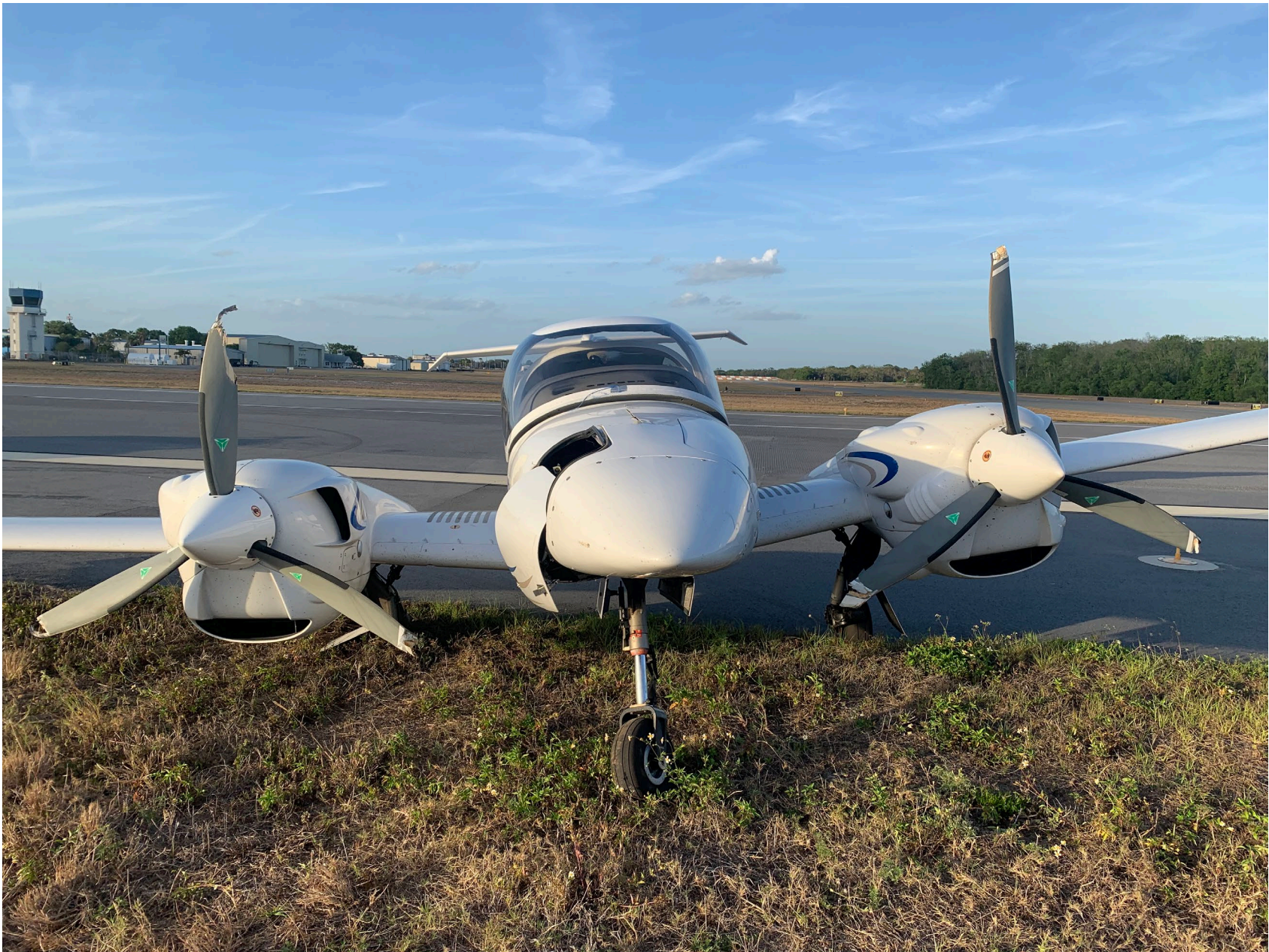
Photo 1 – Embry-Riddle Digital Photograph. Frontal View of the Airplane. Note the Partially Collapsed Right Main Landing Gear.
