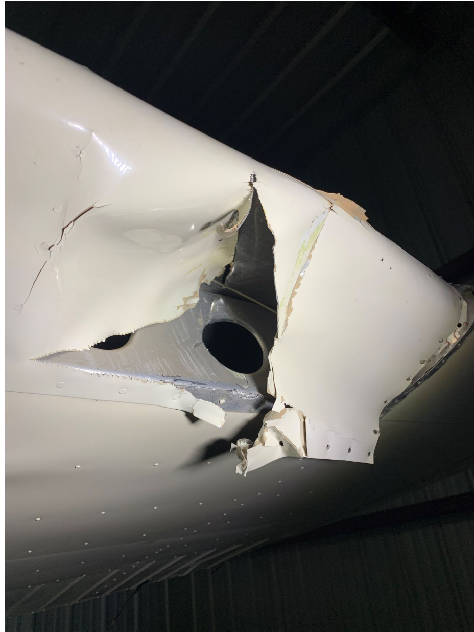
Photo 1: Left wing damage to N7772B
