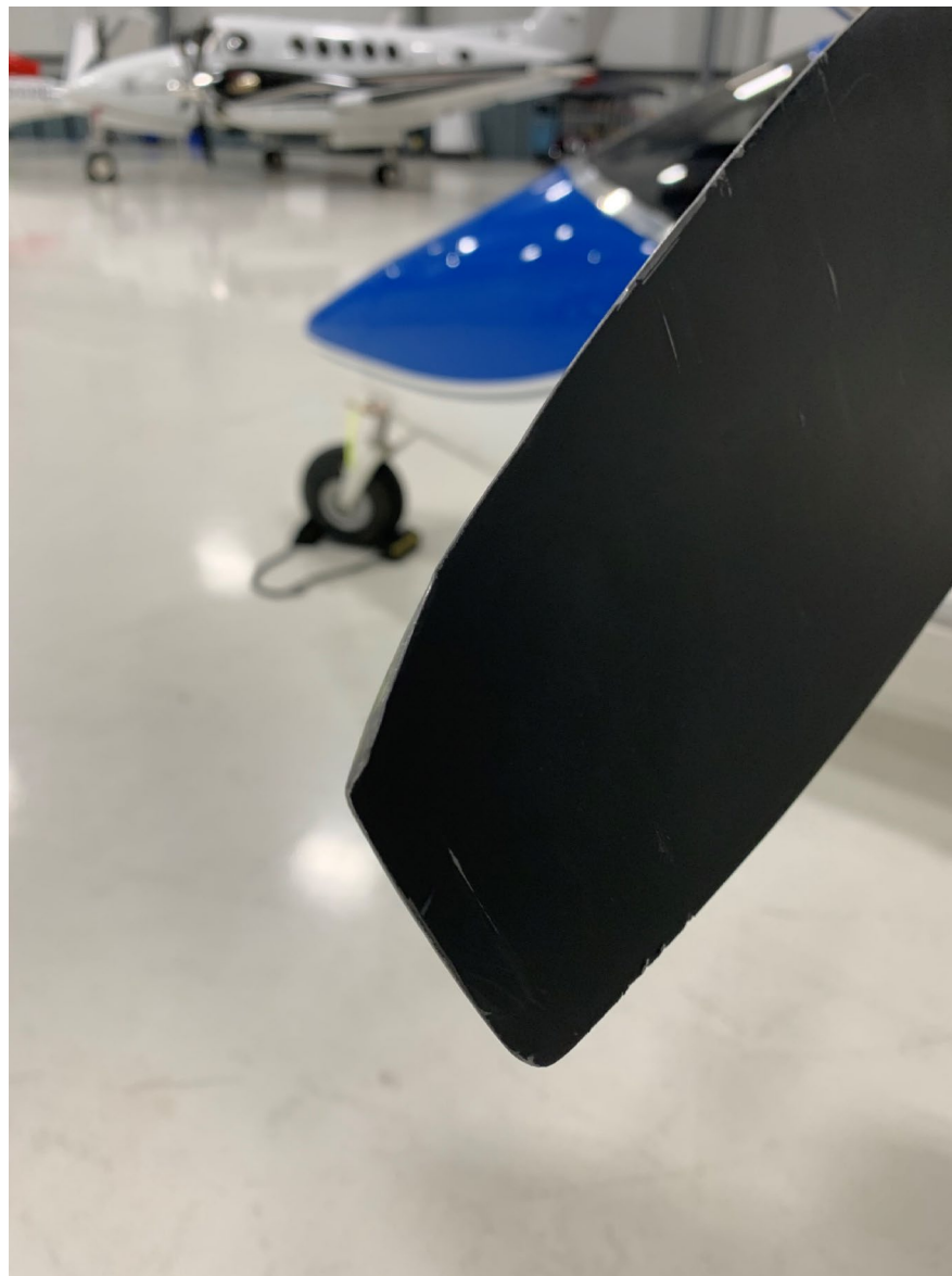
Photo 3: View of right propeller damage to N920AA
