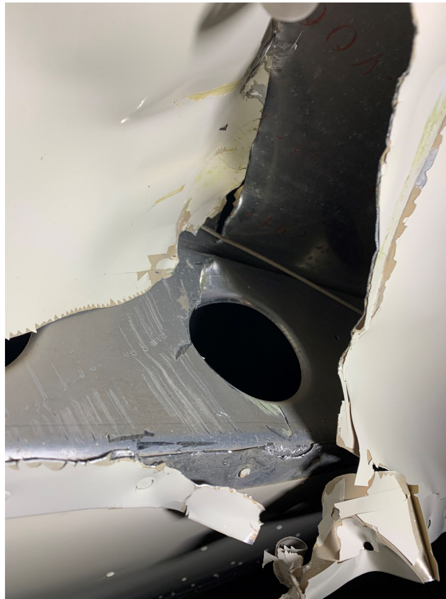
Photo 2: Close-up view of left wing damage to N7772B. Note damage required a form 337 for major repair.
