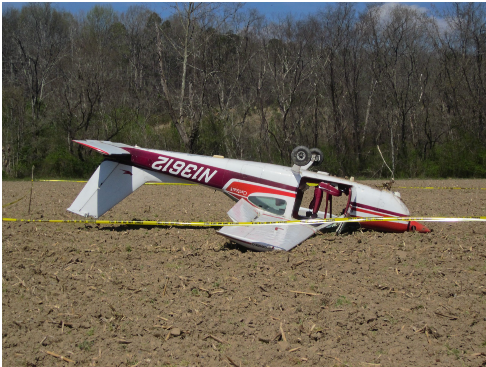
Photo 1 – FAA Digital Photograph. View of the Left Side of the Inverted Airplane. Note the Damage to the top of the Vertical Stabilizer.
