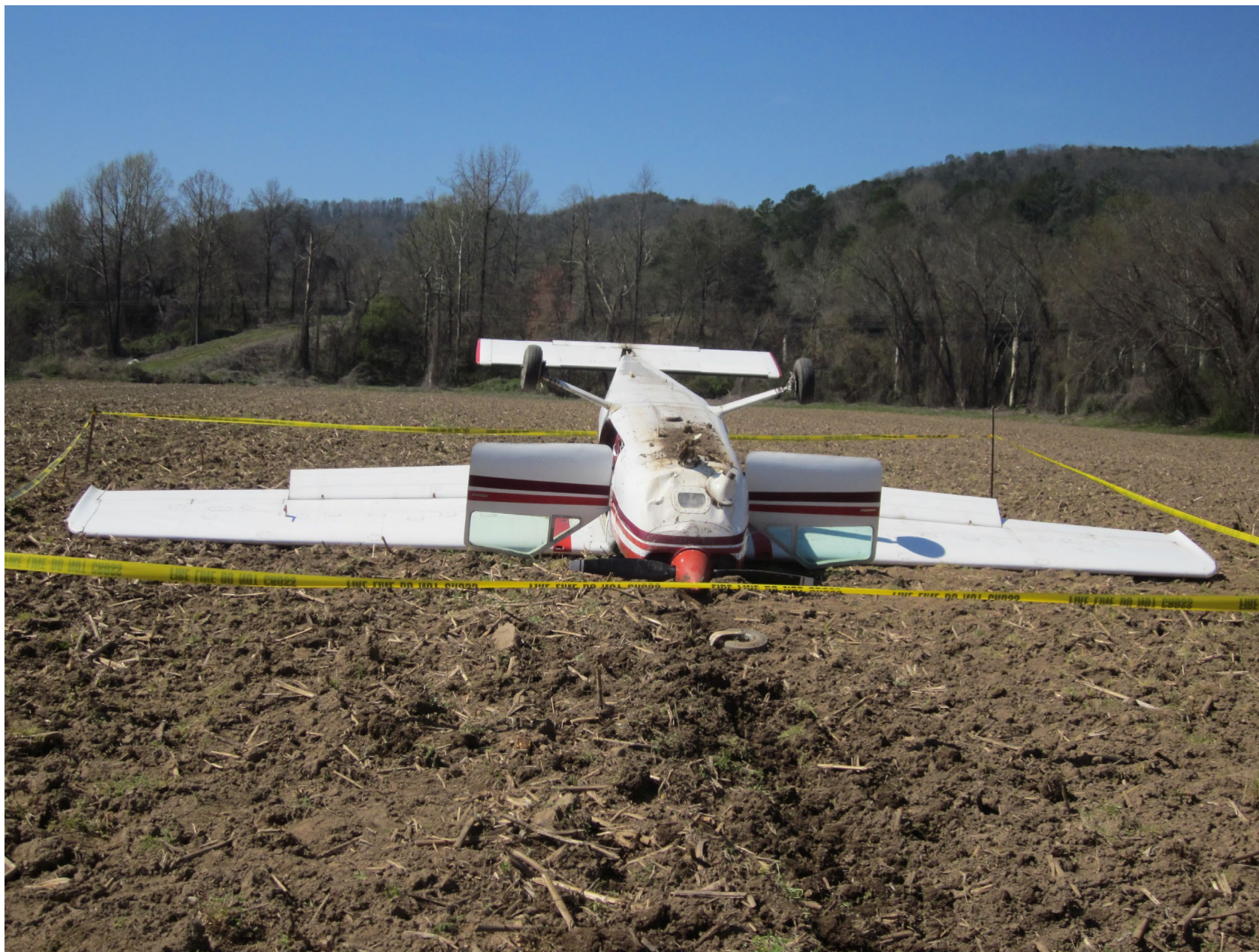
Photo 2 - FAA Digital Photograph. Front View of the Inverted Airplane. Note the Lack of Damage to the Propeller.
