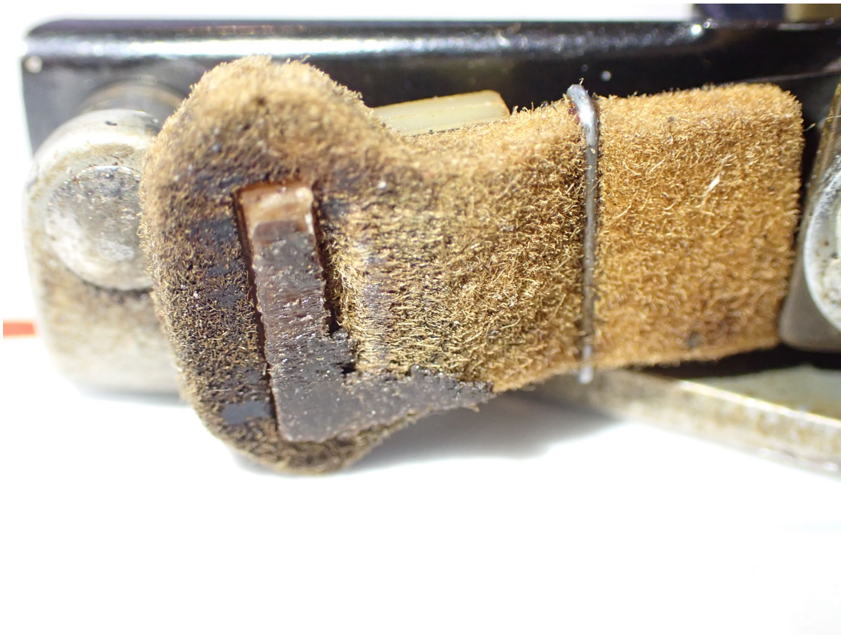
Photo 6 – NTSB Digital Photograph. Close-Up View of the Left Cam Follower and Felt. Note the Heat Discoloration and Distortion of the Cam Follower.
