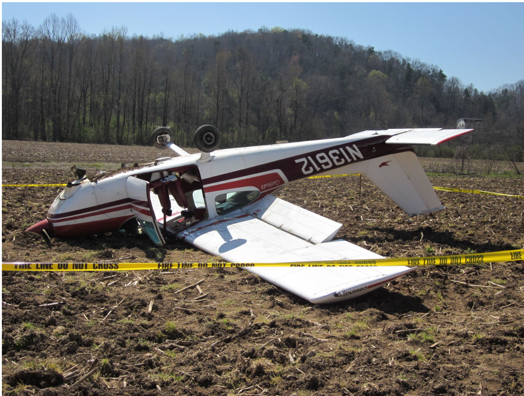
Photo 3 - FAA Digital Photograph. View of the Right Side of the Inverted Airplane. Note the Wrinkles on the lower Right Wing Skin near the Wing Root.
