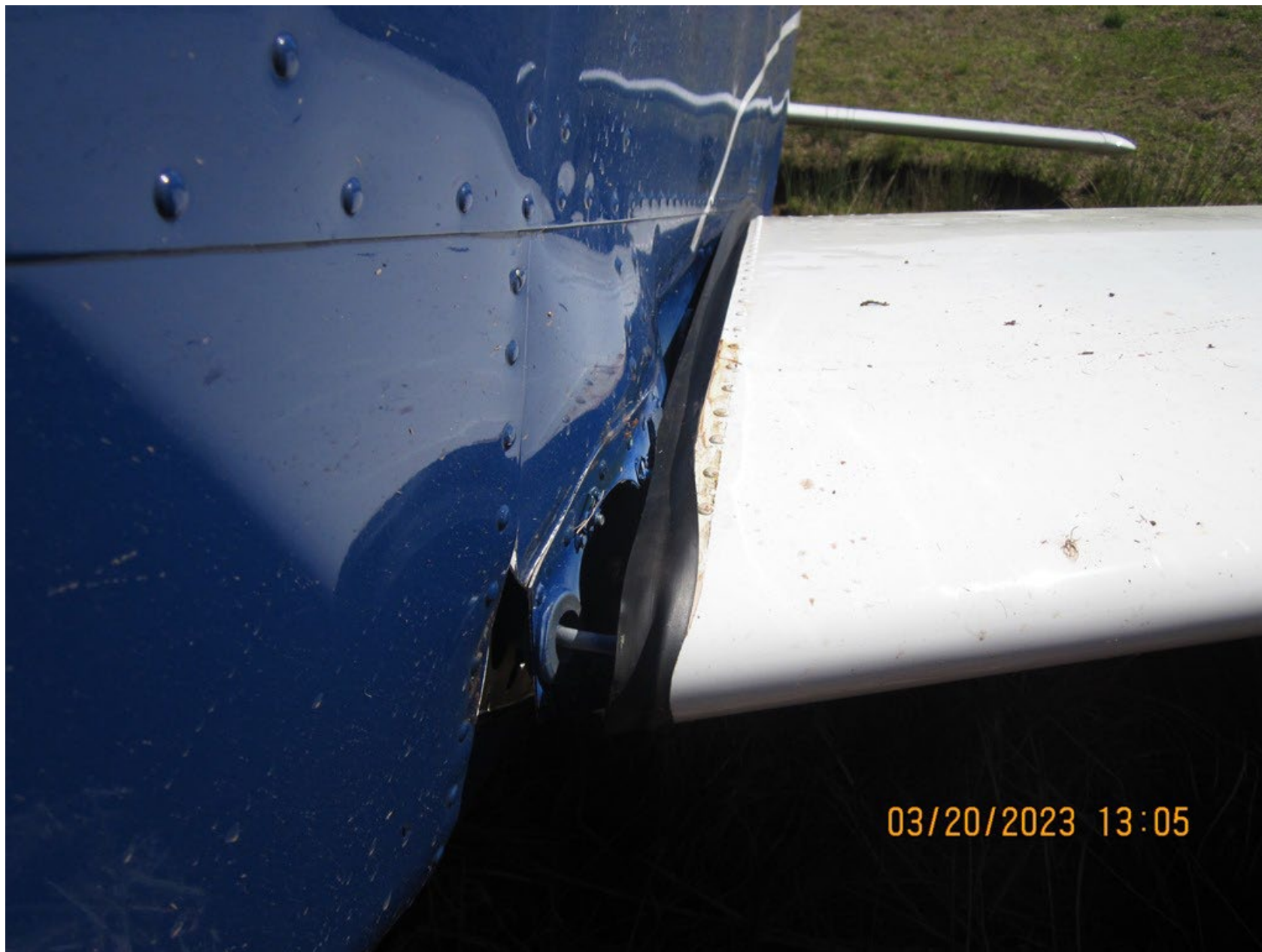
Photo 3 - Damage to LH Wing at Root (FAA)
