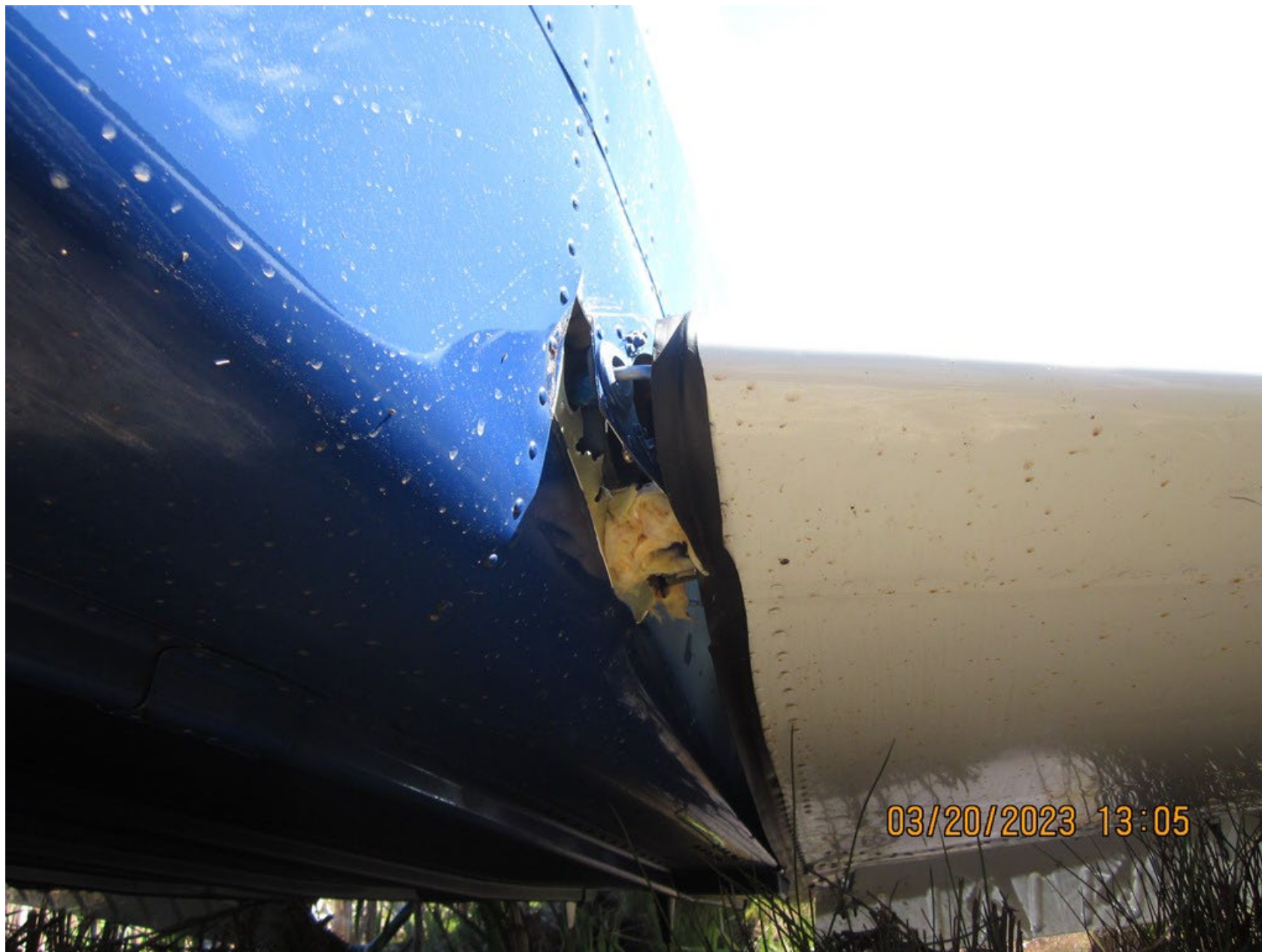
Photo 4 – Damage to LH Wing at Root (FAA)
