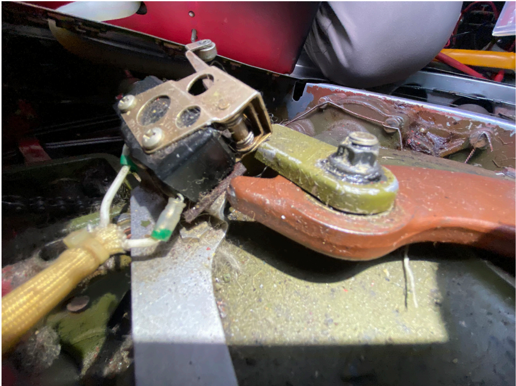
Photo 3 – View of Bent Landing Gear Switch Mount (Thoroughbred Aviation)
