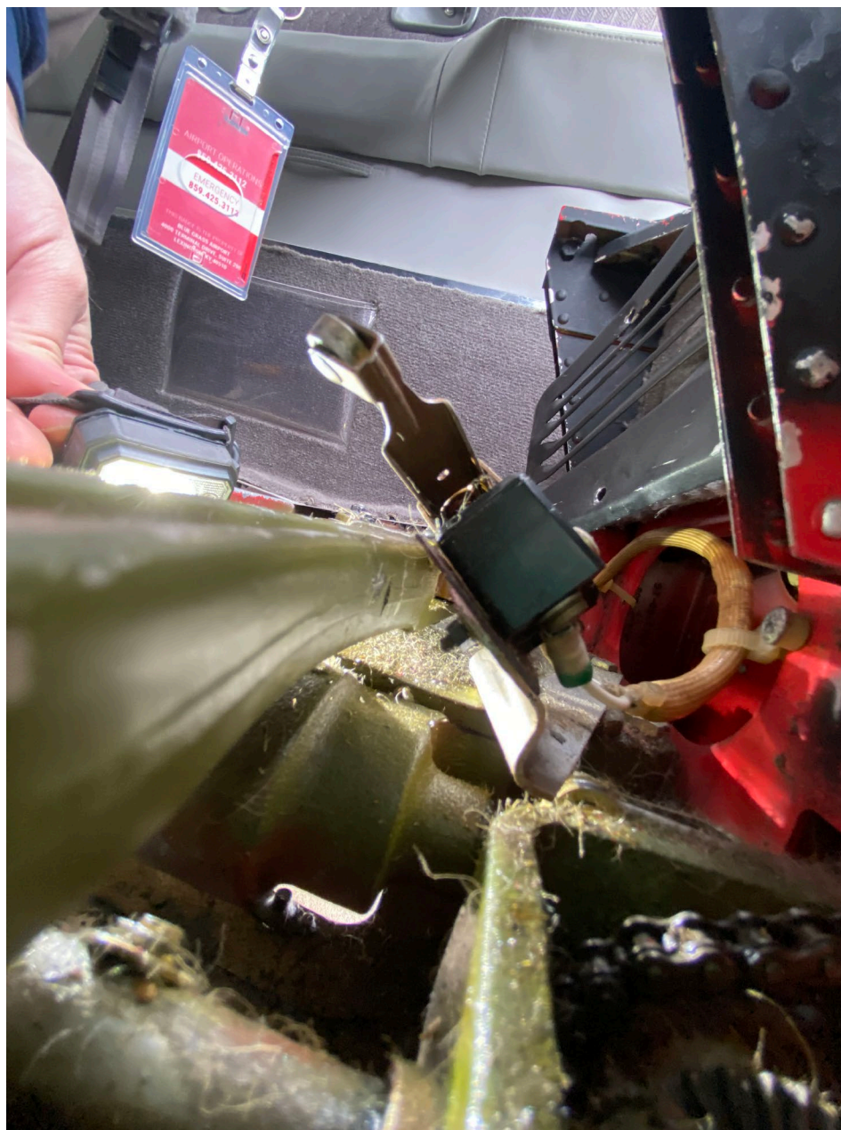
Photo 4 – Profile View of Bent Down-Lock Switch Mount (Thoroughbred Aviation)
