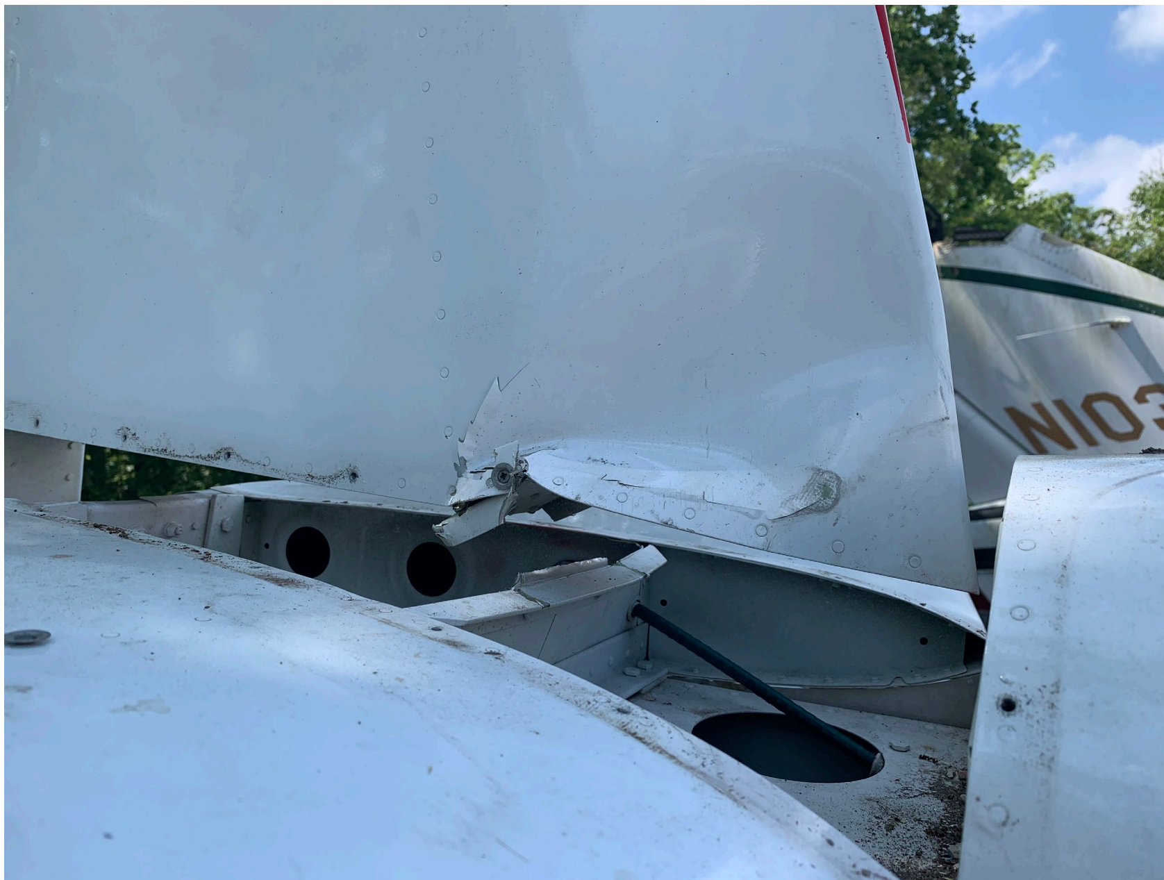
Photo 6 – FAA Digital Photograph. View Showing the Fractured Forward Structure of the Vertical Stabilizer.
