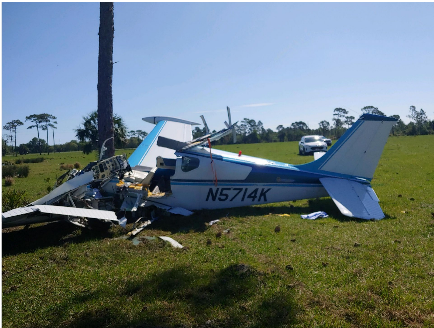
Photo 2 – Left side view of airplane showing cockpit damage. (FAA Photo)
