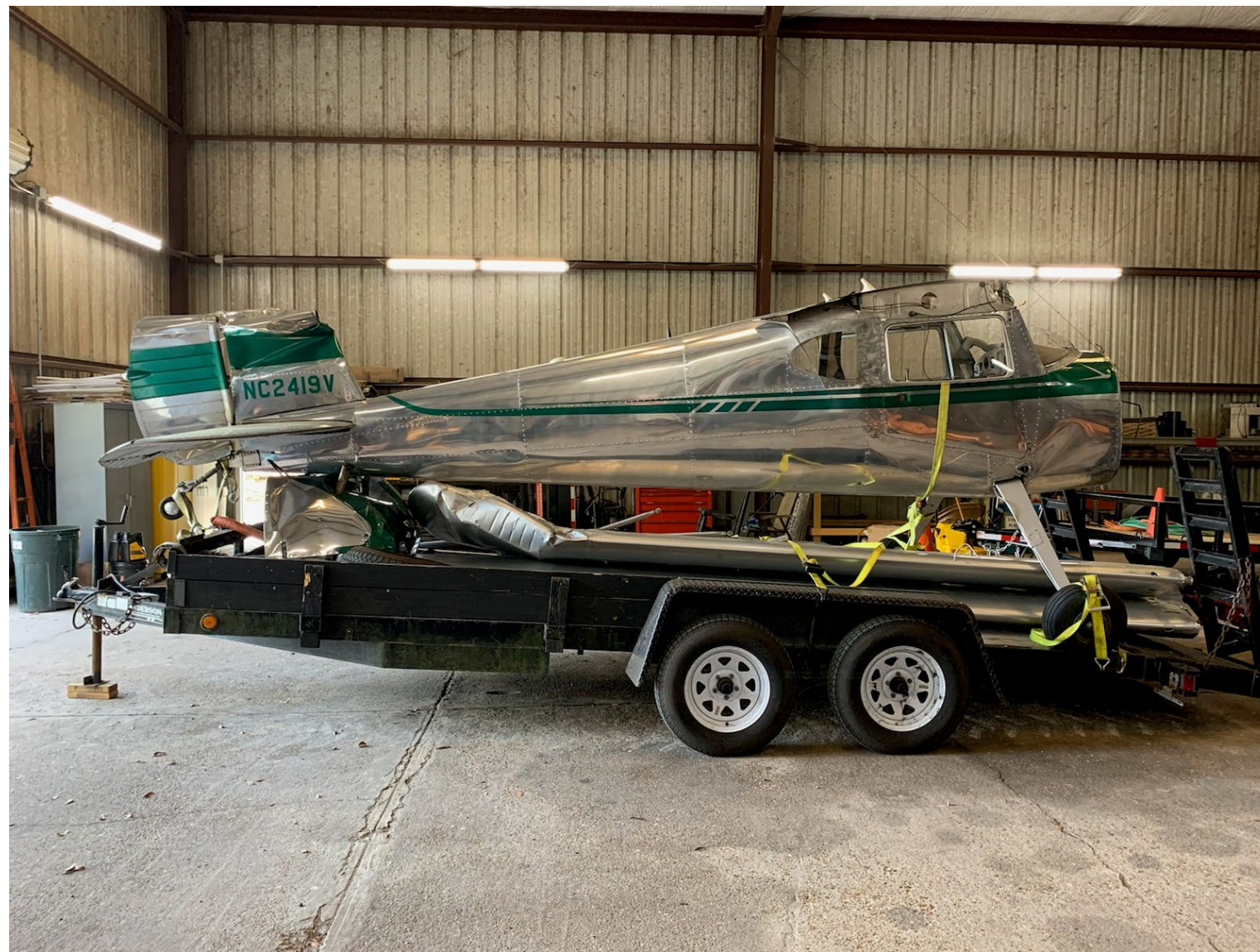
Photo 3: Overview of the airplane in a hangar after recovery with damage to the wings and tail (Photo Courtesy of FAA)
