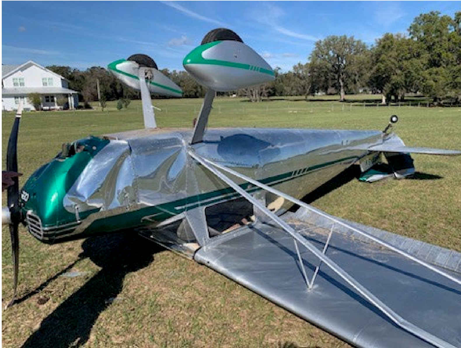
Photo 2: Overview of the airplane as it lay in the field with damage to the fuselage, vertical stabilizer and rudder (Photo Courtesy of FAA)
