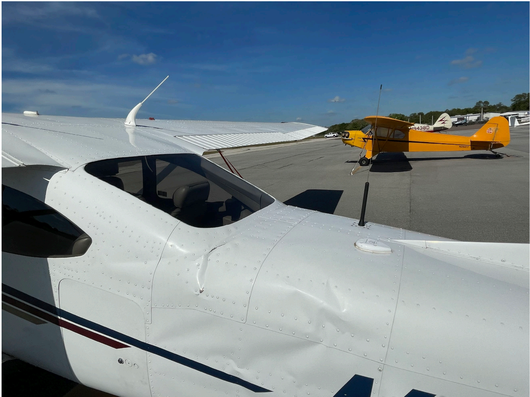
Photo 2 – Aft Fuselage Damage (Left Side) – Courtesy of FAA
