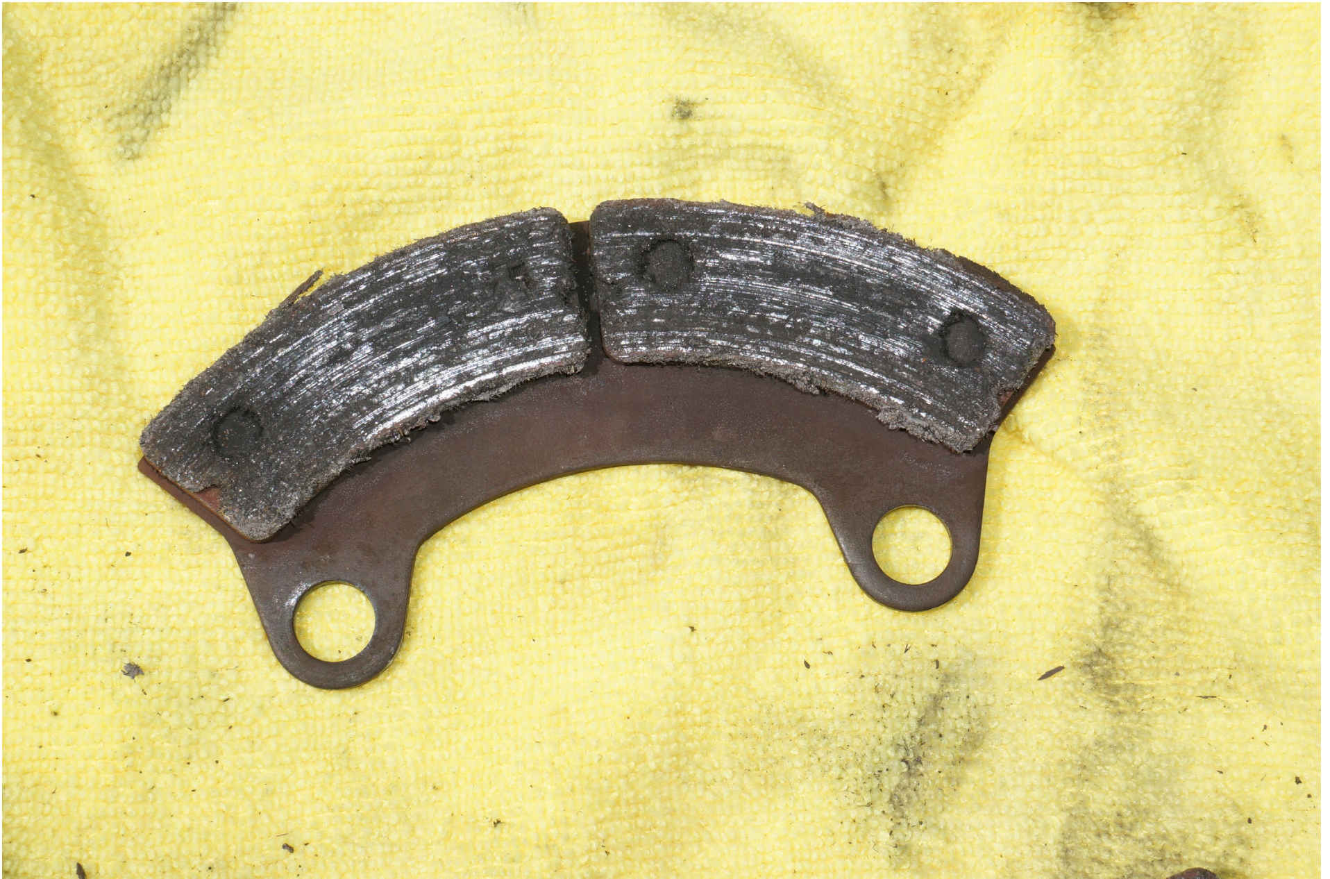
Photo 18 – Close Up of Brake Linings (Pressure Plate Side)
