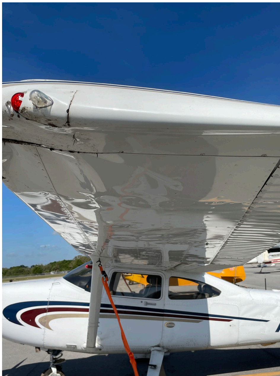
Photo 4 – Left Wing Damage – Courtesy of FAA
