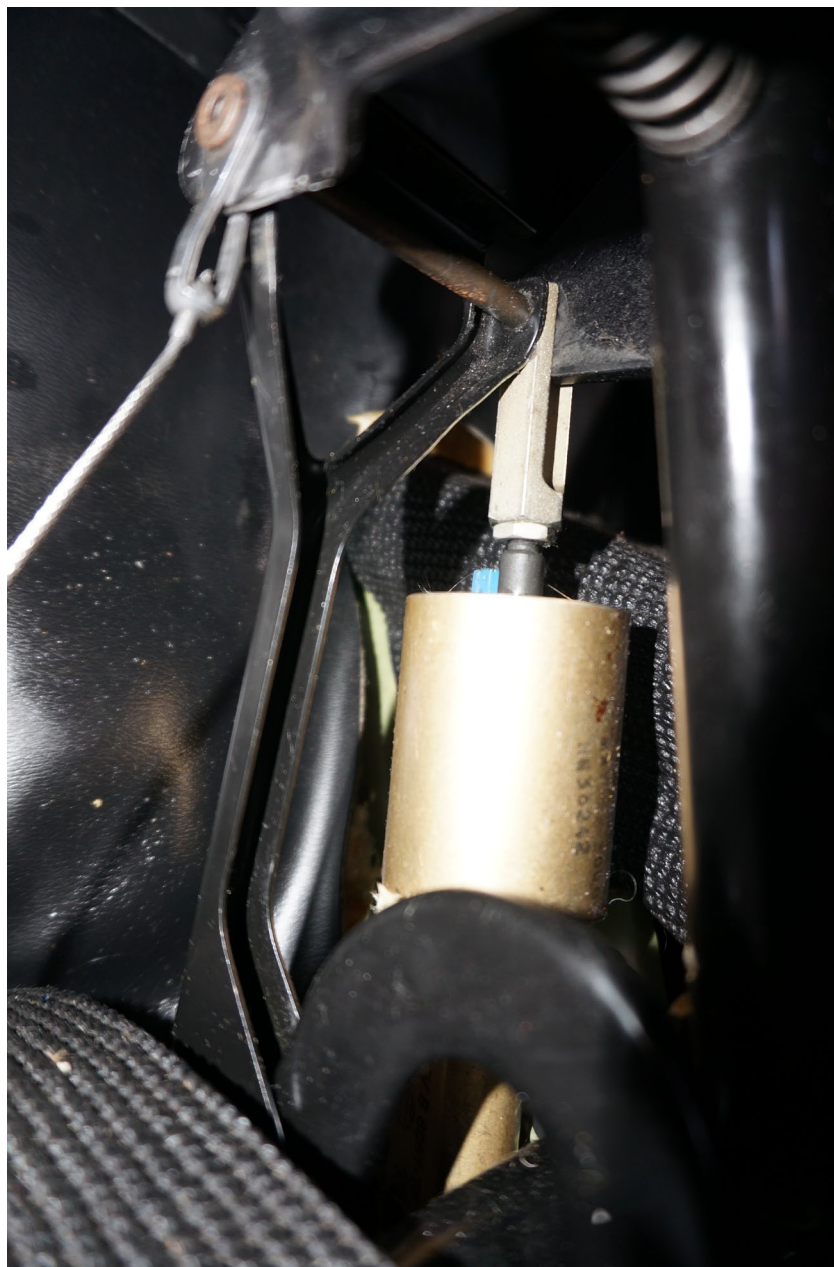
Photo 12 – Master Cylinder (Right Side)
