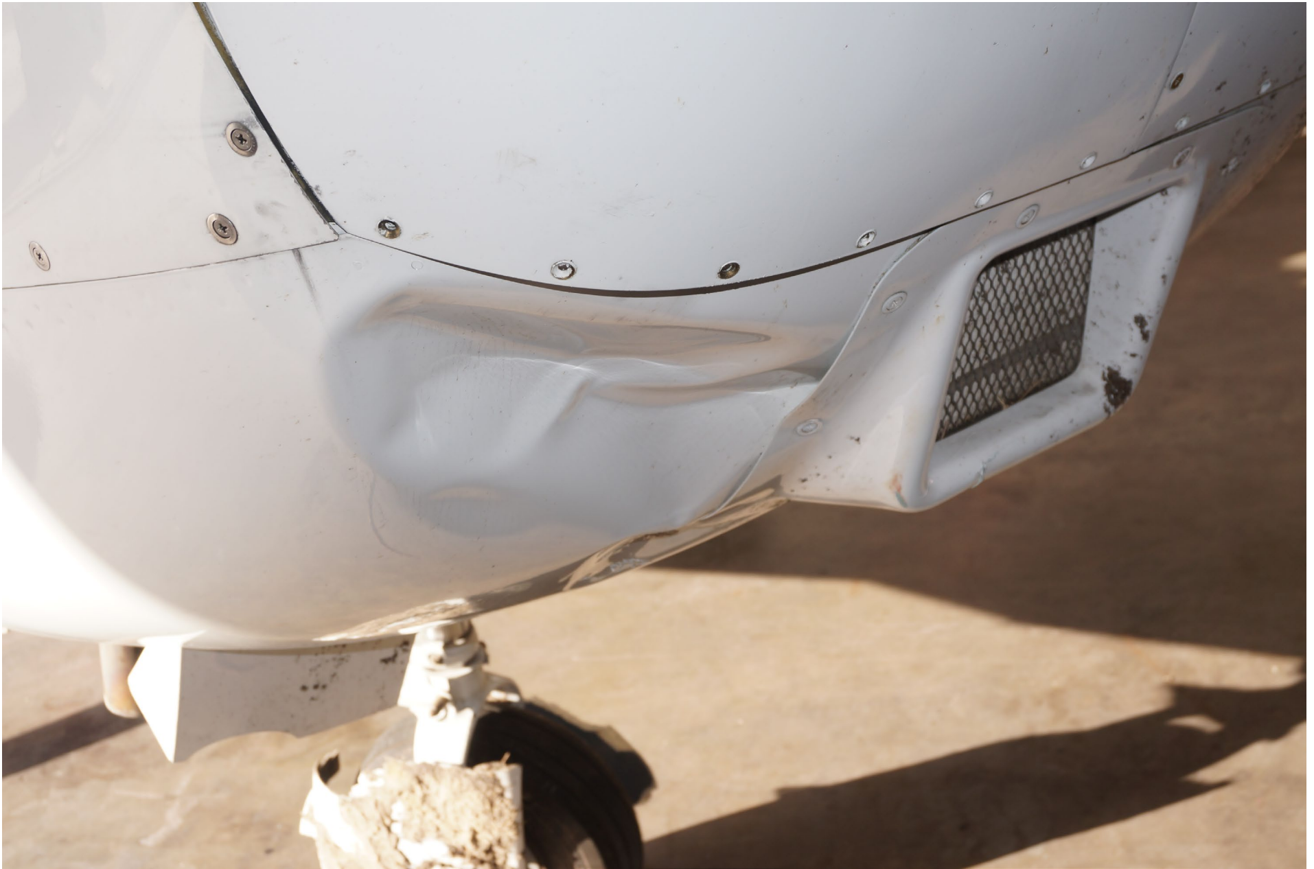
Photo 7 – Damage to Right Front Portion of Engine Cowling
