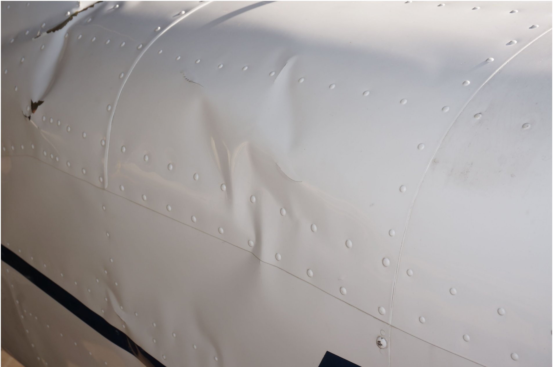
Photo 9 -Close Up of Aft Fuselage Damage (Left Side)
