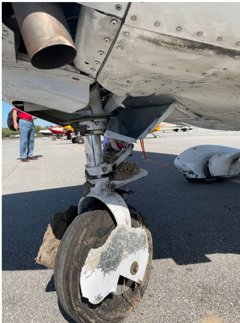
Photo 3 – Nose Landing Gear and Belly Damage (Left Side) – Courtesy of FAA
