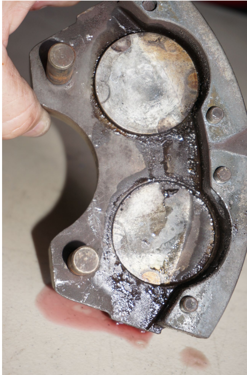
Photo 16 – Leakage from Upper Piston
