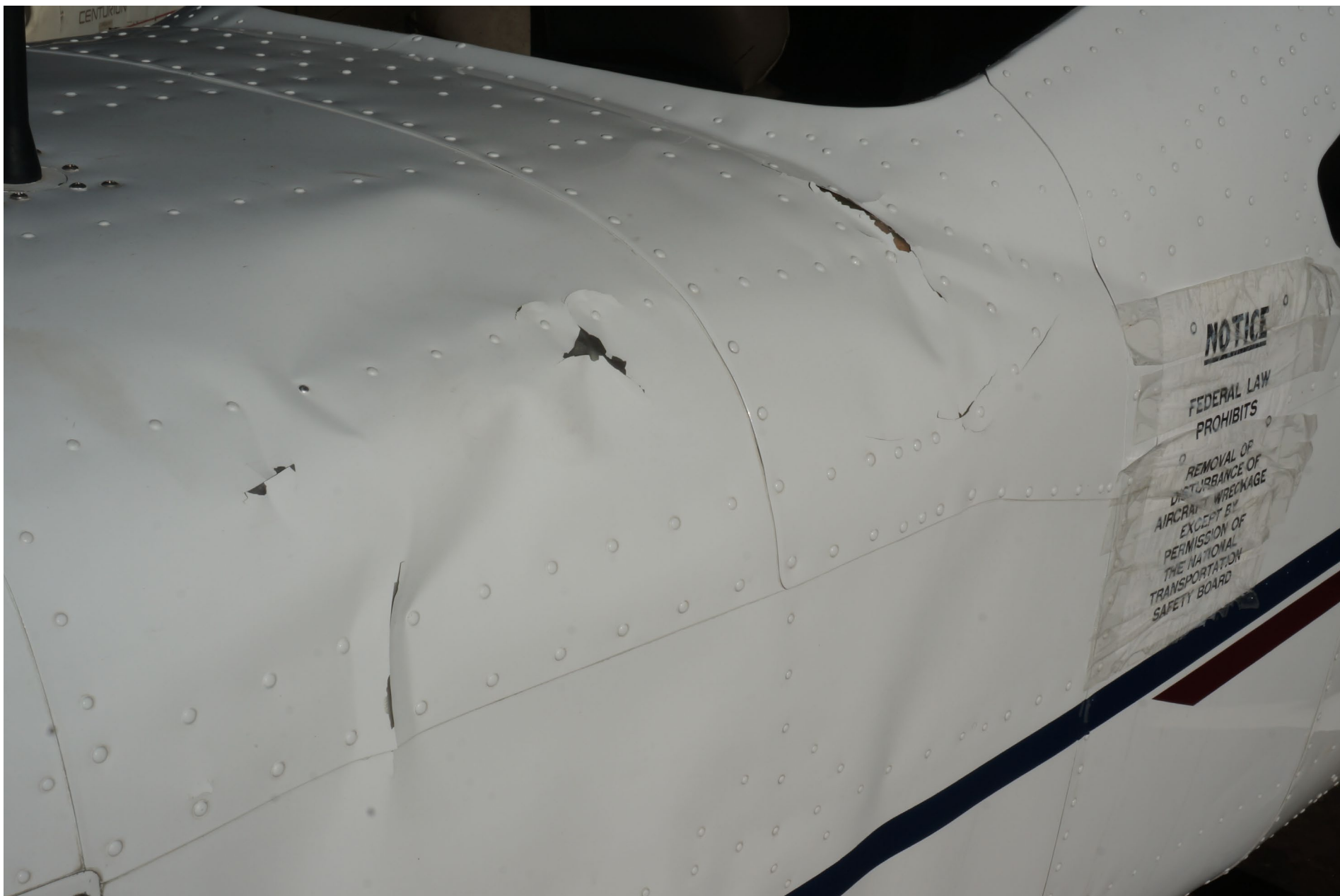
Photo 8 – Aft Fuselage Damage (Right Side)
