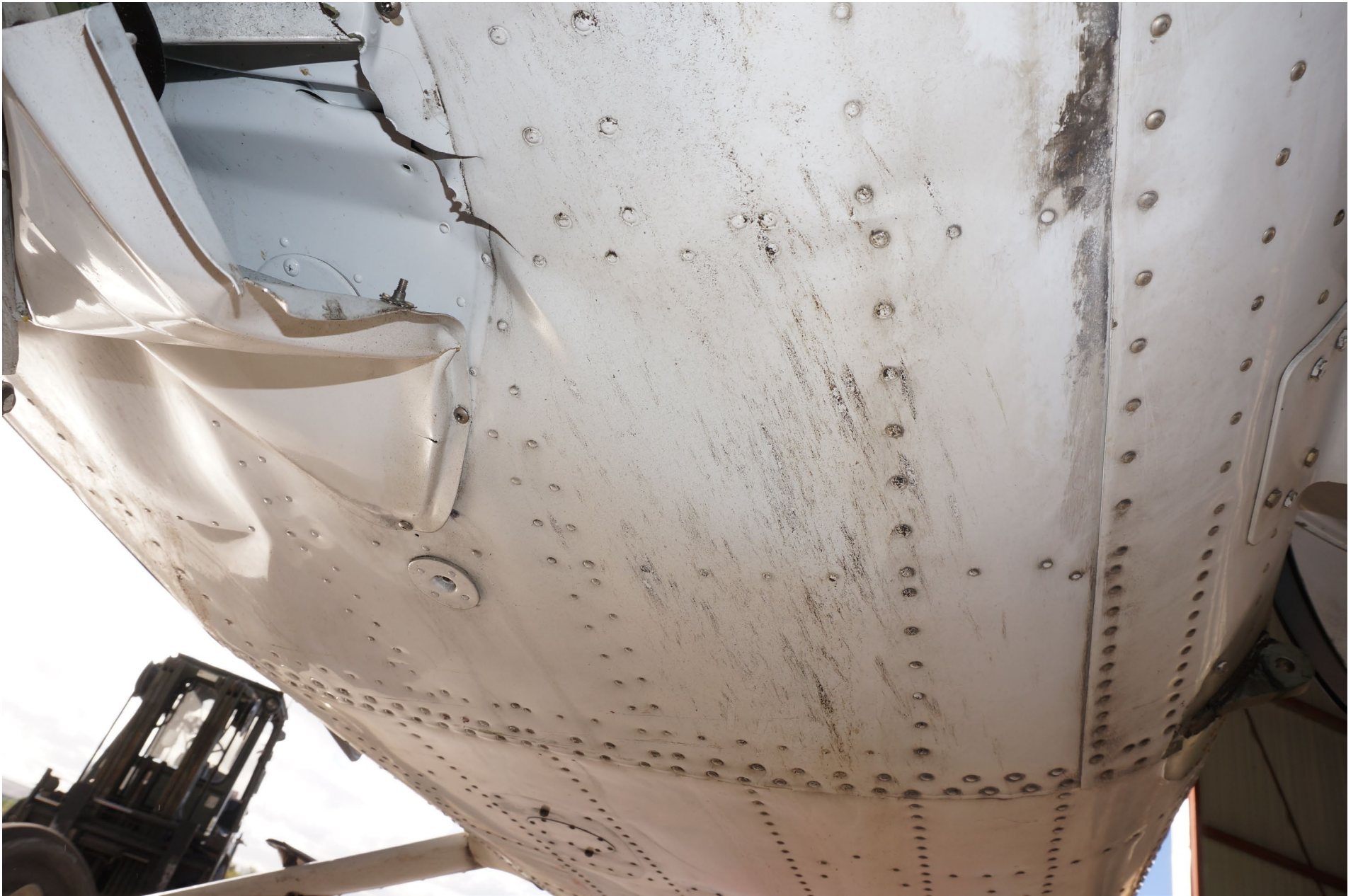
Photo 10 – Close Up of Belly Damage
