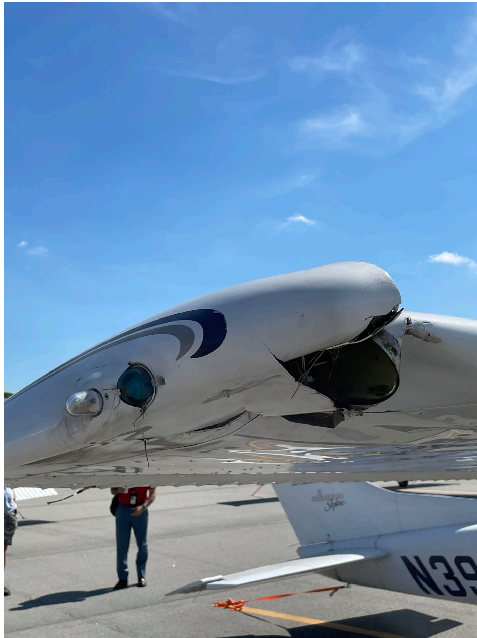
Photo 6 – Close Up of Right Wing Damage – Courtesy of FAA
