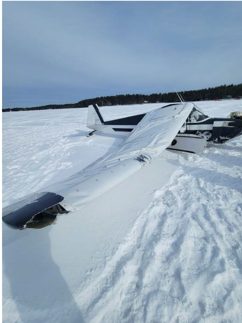
Photo 1 – View of right wight damage (FAA Photo)
