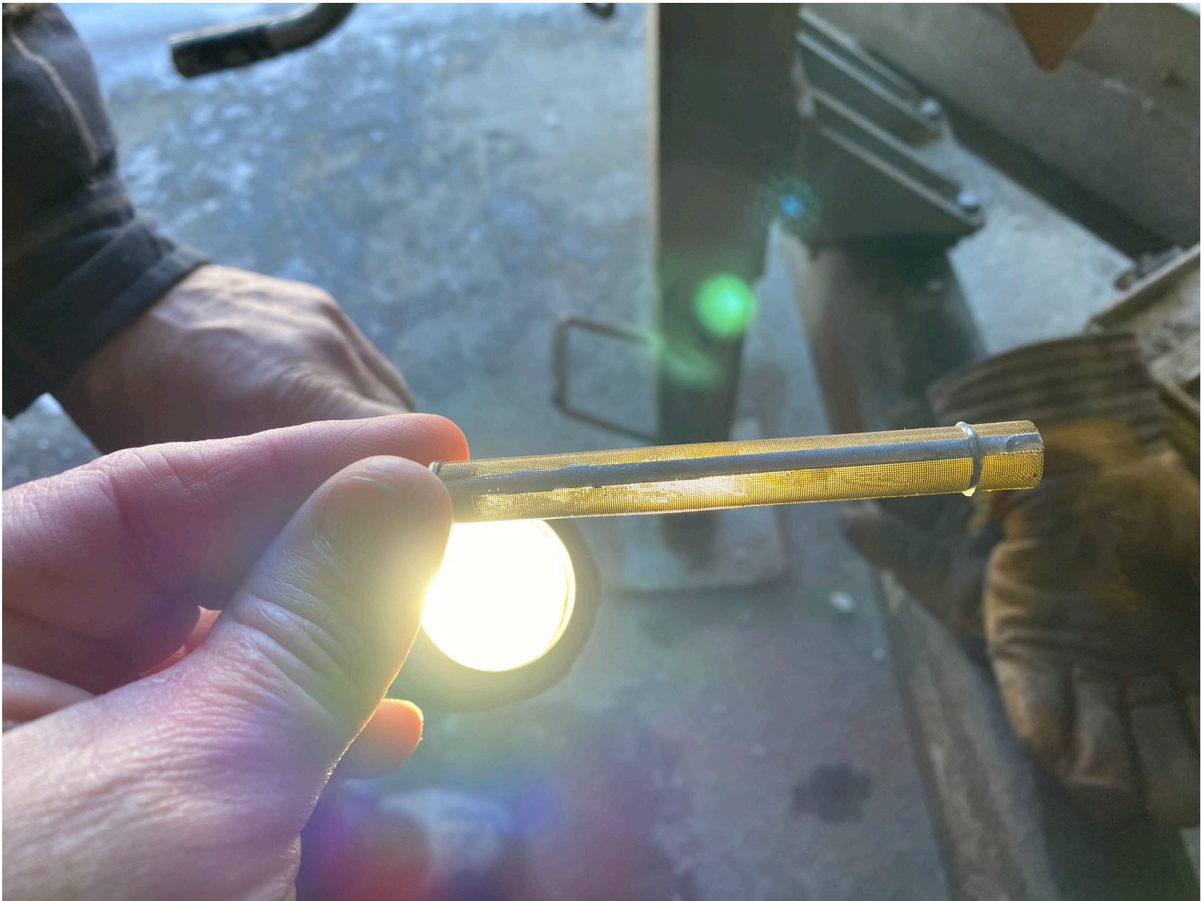
Photo 4 – view carburetor fuel screen (FAA Photo)
