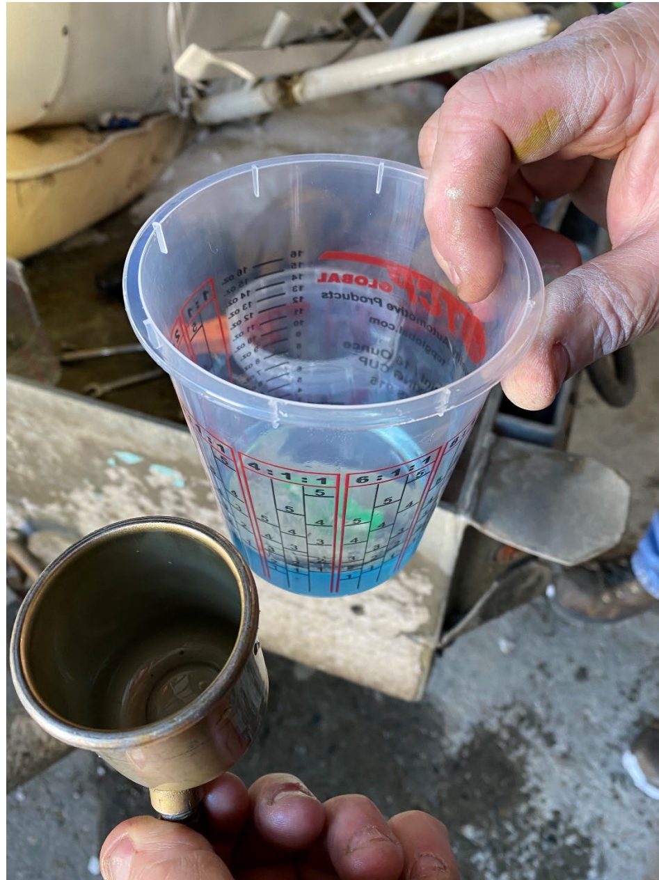
Photo 3 – View of Fuel removed from fuel strainer (FAA Photo)
