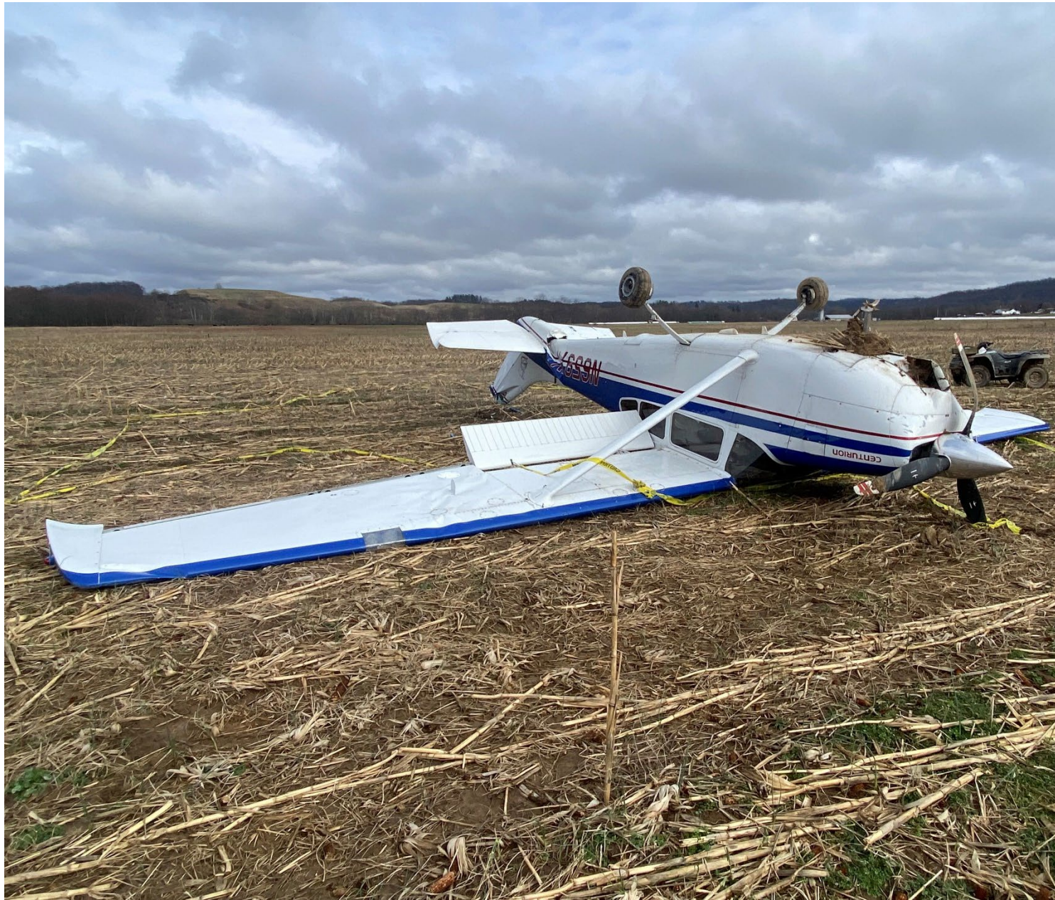
Photo 1 – AMF Aviation Digital Photograph. Left Forward Quartering View of the Inverted Airplane at the Accident Site. Note the Compression Wrinkles in the Lower Skin of the Left Wing Outboard of the Lift Strut.
