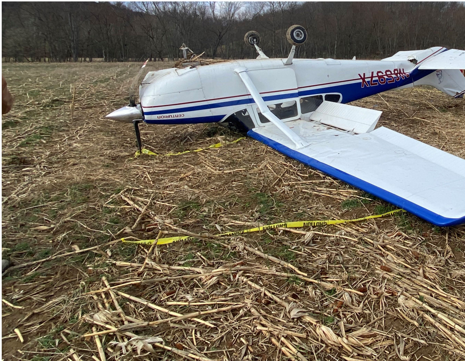
Photo 2 - AMF Aviation Digital Photograph. Right Side View of the Inverted Airplane at the Accident Site. Note the Damage to the Right Lift Strut, Compression Wrinkles in the Right Wing Lower Skin, and Damage to the Aft Fuselage.
