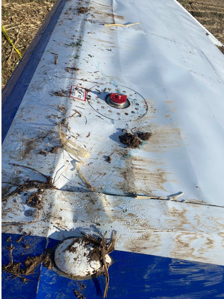
Figure 3: AMF Aviation Digital Photograph. View Looking Outboard Showing the Fuel Staining By the Right Fuel Filler Cap.
