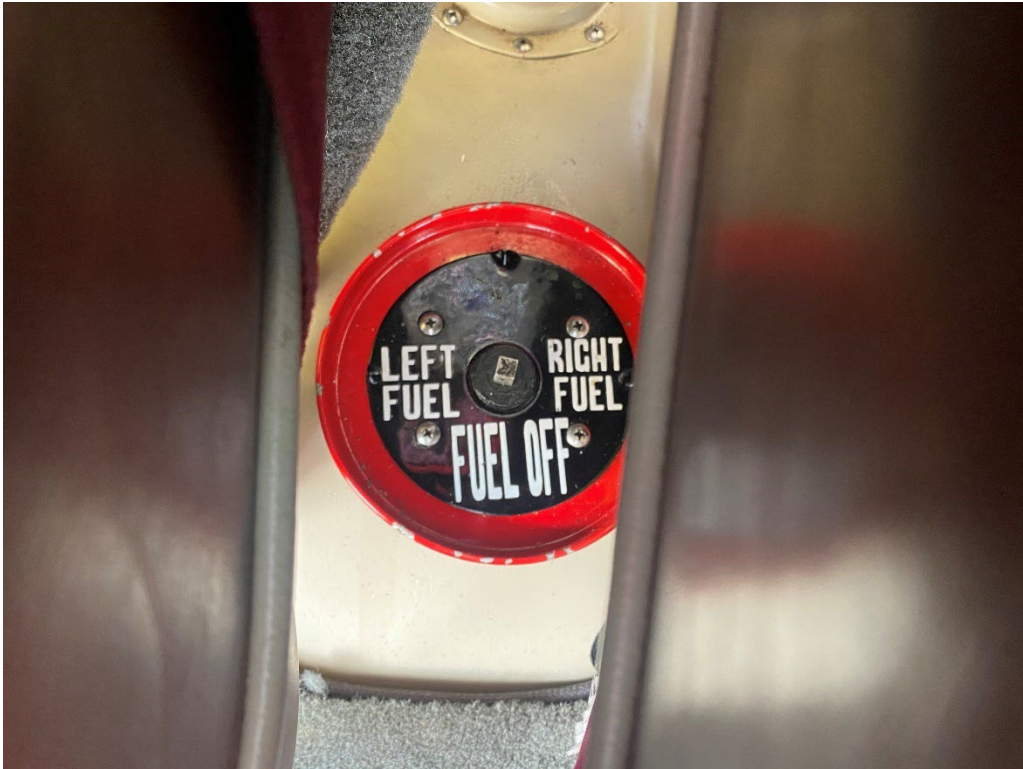
Figure 4: AMF Aviation Digital Photograph. View Showing the Fuel Selector Valve, Placard, and No Handle.
