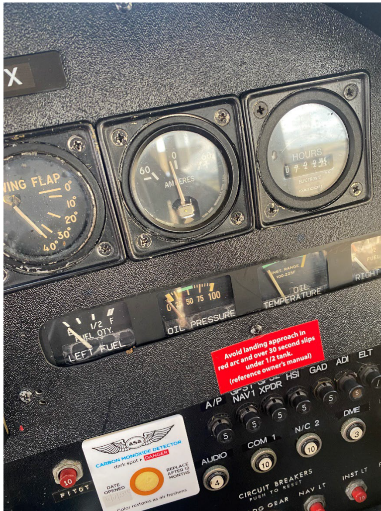
Figure 1: AMF Aviation Digital Photograph. View of a Portion Of the Instrument Panel With the Airplane Upright and Battery Power On Showing the Left Fuel Gauge at Empty and the Right Fuel Gauge Less than Empty.
