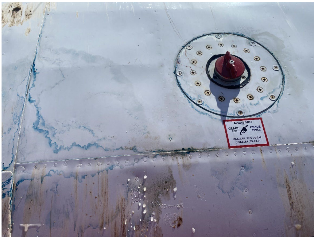
Figure 2: AMF Aviation Digital Photograph. View Looking Aft Showing the Fuel Staining By the Left Fuel Filler Cap.
