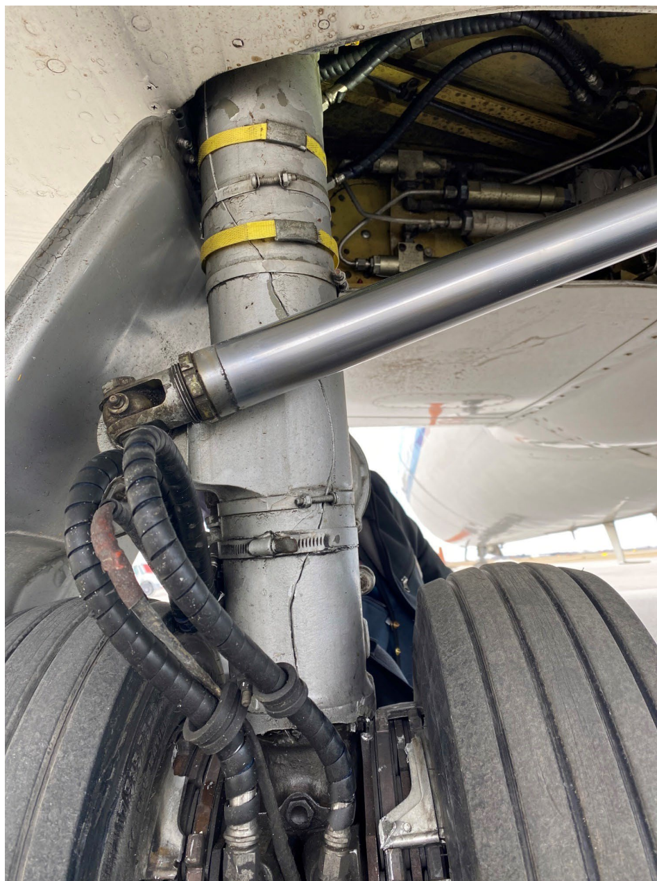
Photo 2 - View of Fractured Landing Gear Leg and Fractured Brake Caliper Retention Caps (FAA)
