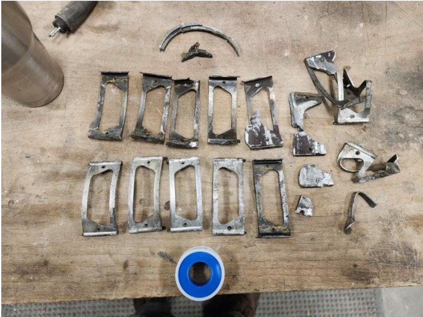
Photo 3 - View of Fractured Brake Caliper Retention Caps Harvested from Runway (FAA)
