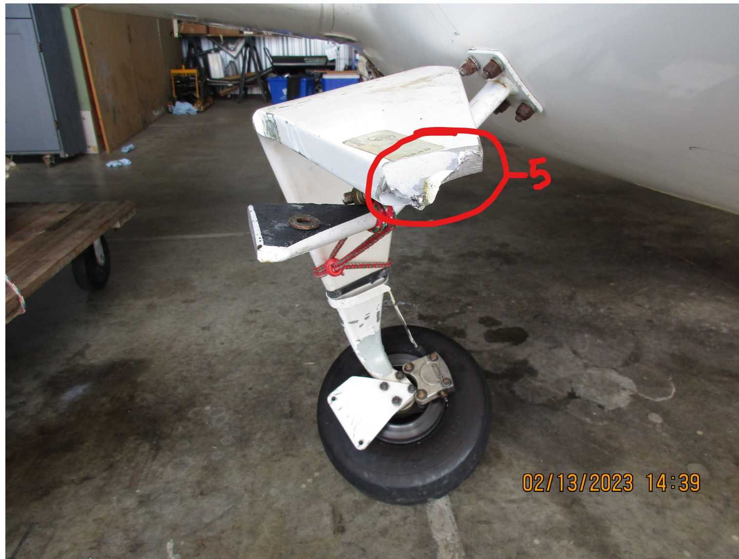
Photo 3: Main Landing gear which sheared off during collapse (Photo Courtesy of FAA)
