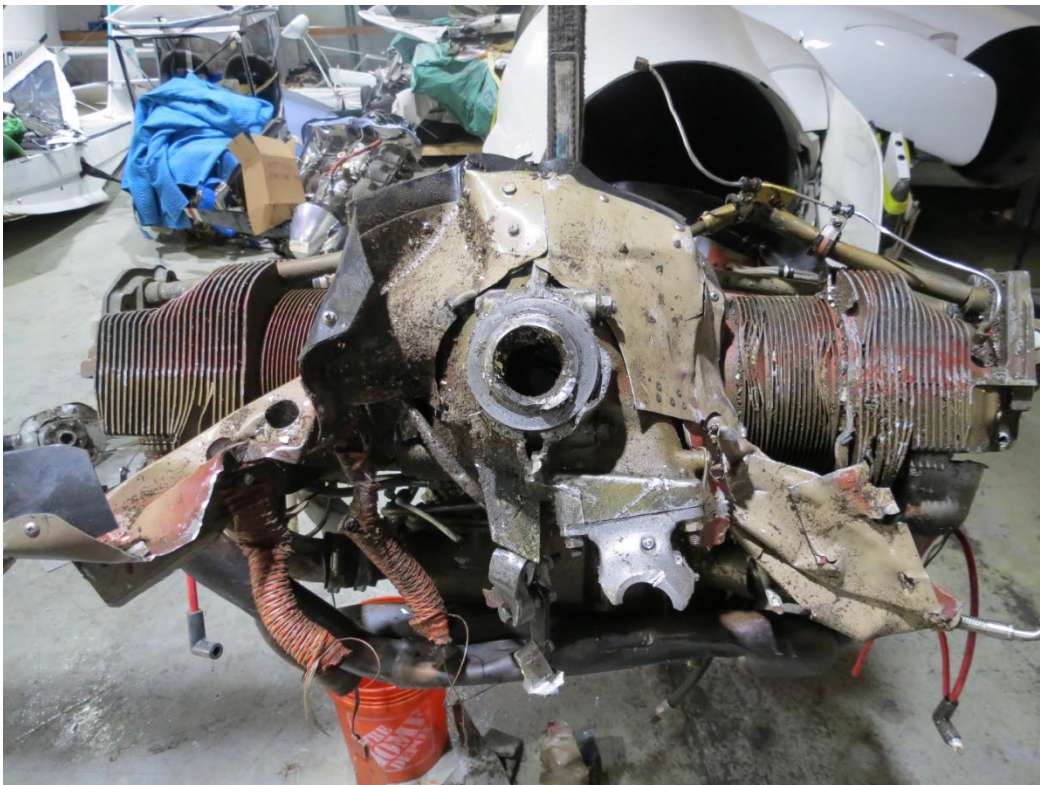
Photo 3: View of engine from the front with heat shielding and rocker covers removed.
