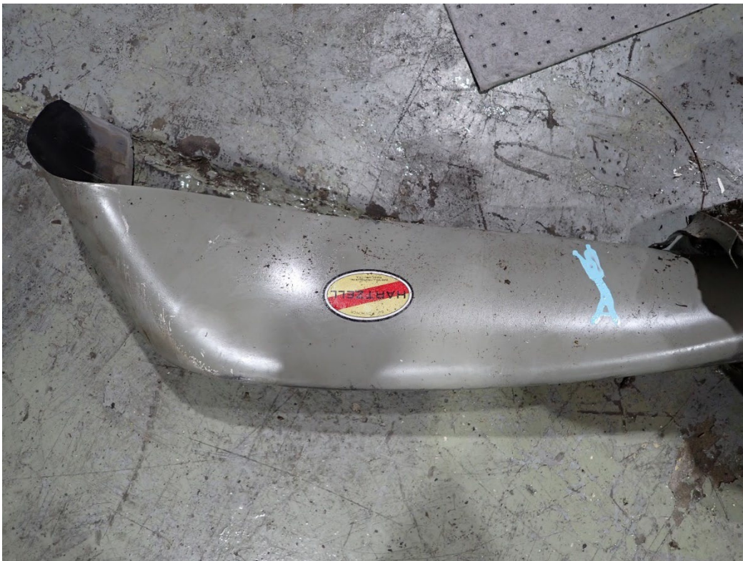
Photo 27: Camber side of propeller blade A.
