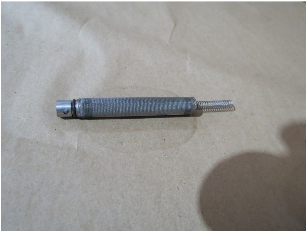
Photo 17: View of the servo fuel inlet screen.
