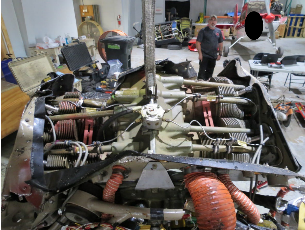
Photo 18: View of the fuel flow divider attached to the engine.
