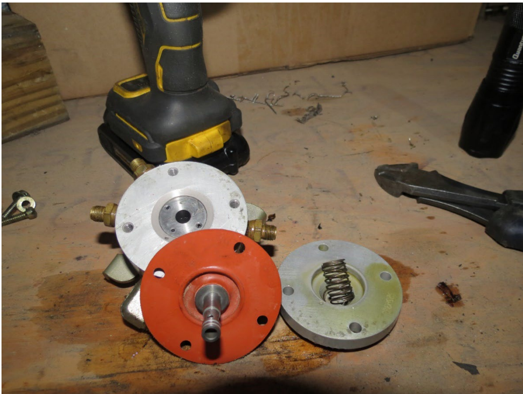
Photo 19: View of the fuel flow divider disassembled for examination.
