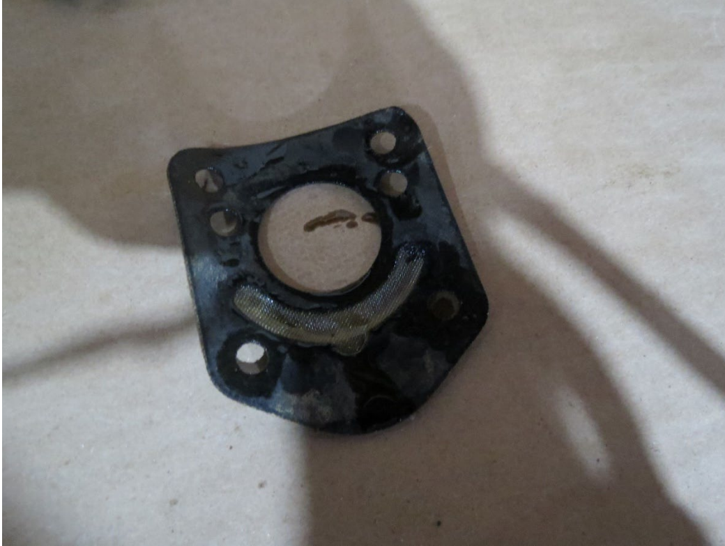
Photo 34: Propeller governor oil screen.
