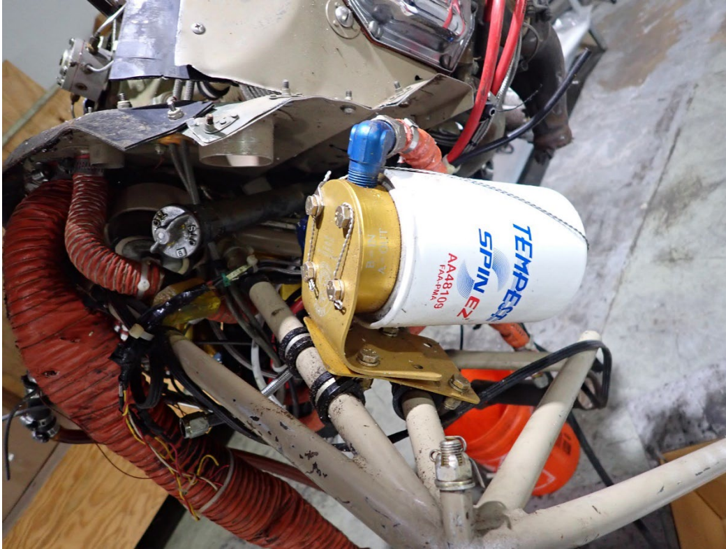
Photo 23: View of the oil filter attached to its mount.
