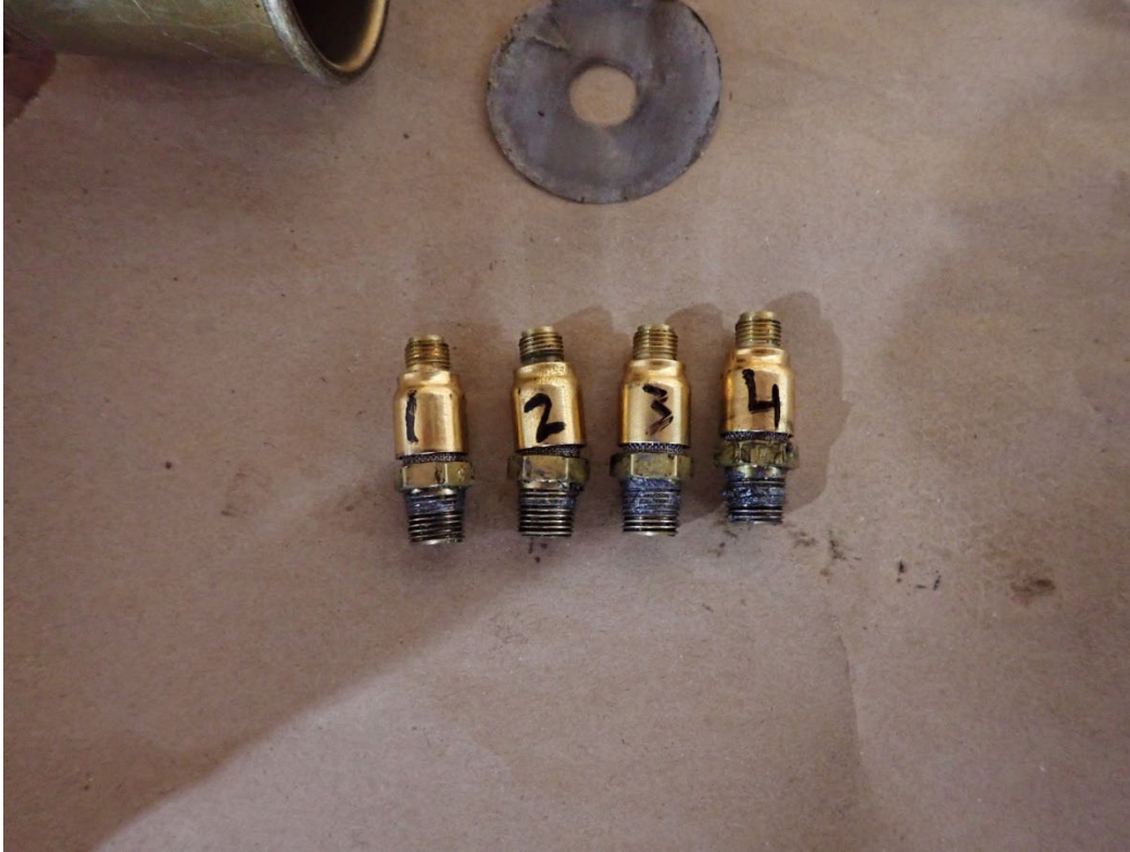
Photo 20: View of all four fuel injector nozzles.
