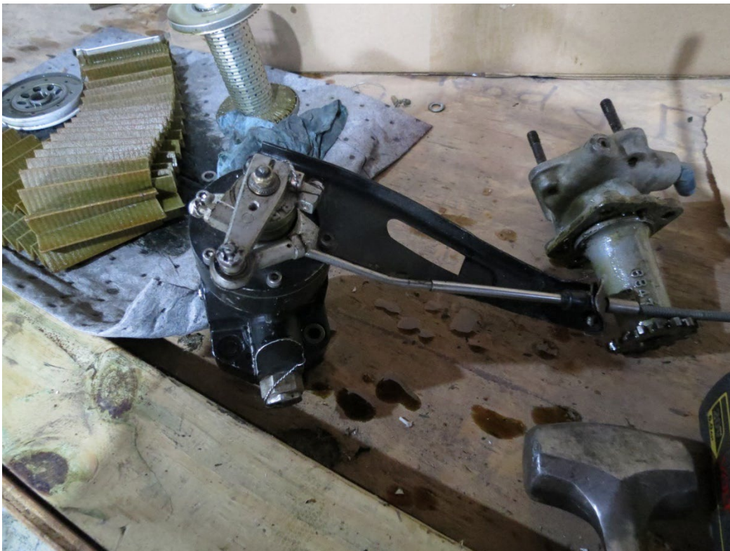
Photo 33: Overview of the propeller governor partially disassembled for examination.
