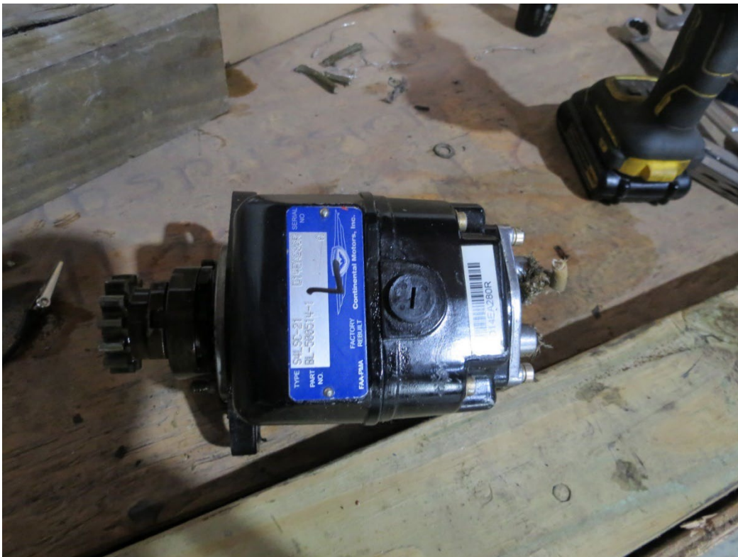
Photo 6: View of the left standard magneto removed for examination.
