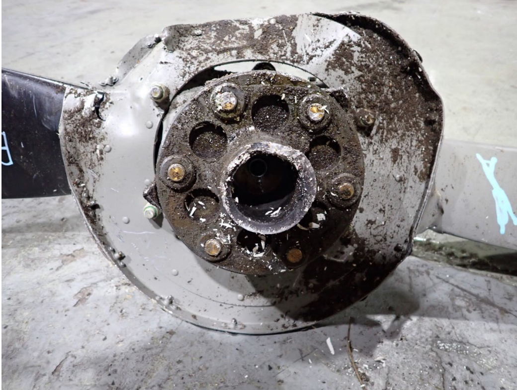
Photo 26: View of the crankshaft flange which remained attached to the propeller hub.
