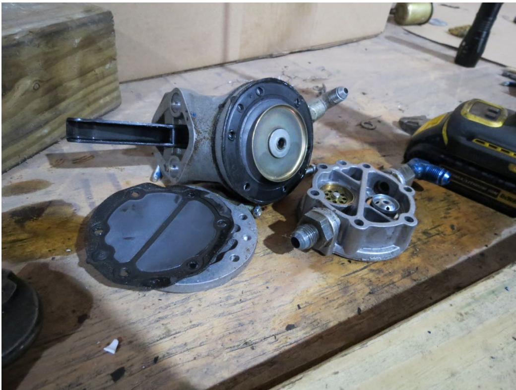
Photo 13: View of the engine driven fuel pump disassembled for examination.
