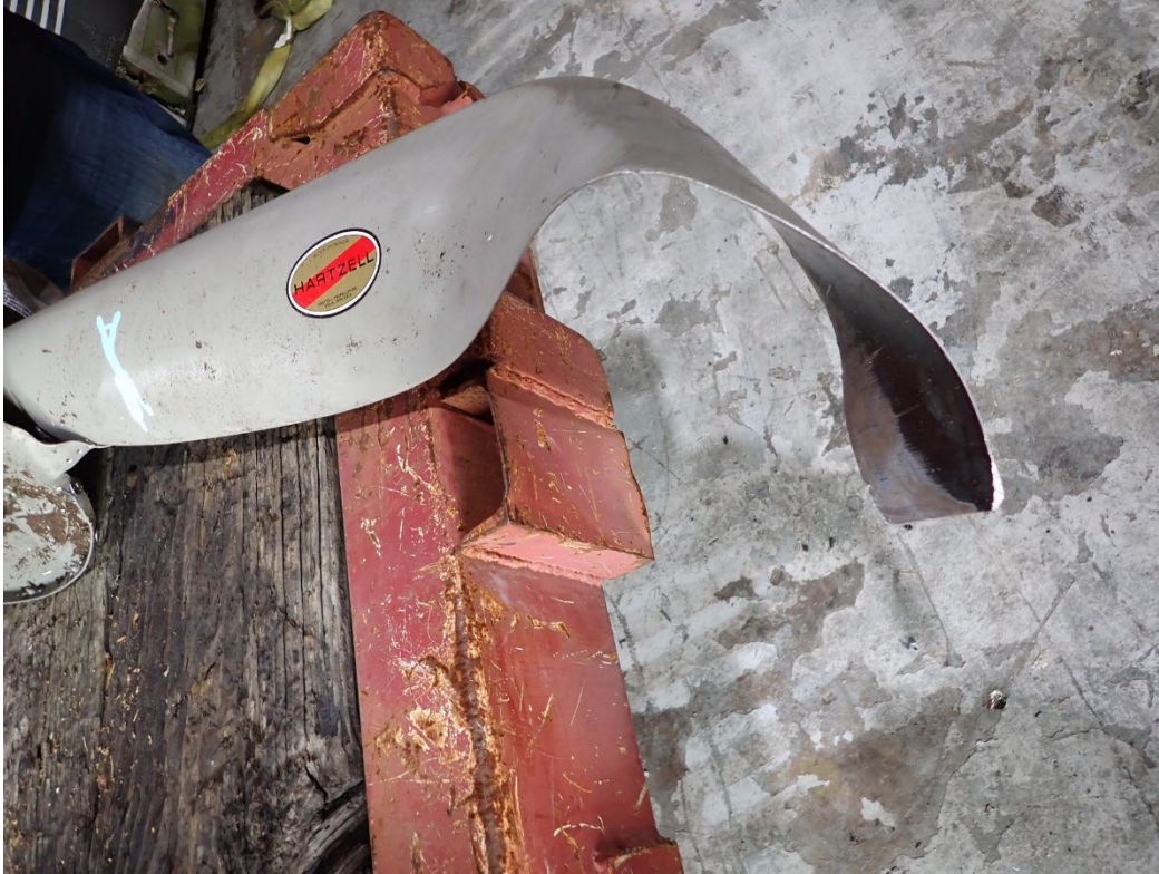
Photo 28: S-bending of propeller blade A.
