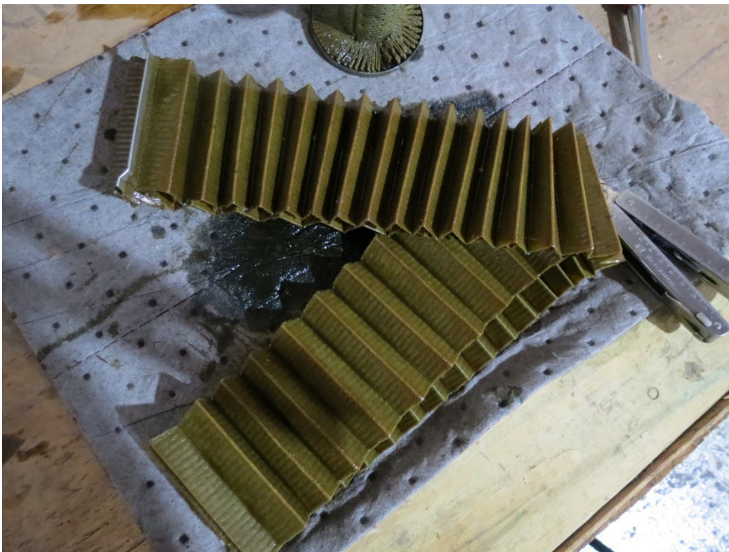
Photo 24: View of the oil filter pleats.
