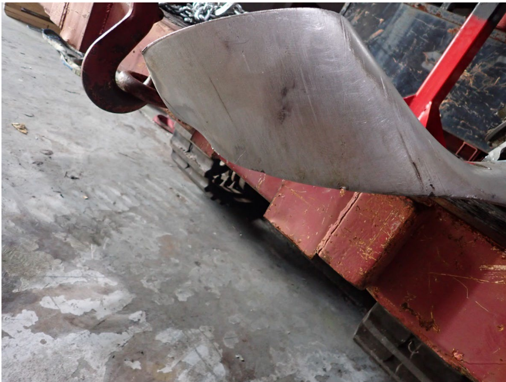
Photo 29: Polishing and leading-edge gouging of propeller blade A.
