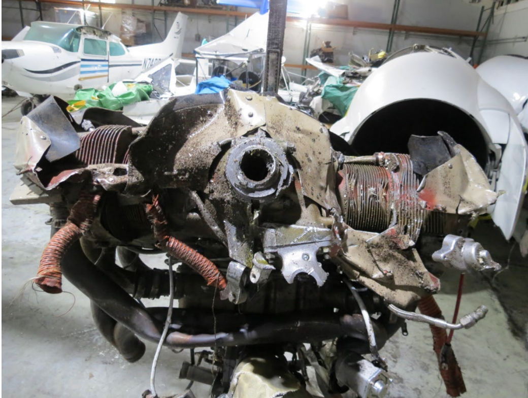
Photo 2: Impact separation of the crankshaft flange.
