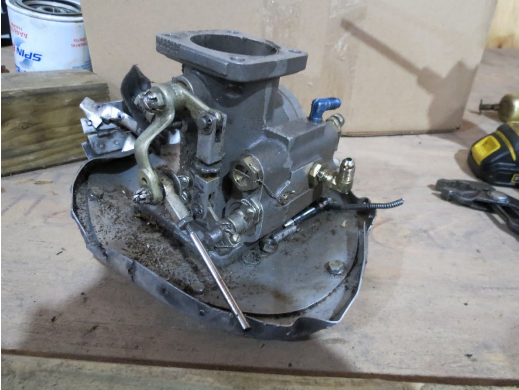
Photo 14: View of the fuel injector servo removed for examination.
