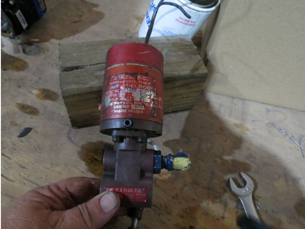
Photo 12: View of the fuel boost pump removed for examination.
