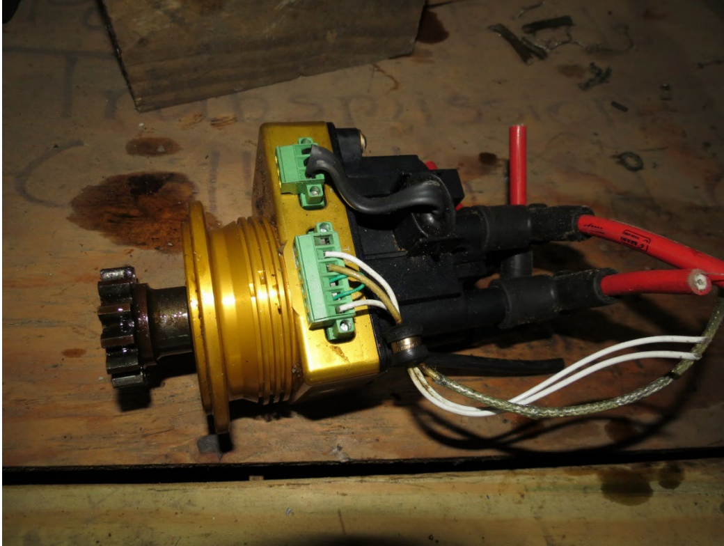
Photo 7: View of the electronic magneto removed for examination.
