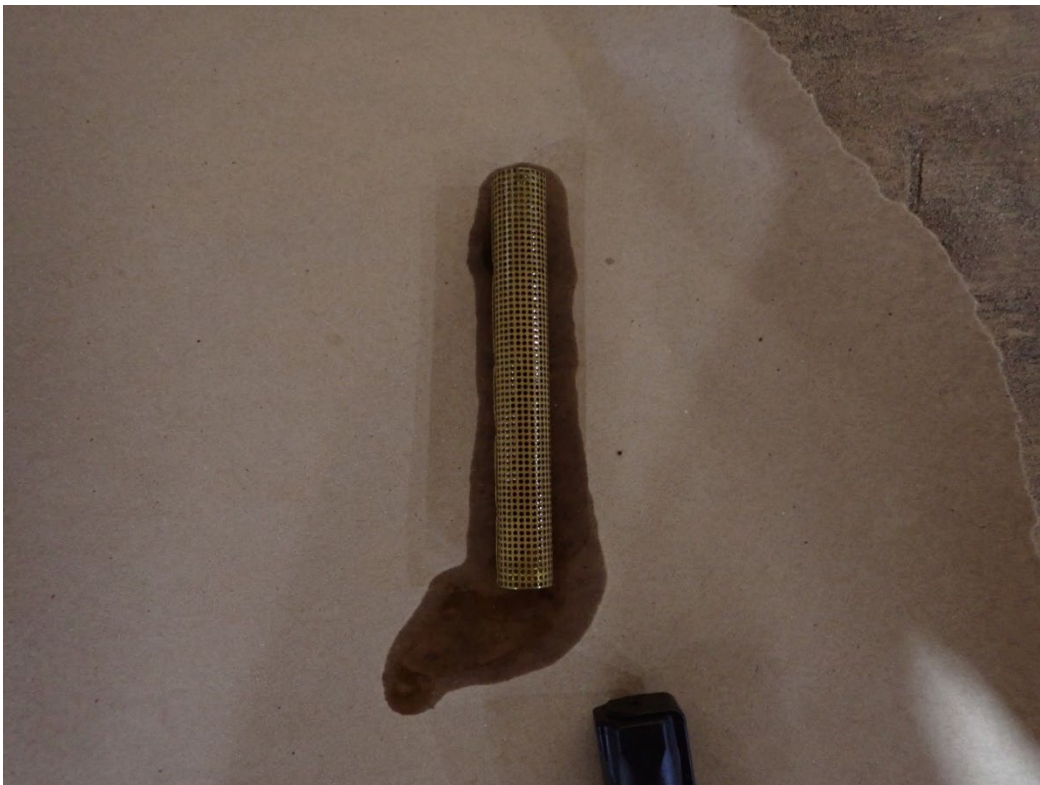
Photo 22: View of the oil suction screen removed for examination.
