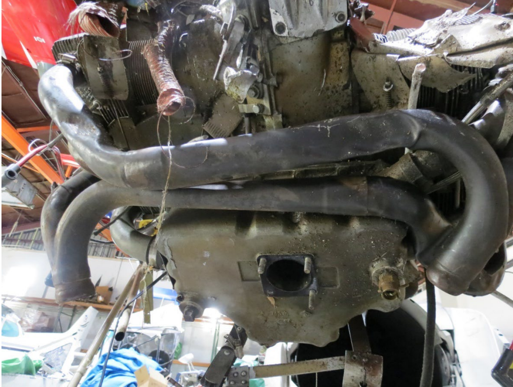
Photo 21: View of the oil pan from the bottom with the fuel injector servo removed.
