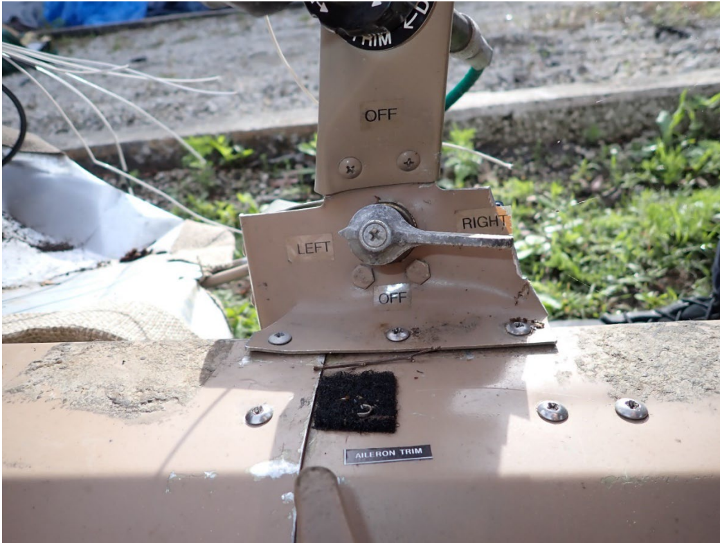
Photo 10: Fuel selector as first seen at the recovery facility.
