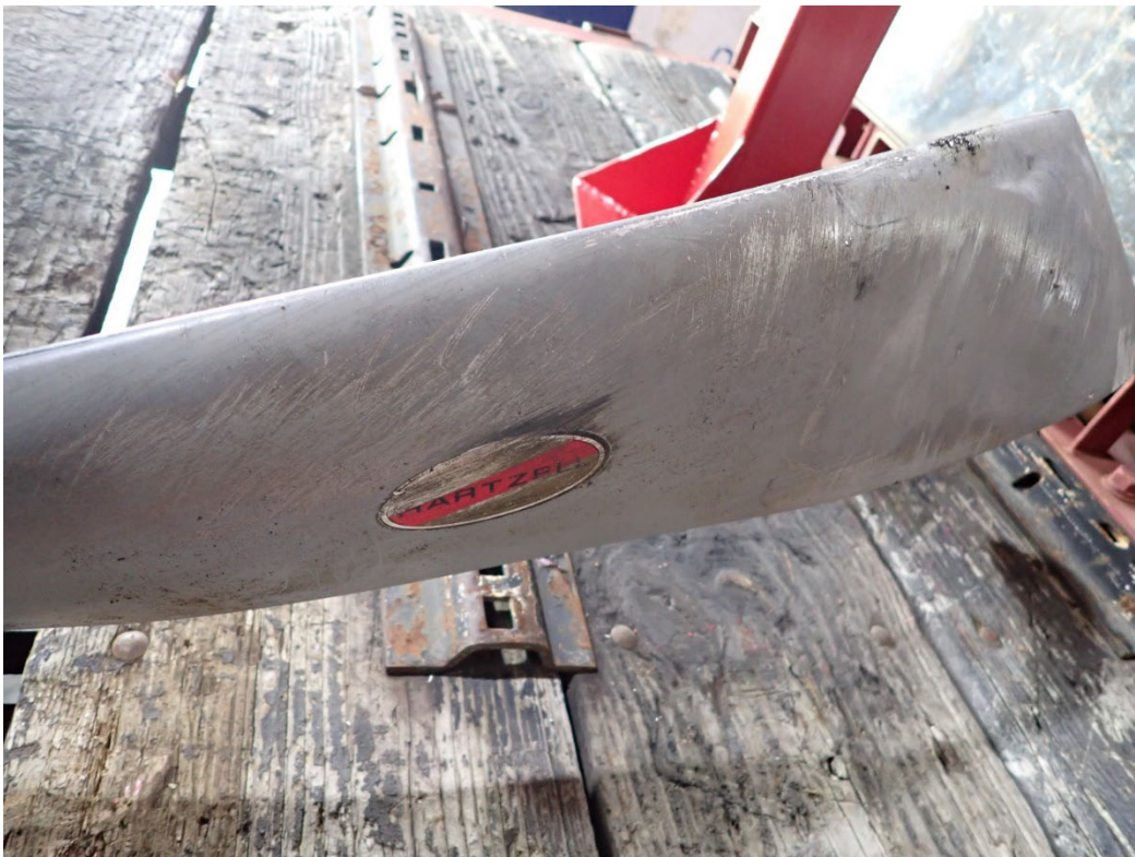
Photo 31: Chordwise scratching and polishing of propeller blade B.
