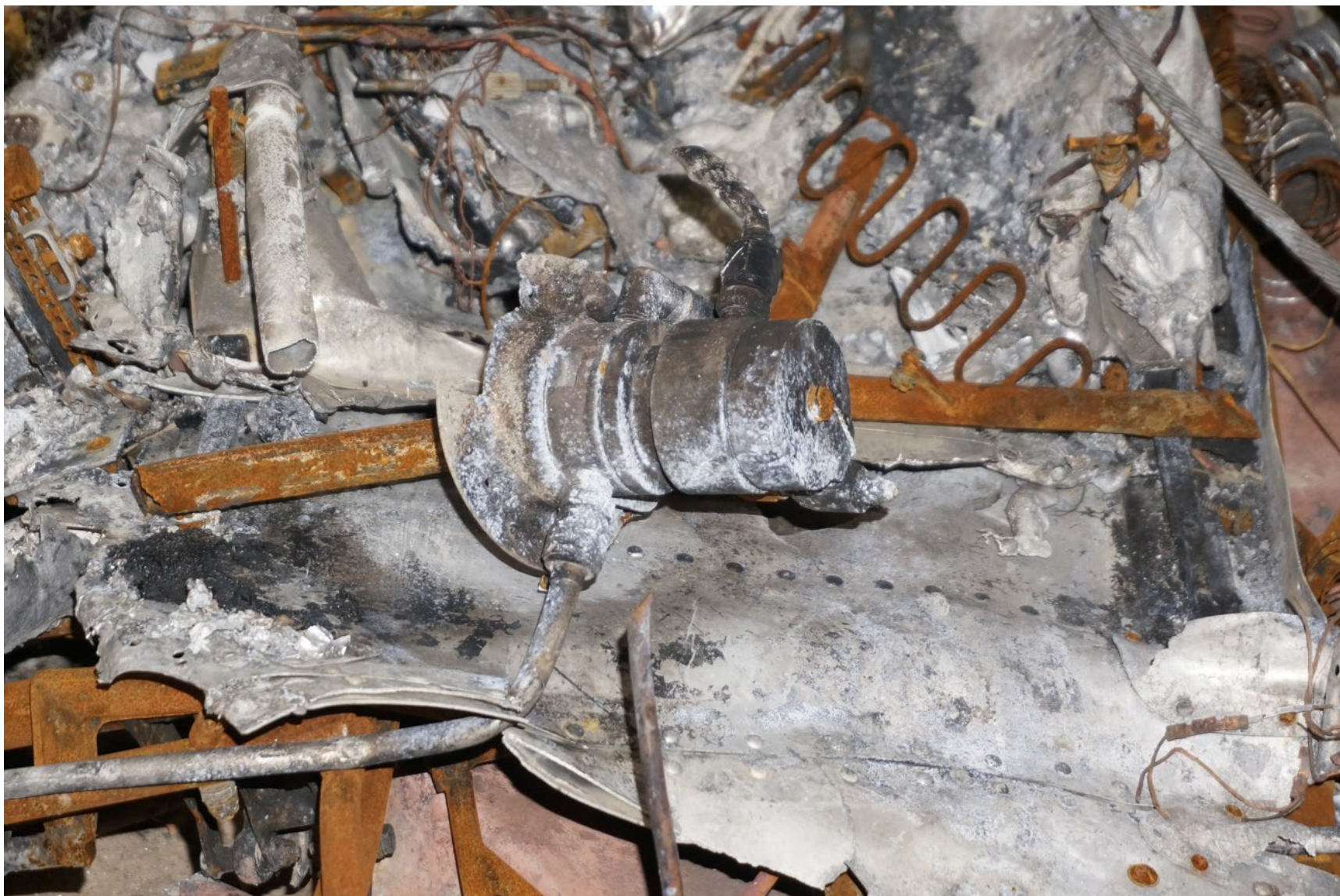
Photograph 8 - Fuel Selector Valve
