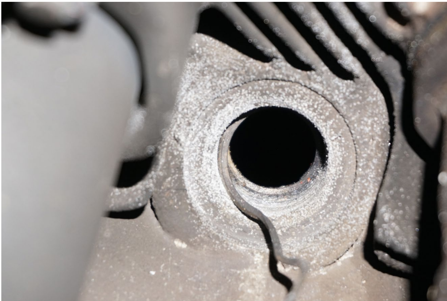
Photograph 12 - Close Up of No.3 Bottom Spark Plug Hole and Helicoil
