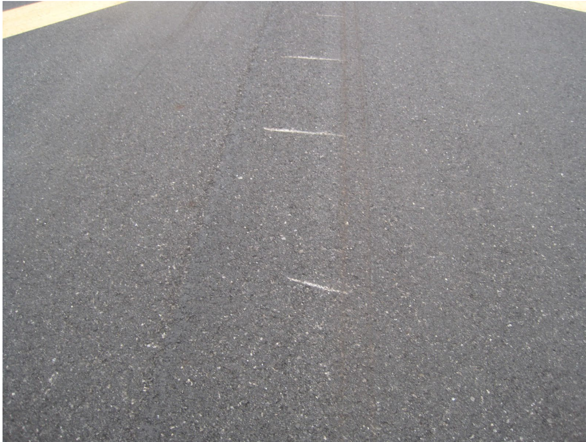
Photograph 2 - Close Up of Propeller Strike Marks (Courtesy of FAA)
