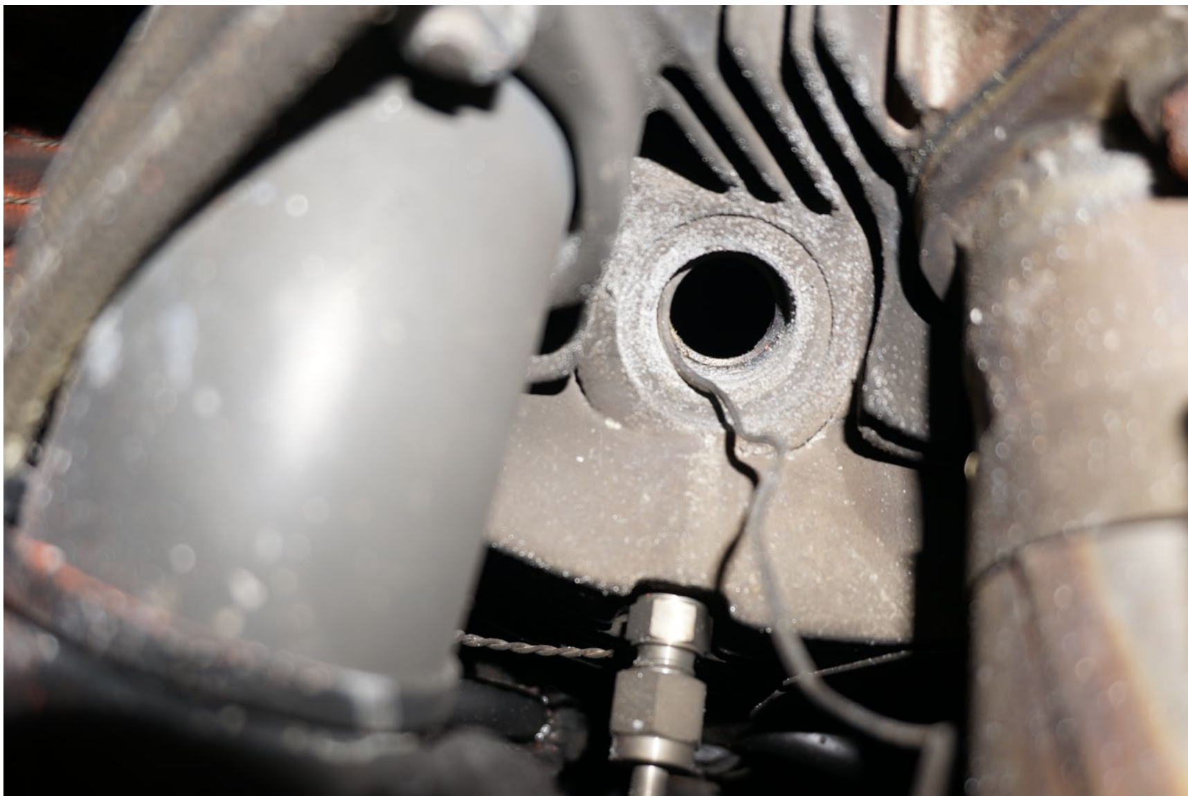
Photograph 11 - No.3 Bottom Spark Plug Hole and Helicoil
