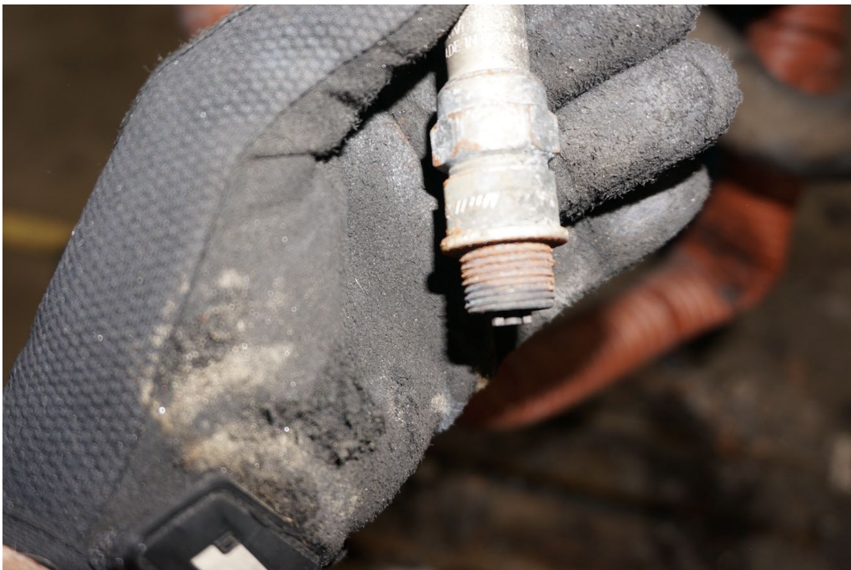
Photograph 10 - Close Up of No.3 Bottom Spark Plug
