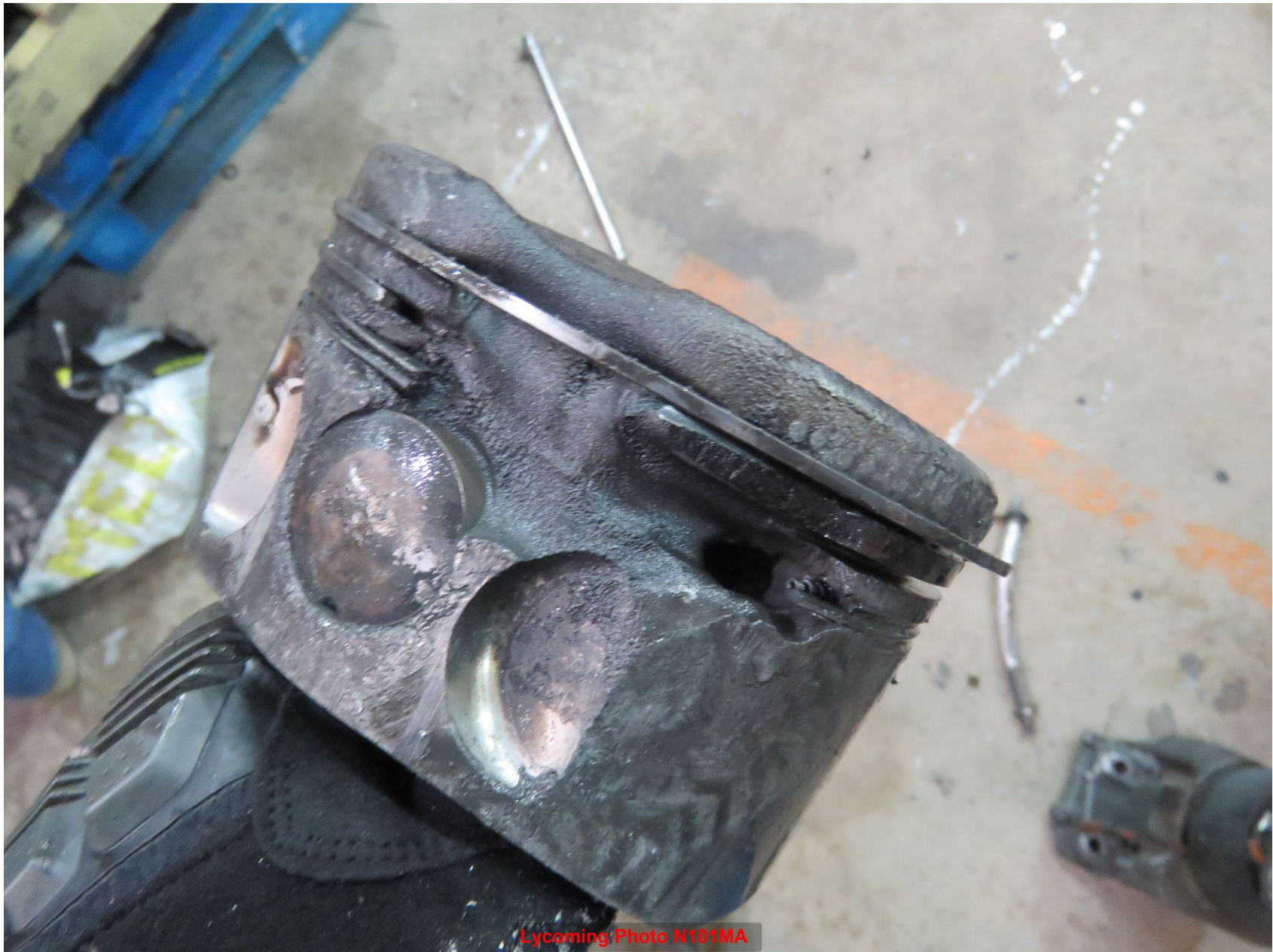
Photo 6 – View of #5 Piston Displaying Damage Signatures Consistent with Detonation (Lycoming)
