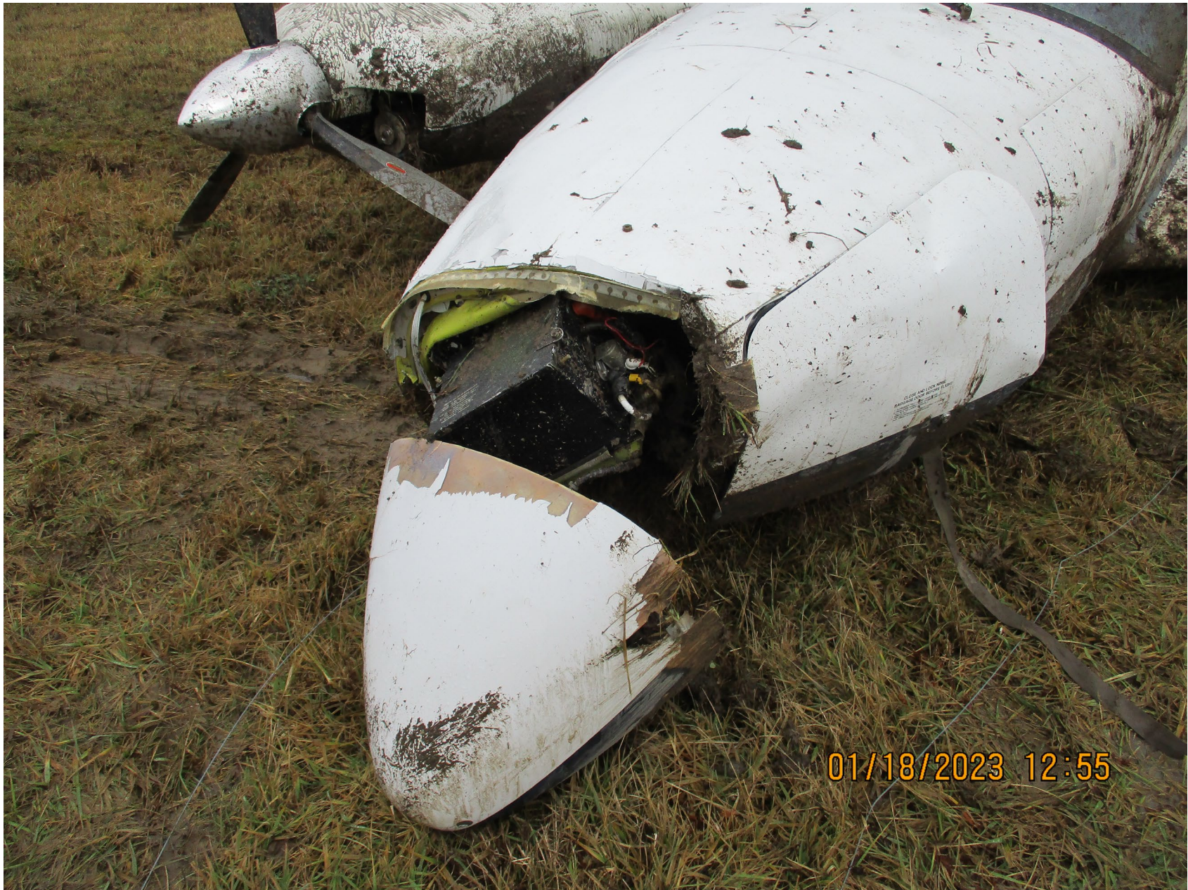
Photo 3 – View of Damage to Nose Compartment (FAA)
