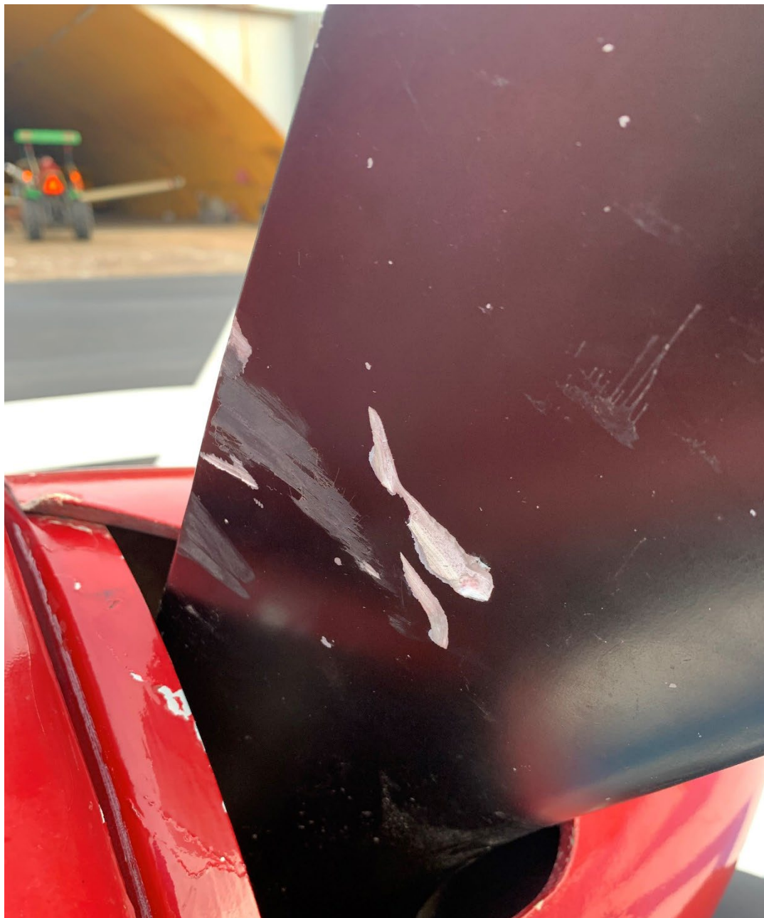
Photo 2 – Closeup of Damage to Rear Side of Propellor Blade (Courtesy of Operator)
