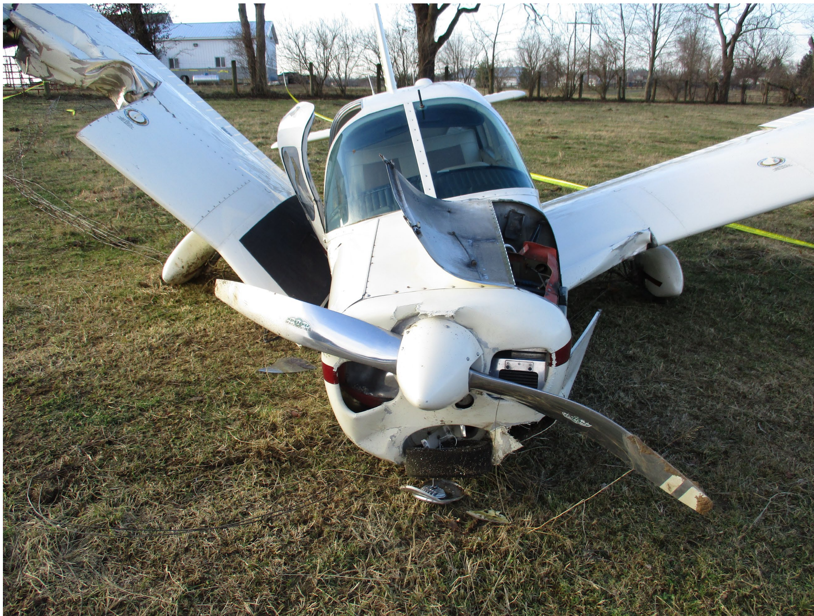
Photo 1 – View of airplane from the front showing damage to engine cowling (FAA Photo)
