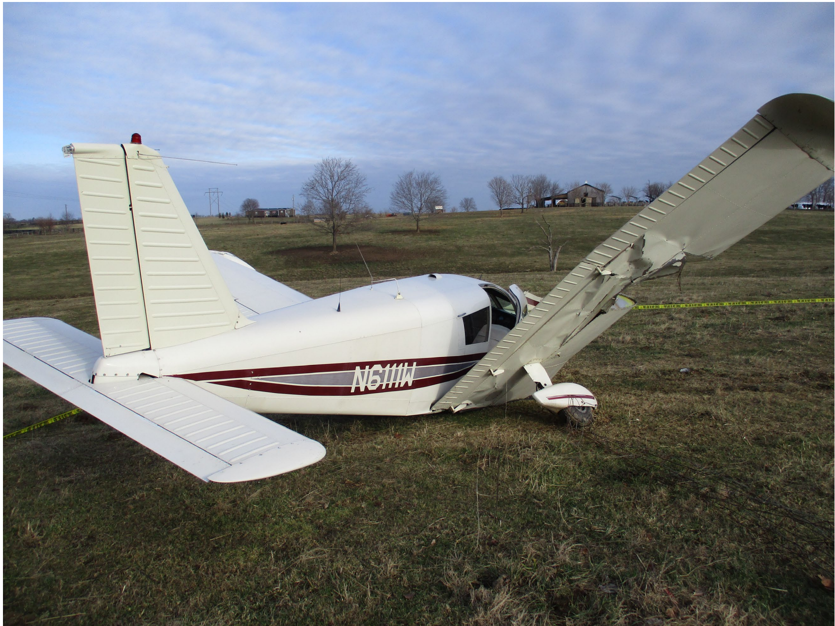
Photo 2 – View of airplane from right side showing damage to right wing (FAA Photo)
