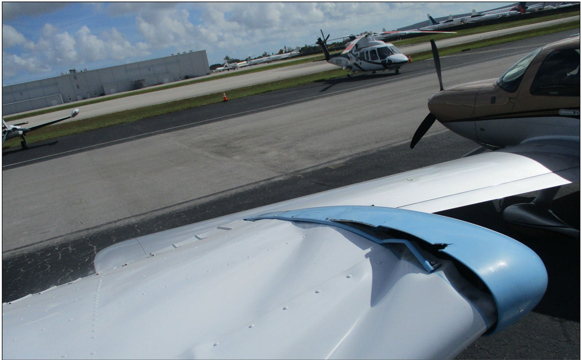
Photo 1: Overview of the left wing and substantial damage (Photo Courtesy of FAA)
