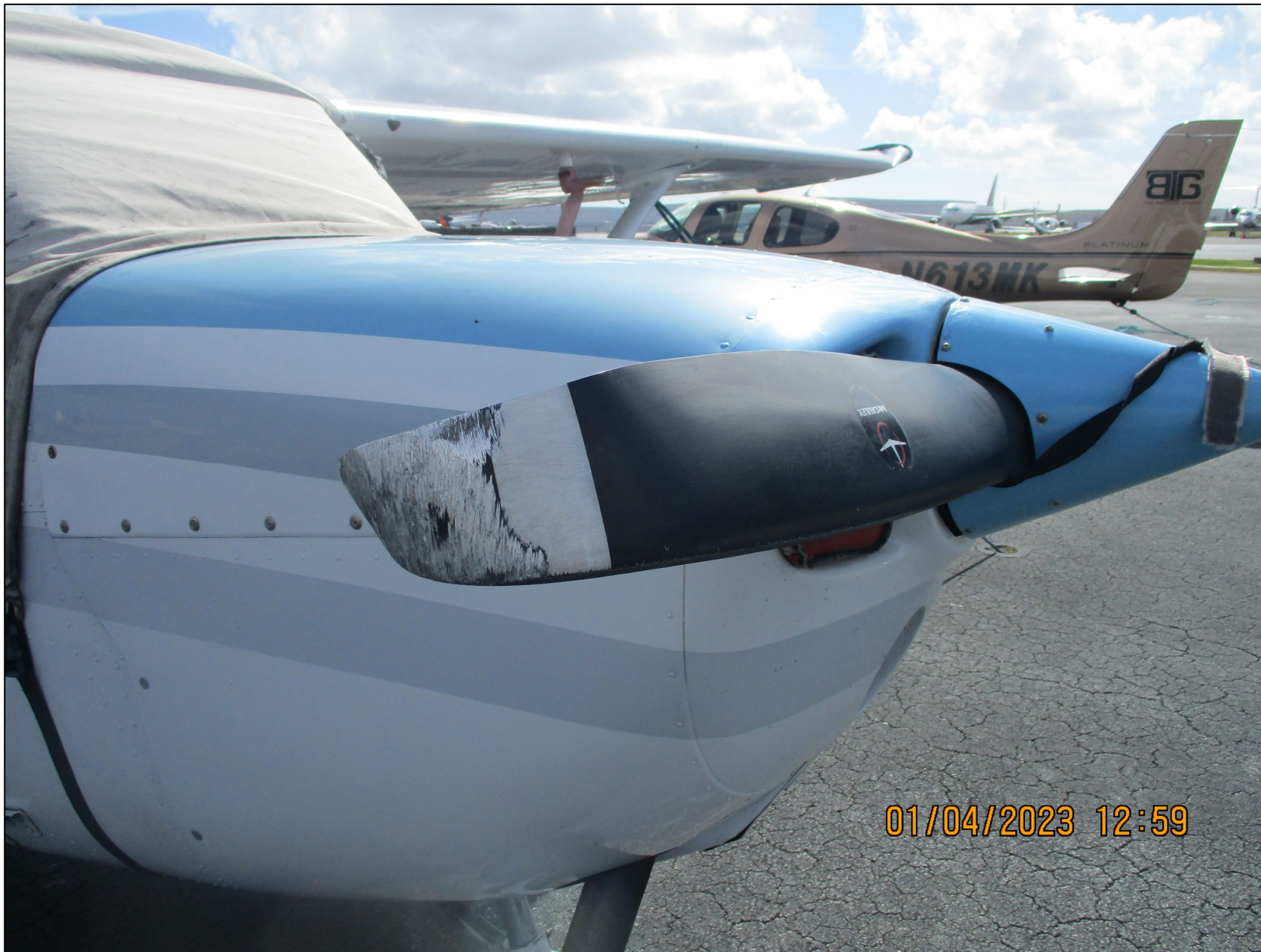
Photo 3: View of the propeller damage (Photo Courtesy of FAA)
