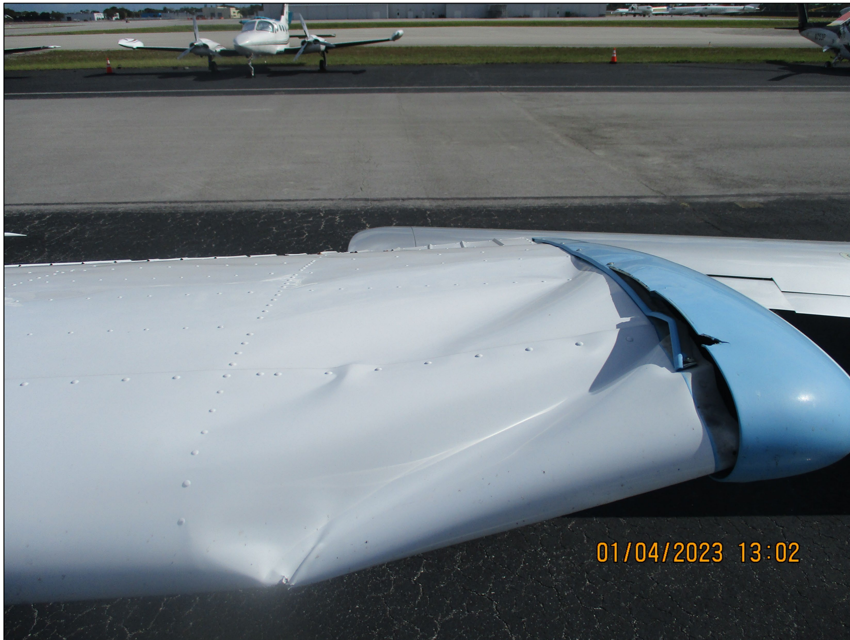
Photo 2: Additional view of the substantial damage sustained to the left wing (Photo Courtesy of FAA)
