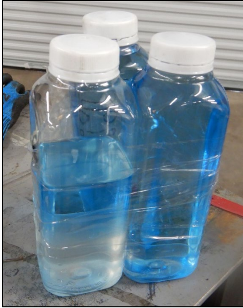
Photo 10 - View of recovered fuel with water present
