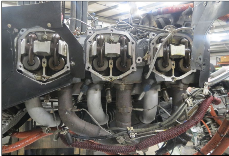
Photo 17 - Cylinder Nos 2, 4, and 6 with rocker covers removed
