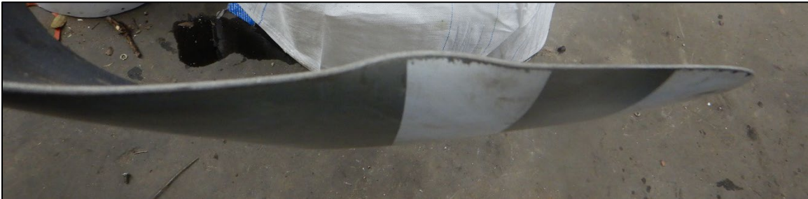
Photo 23- View of deformation of the outermost portion of propeller blade "B"
