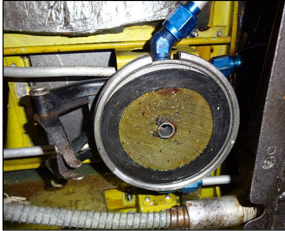
Photo 7 - View of gascolator filter with debris
