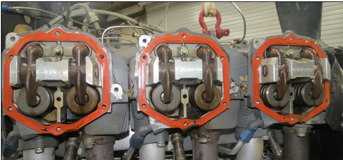
Photo 18 - Cylinder Nos 1, 3, and 5 with rocker covers removed
