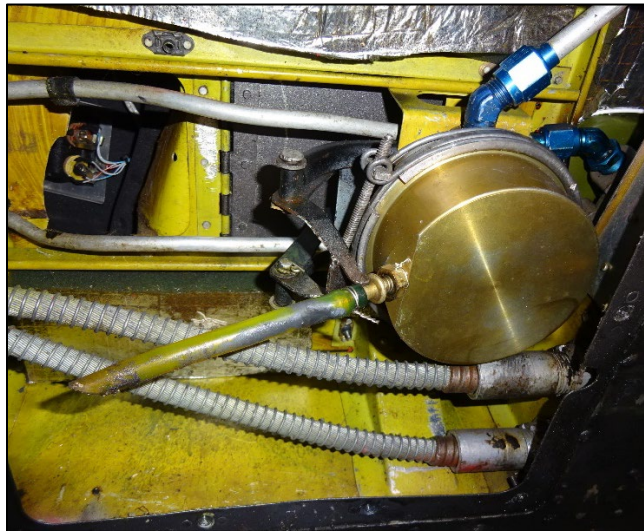
Photo 6 - View of gascolator in airplane belly below flight selector
