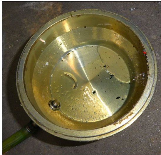
Photo 8 - View of gascolator bowl before testing
