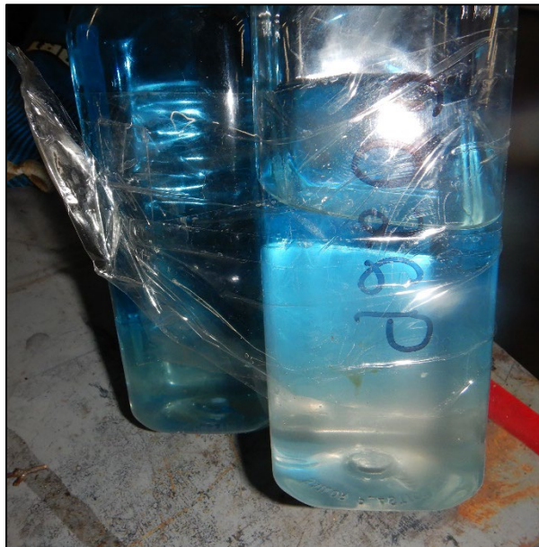
Photo 11 - Close-up view of water in fuel
