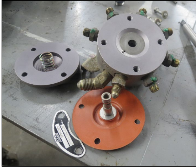
Photo 19 - Fuel flow divider after examination
