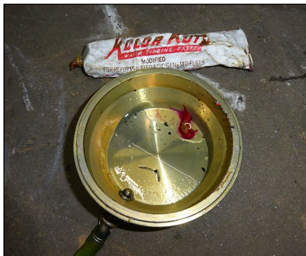
Photo 9 - View of gascolator bowl with red water-finding paste
