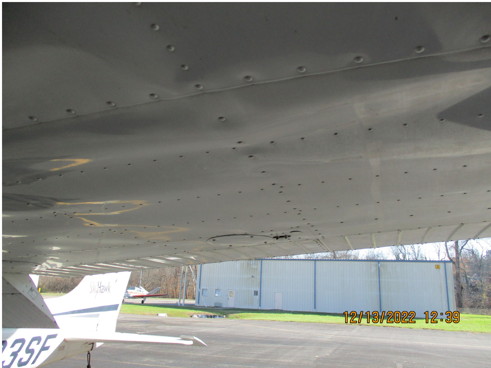
Photo 5 – Wrinkling of skin aft of the forward spar (FAA Photo)
