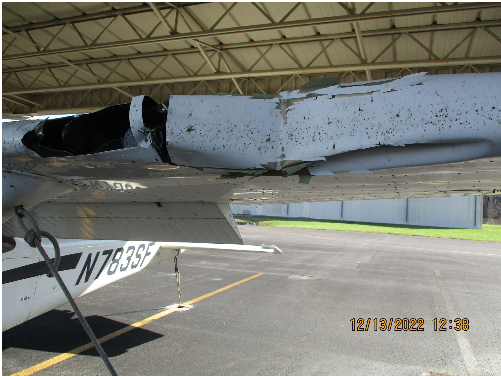
Photo 2 – Left wing damage (FAA Photo)
