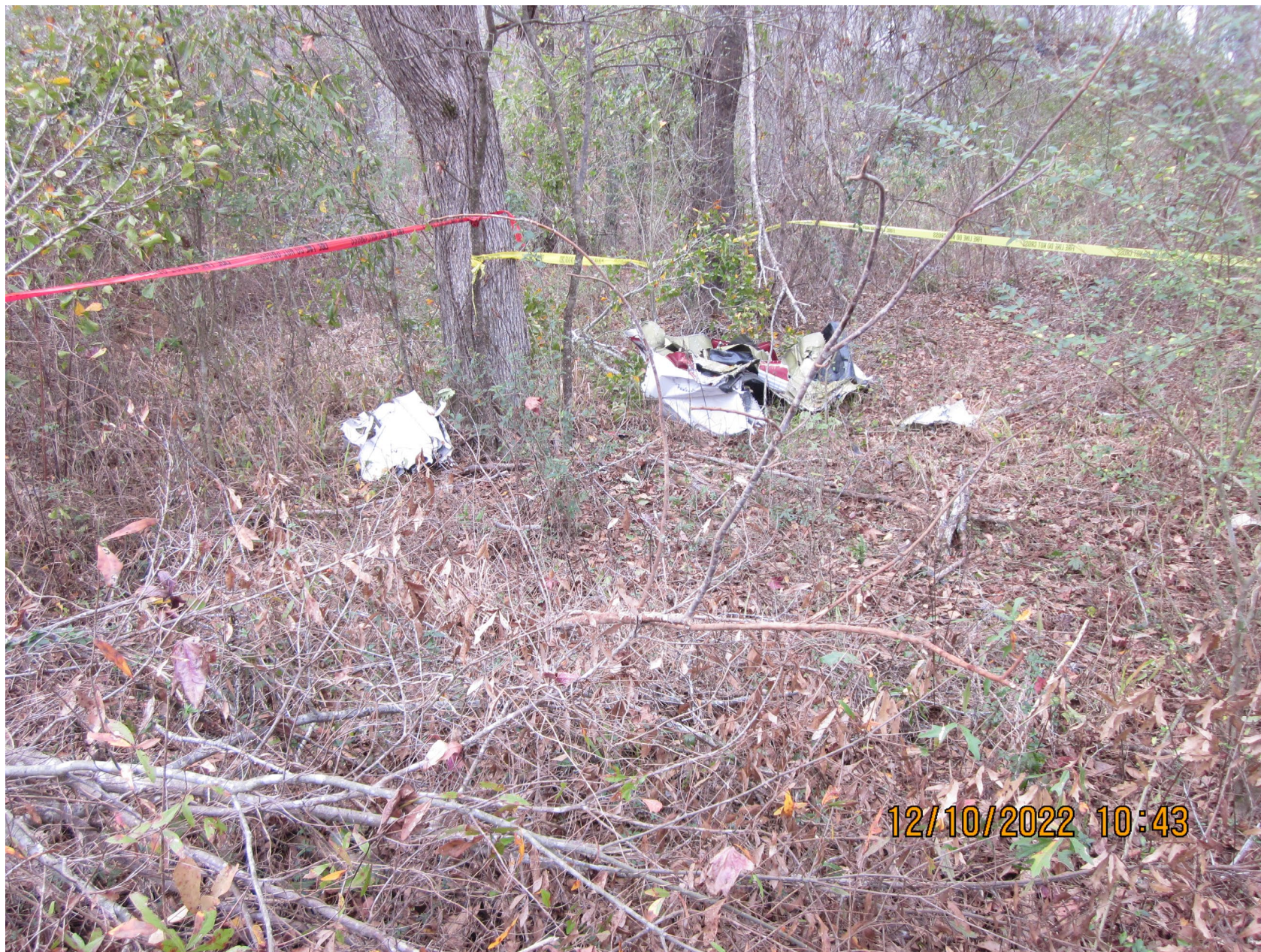
Photo 4 – Impact separated wreckage of right wing (FAA Photo)
