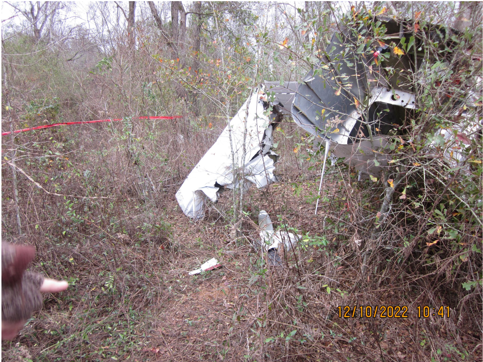
Photo 2 – Damage to the right wing (FAA Photo)
