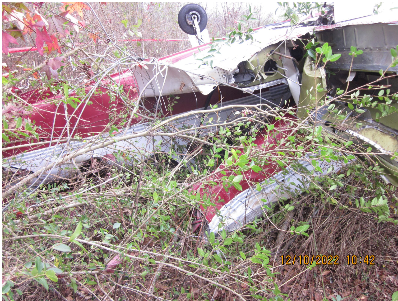
Photo 3 – Damage to right wing (FAA Photo)
