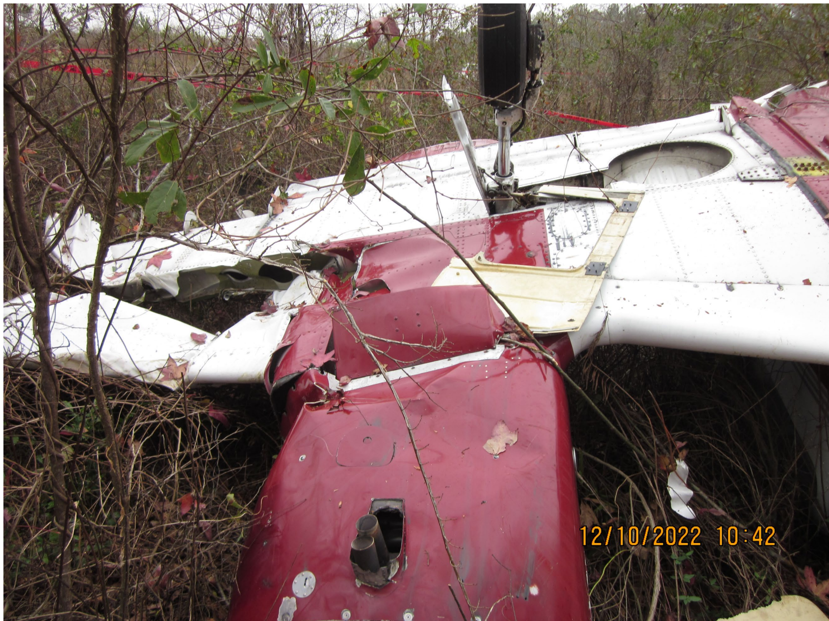
Photo 5 – Damage to left wing (FAA Photo)
