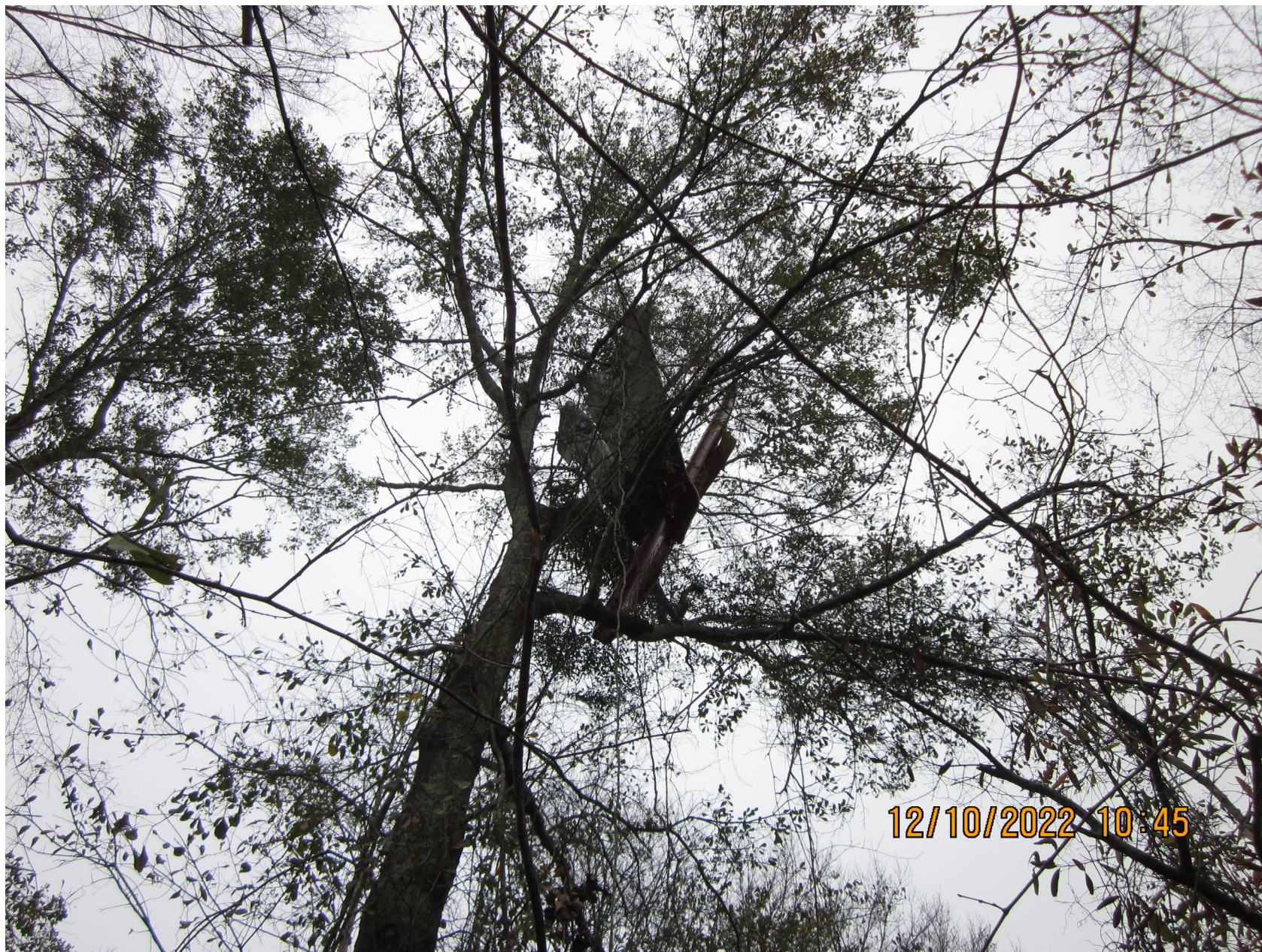
Photo 6 – Impact separated tail section, found in a tree about 40 yards from main wreckage (FAA Photo)
