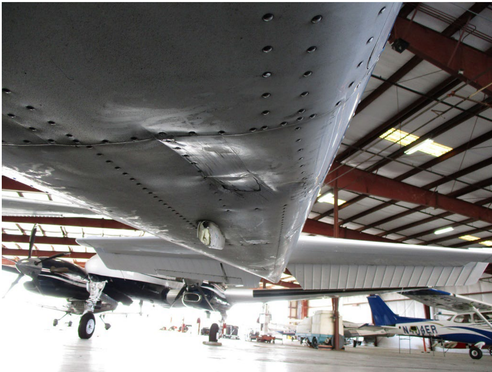
Photo 2 – Empennage Damage (Photo Courtesy of FAA)
