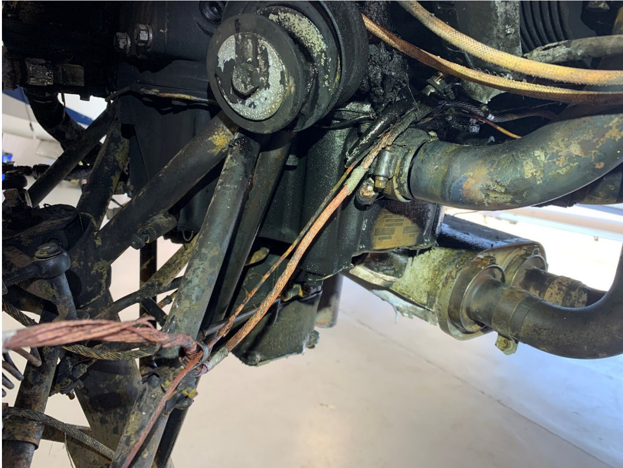
Photograph 2 - View of engine compartment alternator wire. (Courtesy of FAA)
