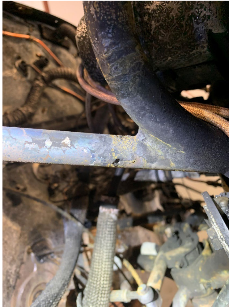
Photograph 4 - View of engine mount electrical arc damage. (Courtesy of FAA)
