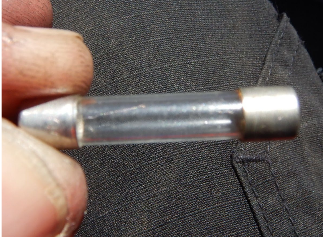
Photo 1 - Open 2-amp Fuse (Courtesy Textron Aviation)
