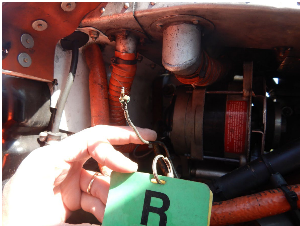
Photo 2 - Separated Alternator Field Wire (Courtesy Textron Aviation)
