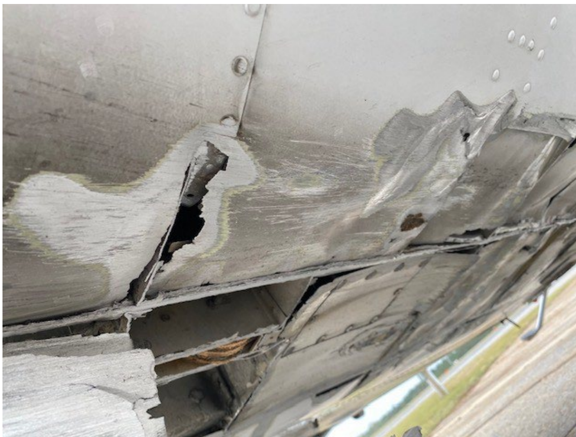
Photograph 2 - Lower Fuselage Skin and Structure Damage (Courtesy of FAA)
