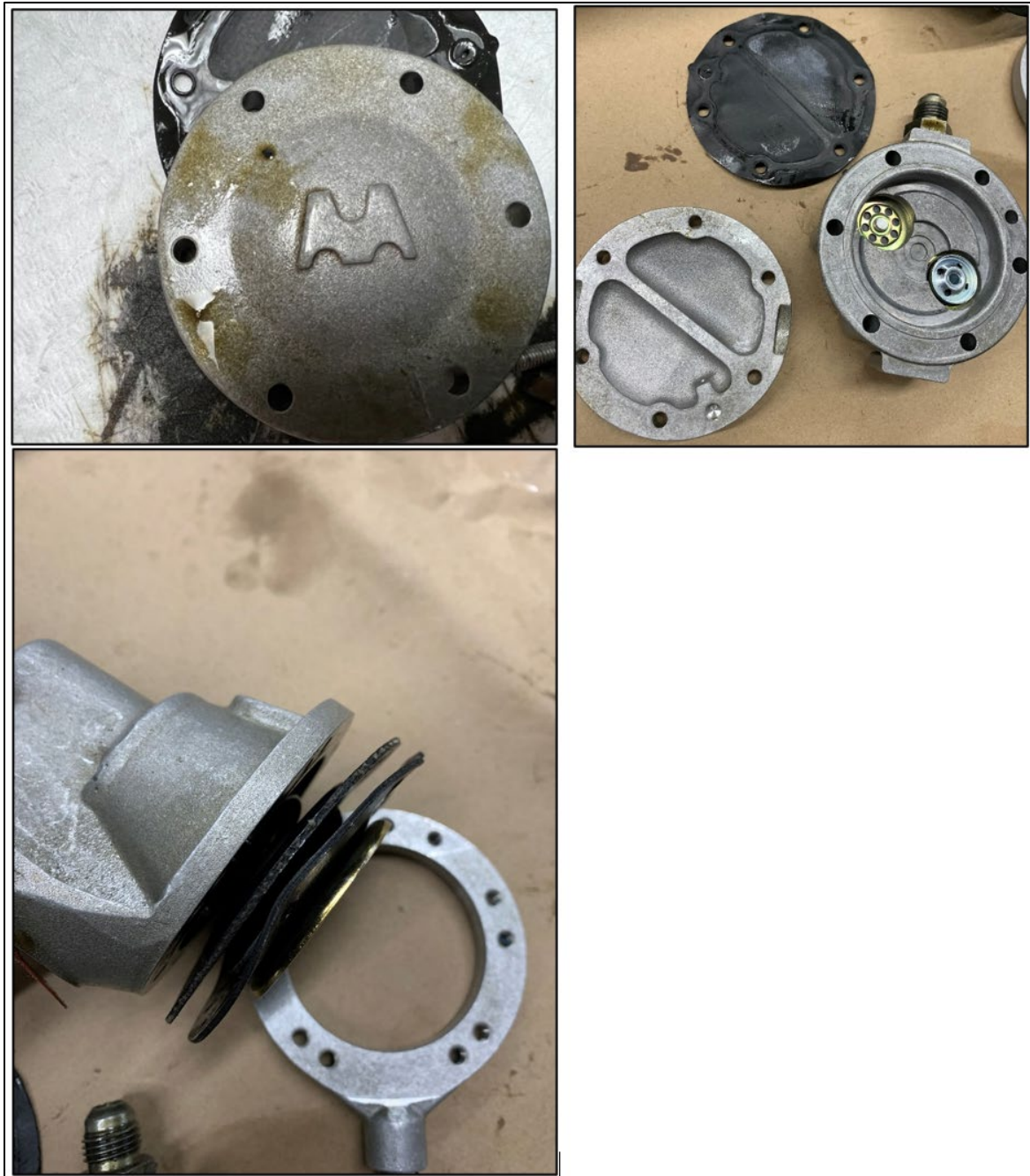
Figure 1: View of the engine driven fuel pump disassembled postaccident.
