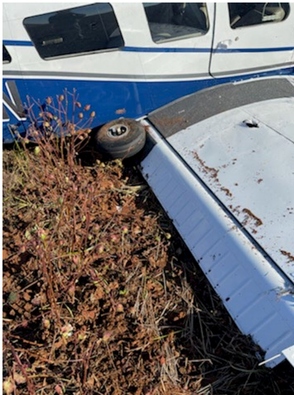
Photo 2 – Right Wing Damage (Photo Courtesy of FAA)
