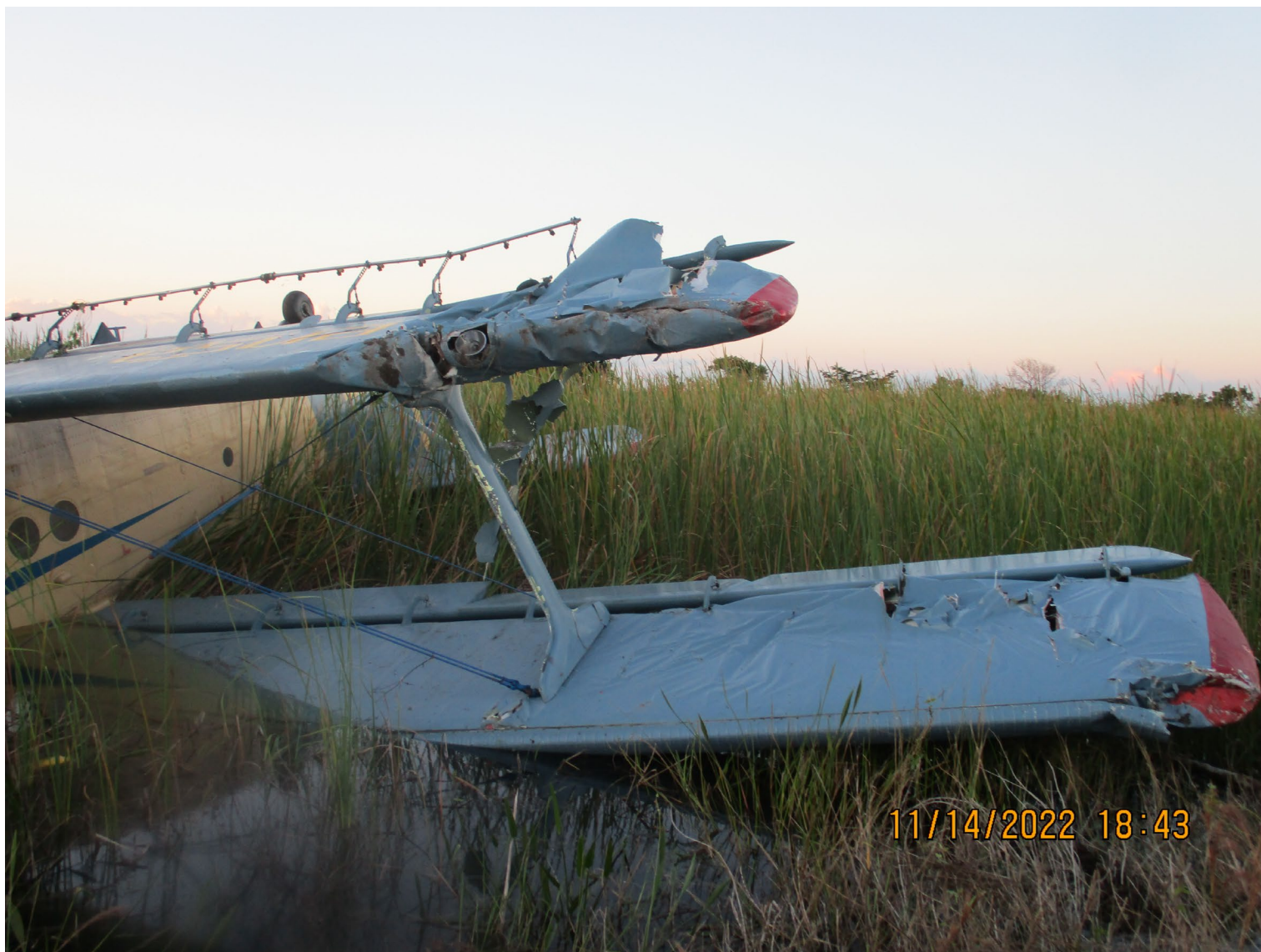
Photograph 3 - Close Up of Outboard Sections of Lower and Upper Outboard Right Wing Sections (Courtesy of FAA)
