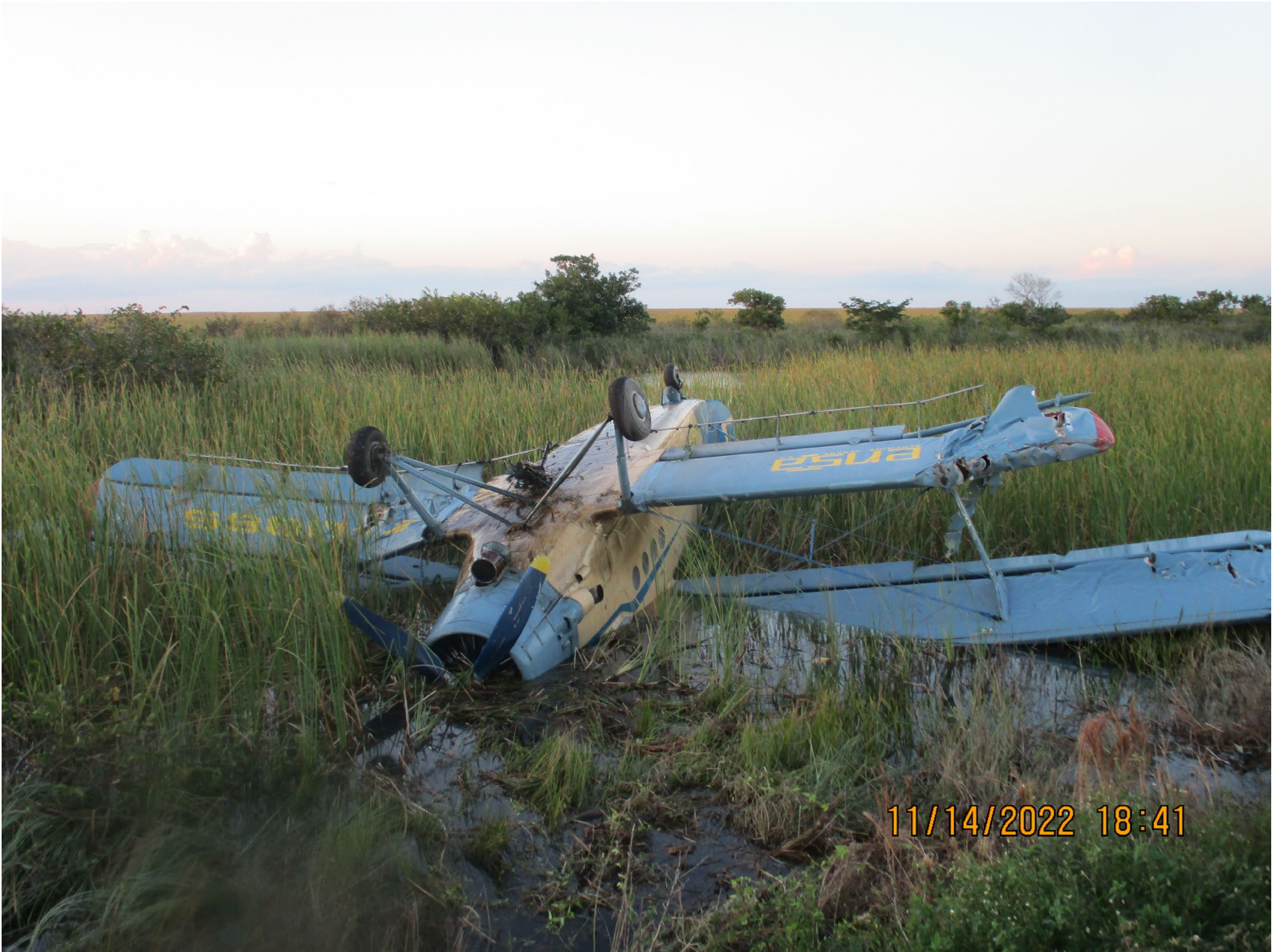
Photograph 1 - Main Wreckage (Courtesy of FAA)
