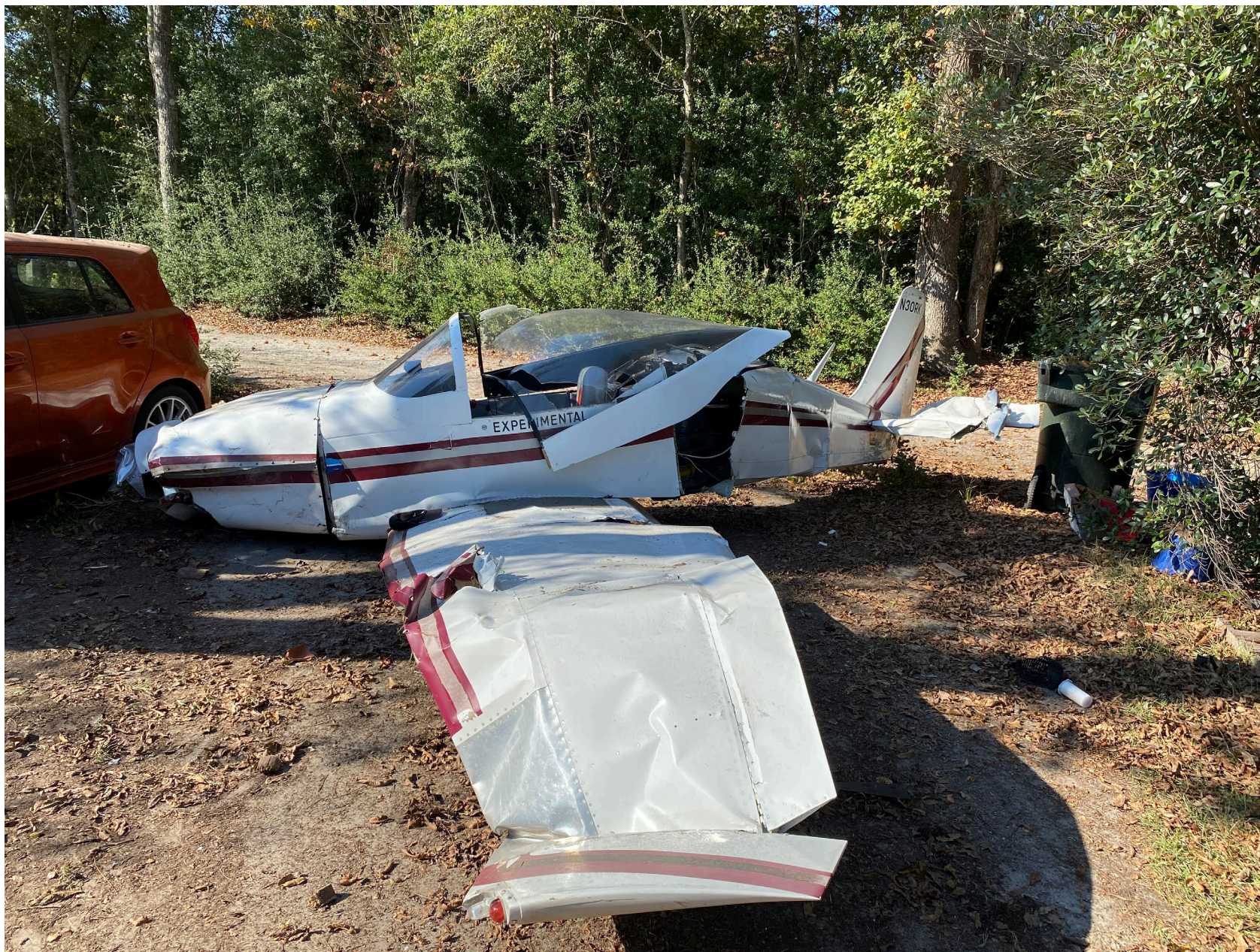
Photo 2 - FAA Digital Photograph. Left Side View of the Wreckage at the Accident Site. Note the Substantial Damage to the Left Wing.
