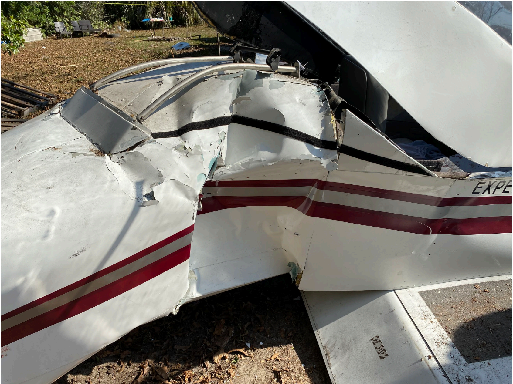
Photo 3 – FAA Digital Photograph. Right Side View of the Fuselage Aft of the Wing Center Section. Note the Substantial Damage.
