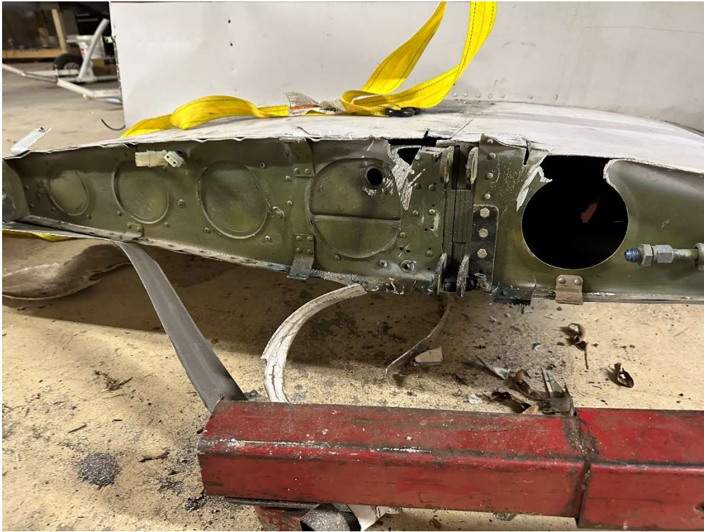
Figure 2: Digital Photograph from Jeremy Hill. View of Right Side of the Wing Center Section. Note the absence of any fuel tank between the main and aft spars.
