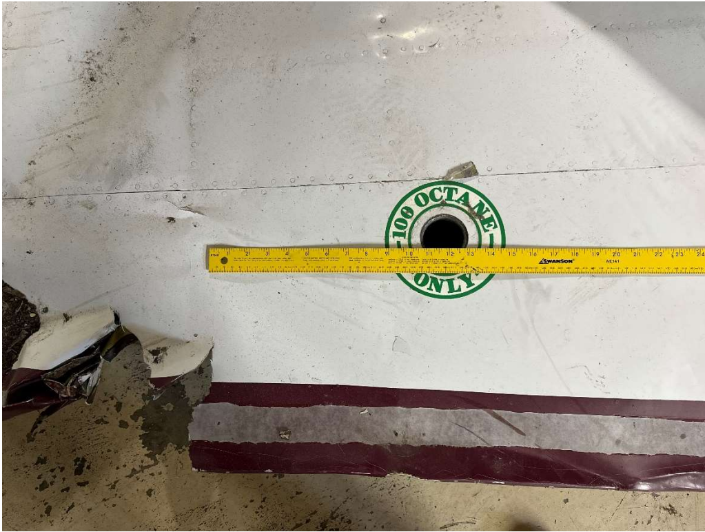
Figure 1: Digital Photograph from Jeremy Hill. Frontal View of a Portion of the Leading Edge of the Right Wing. Note the measurement from the fuel Filler Opening to the Outer Most Rib of the Wing Fuel Tank.
